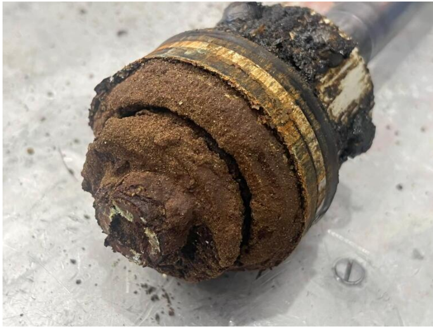
Figure 1 - Main Landing Gear Actuator Corrosion
