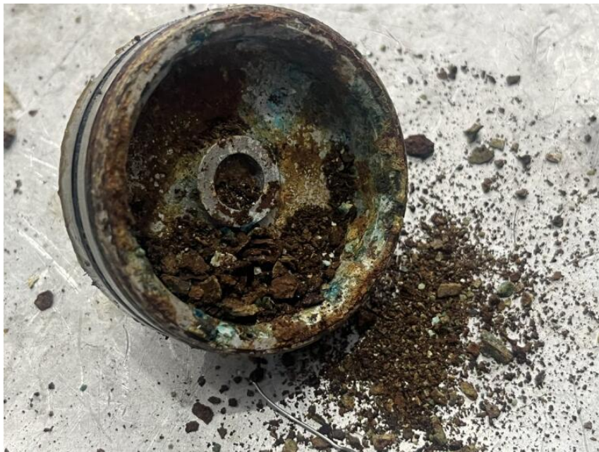
Figure 2 - Main Landing Gear Actuator Corrosion
