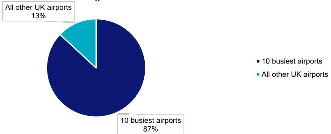
**Figure 27: Proportion of NO<sub>x</sub> emissions by aircraft during LTO cycle between 10 busiest and all other UK airports (2023)**
