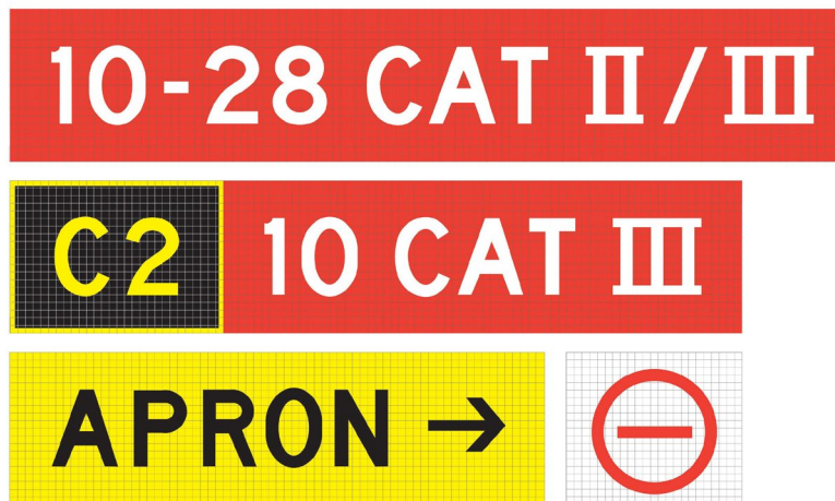
Figure 7A.8 Sign face size proportions and layout
