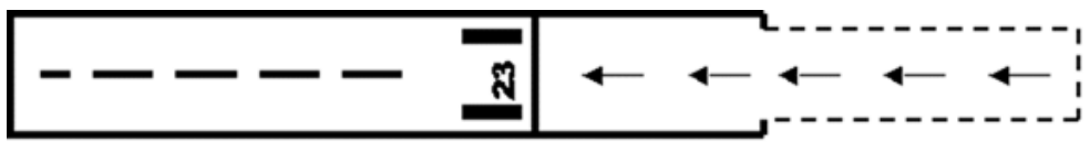
Figure 3H.1 Starter extension and pre threshold markings
