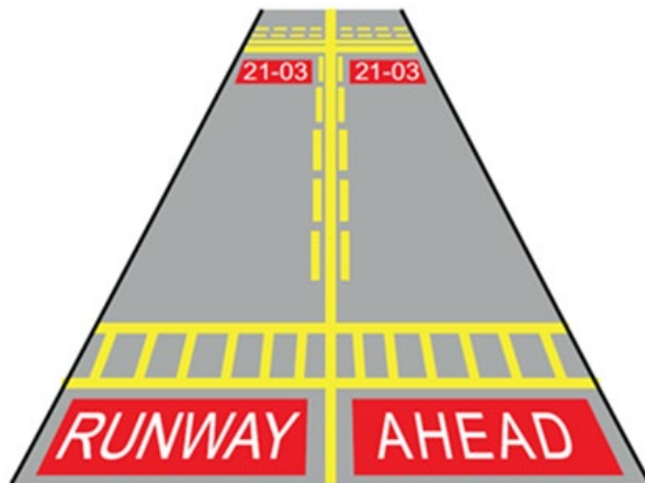
Figure 2D.2 Runway ahead marking – for pattern B (Cat II/III) holding position
