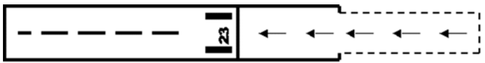
Figure 3H.1 Starter extension and pre threshold markings
