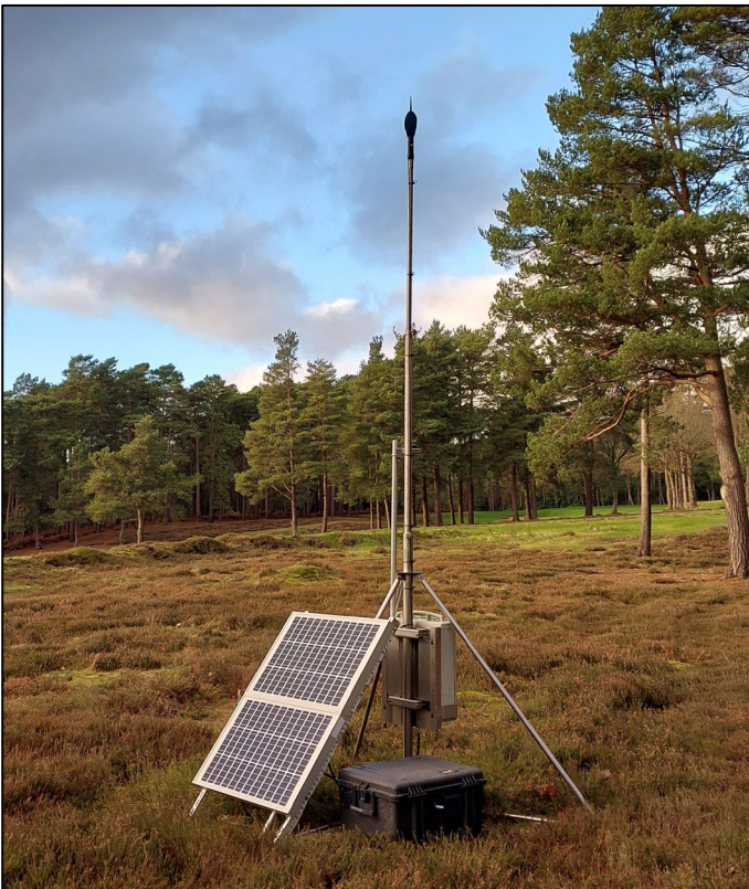
Figure 2 NTK mobile noise monitor
