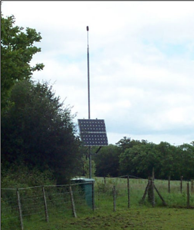
Figure 1 NTK fixed noise monitor
