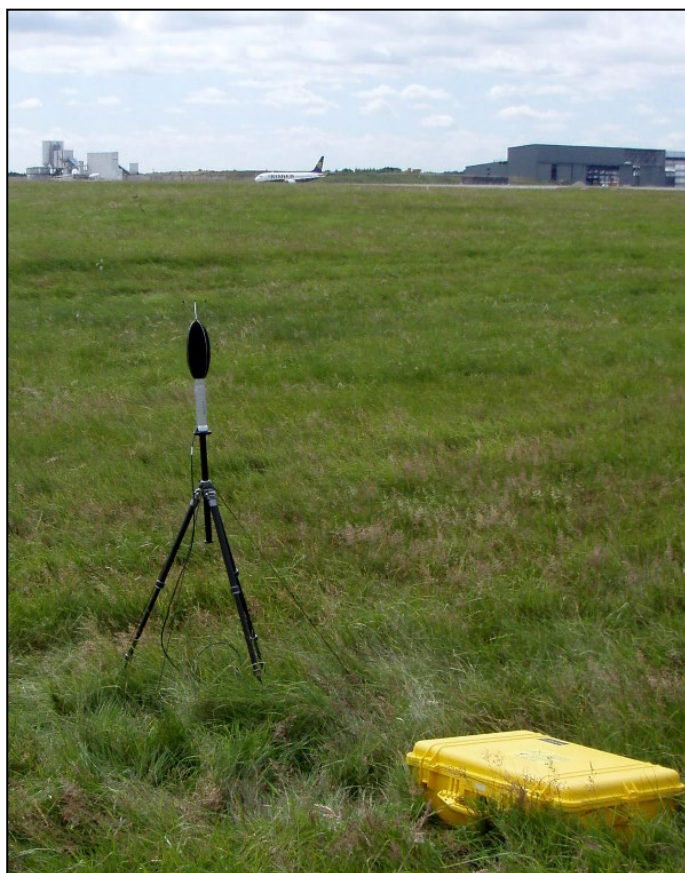
Figure 3 ERCD all-weather noise monitoring system
