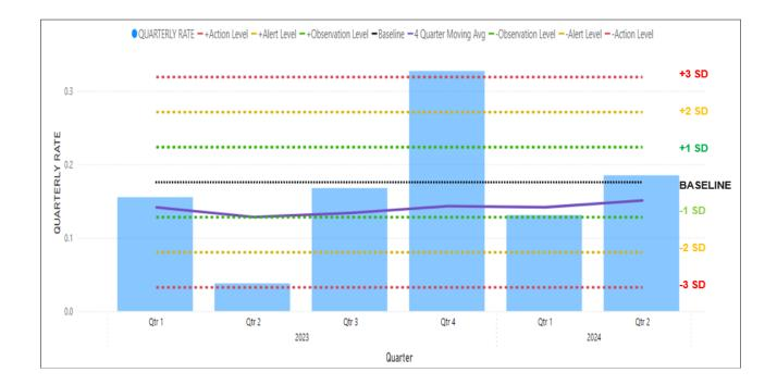
The graph shows the rates and alert levels for all of the data associated with it for fixed wing and rotary wing. The standard deviations are calculated around the baseline value which is simply an average of a 12-month period. The up and down line is the 12-month rolling average which in this case is displayed in quarters. The blue vertical bars are simply the quarter value.
