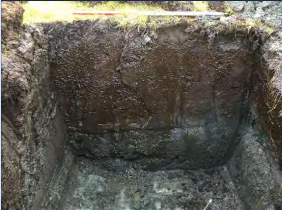
Plate 8: West facing section of TP012. A thin dark deposit is visible between the 1.03m deep layer of peat and the underlying light bluish grey clayey sand. TP012 was terminated on presumed bedrock.
