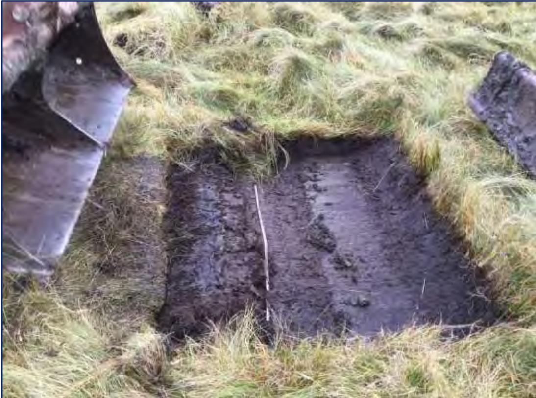
Plate 3: East facing view of TP015 showing the cable found upon opening.
