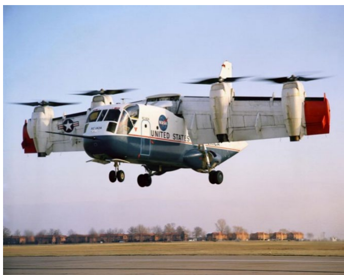
Figure A. XC-142 Tilt wing evaluated in the United States during the 1960s. Photo: NASA
