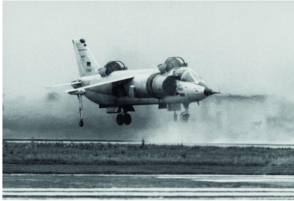
Figure 7: The VFW-Fokker VAK-191B, one of the more complex jet-lift aircraft that was built and flown in the 1970s. The vehicle is shown here in hover – a wet runway revealing some of the effects on its surroundings of the resultant outwash from the six nozzles that were used to sustain the aircraft in vertical flight. (Image source: VFW-Fokker.)
