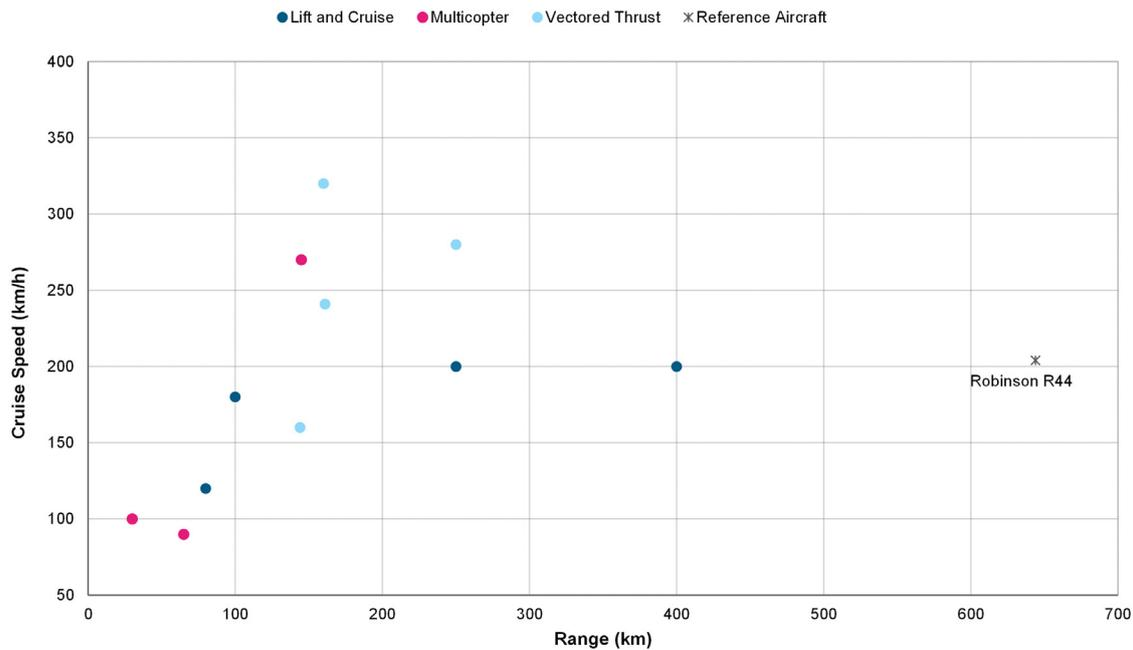
Figure 4-12 – Speed and range comparison
