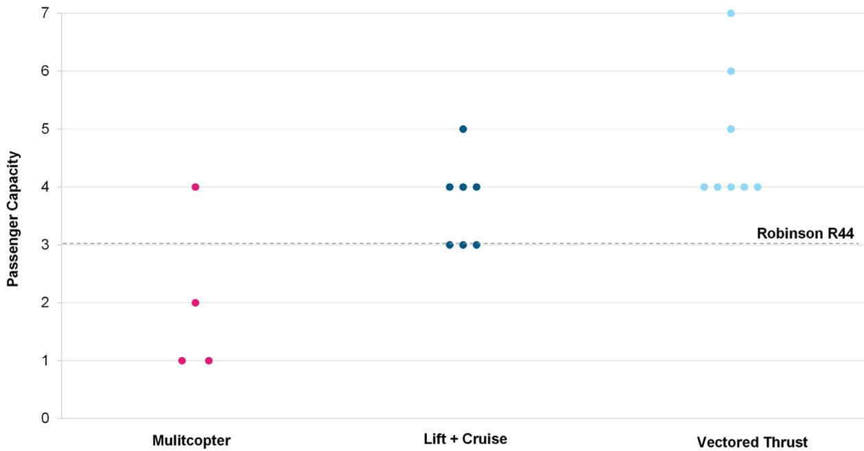
**Figure 4-2 – Variation of passenger capacity**
