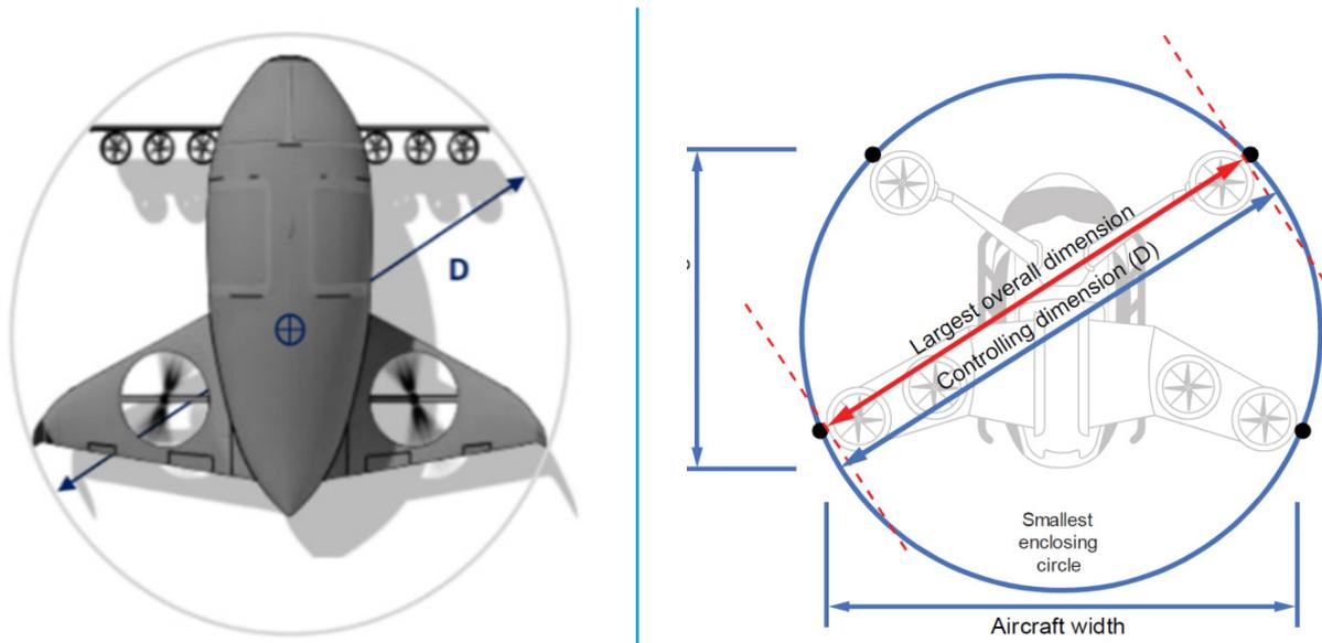
Figure 4-5 – EASA smallest enclosing circle (left) and FAA controlling dimension (right)
