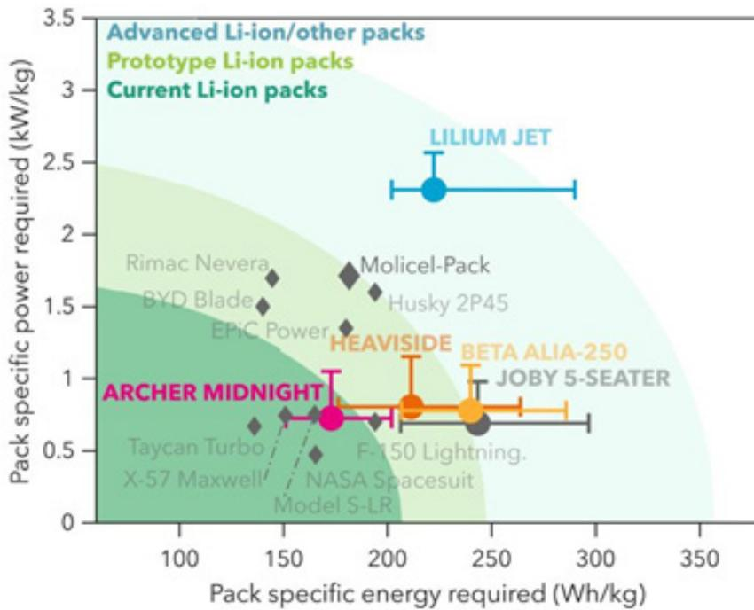
Figure 4-11 – Battery specific energy and specific power requirements
