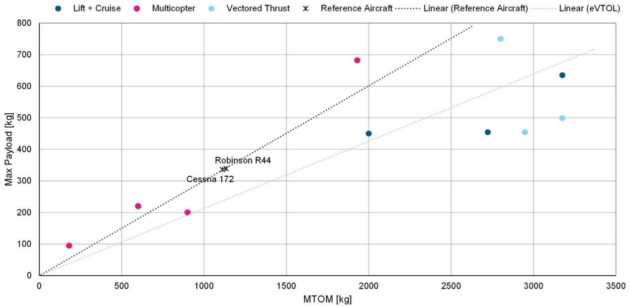
**Figure 4-3 – Relation of maximum payload mass and MTOM**
