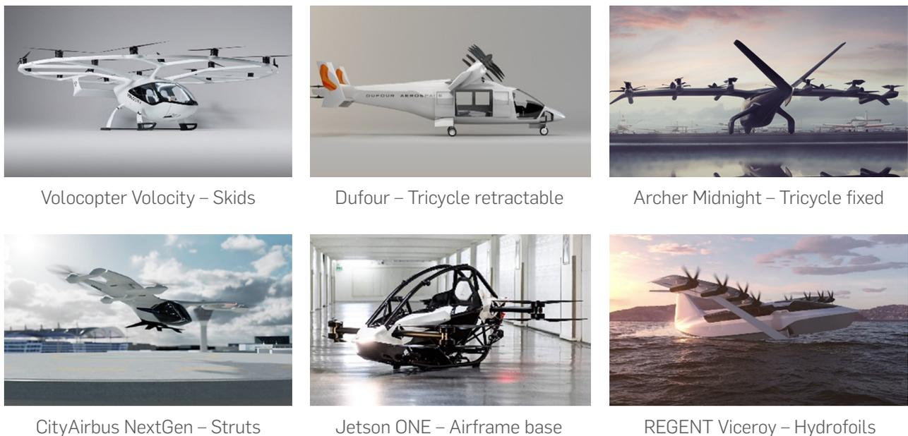
**Figure 4-7 – Landing gear configurations**
