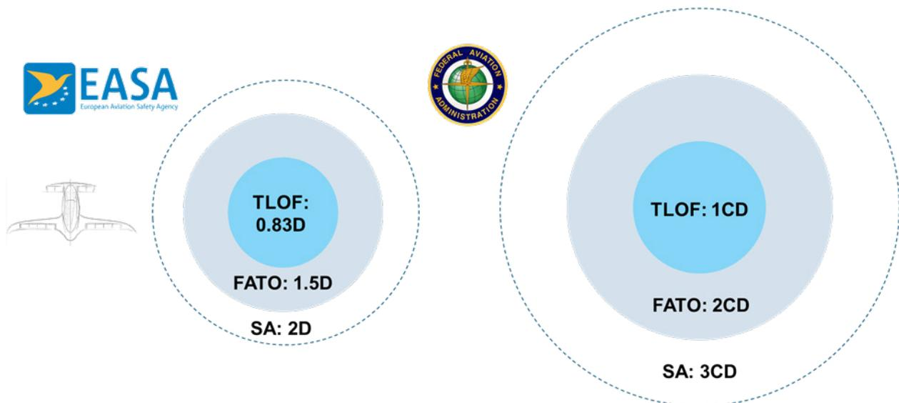
Figure 5-1 – Regulator sizing requirements
