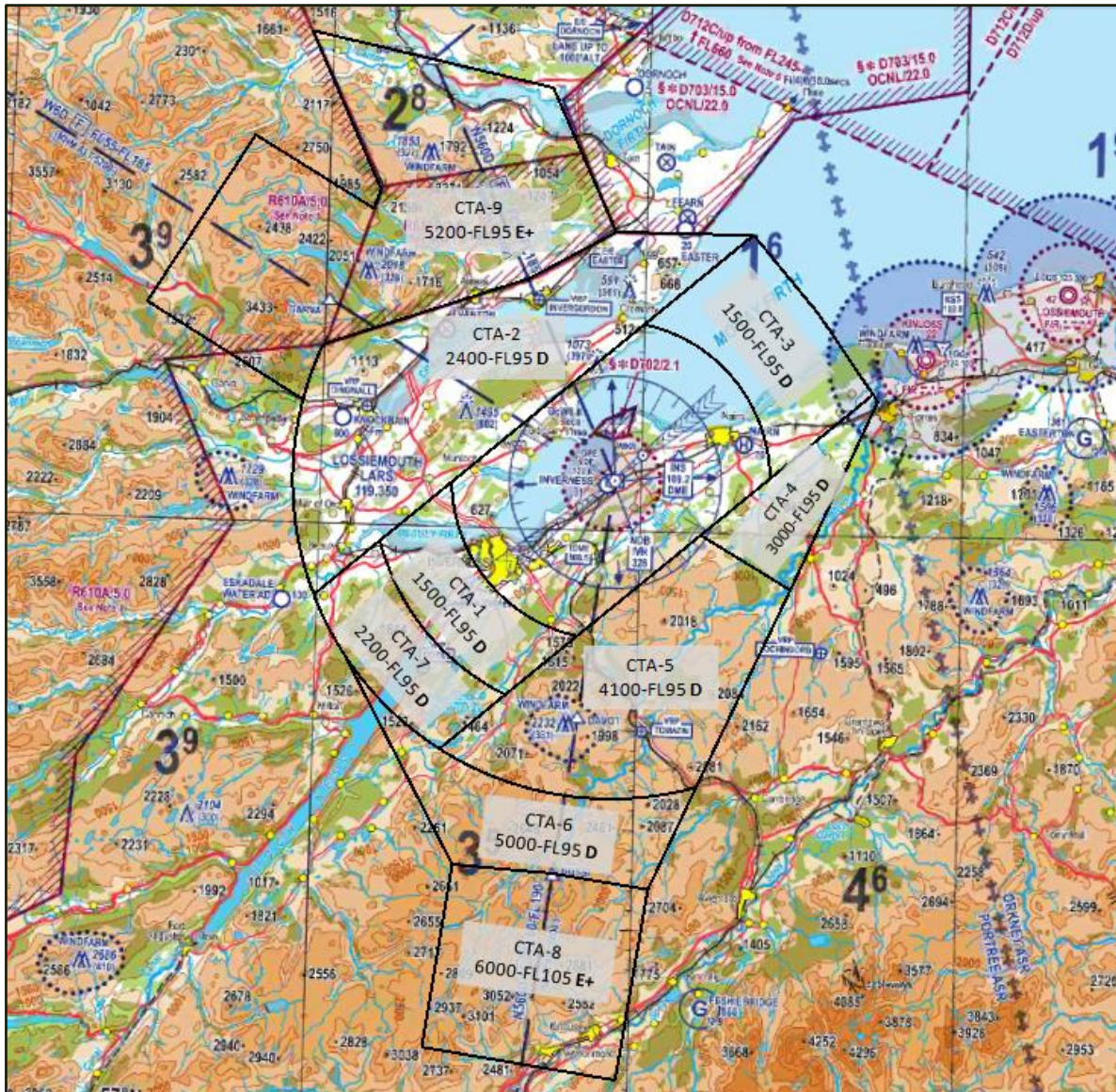
Figure 3: Proposed Inverness Airport CAS (base altitudes, top levels and airspace classification shown)
