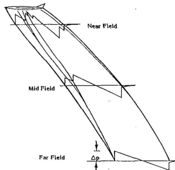
Design improvements to the shape of an aircraft cross-section can alter the N-wave signature to reduce the peak and soften the sound of the boom to an acceptable level. This will potentially enable supersonic flight over land. A level of acceptability of sonic booms has yet to be determined and may only be established by flying a demonstrator aircraft having a low-amplitude shaped signature over communities<sup>31</sup>.
