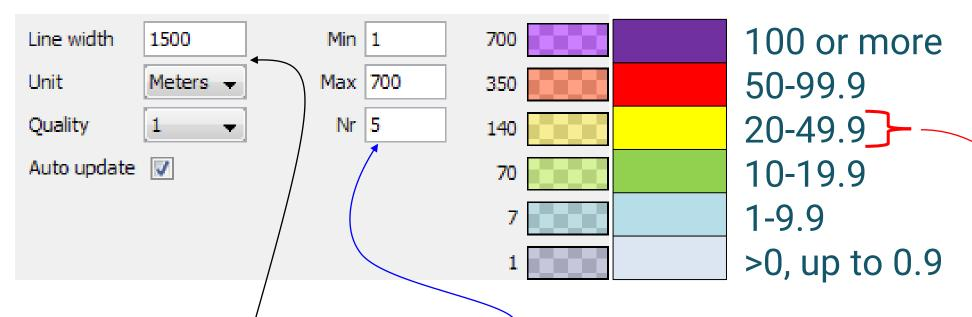
Each flight in this sample is set to be a 1500m wide track (750m either side of the radar trajectory)
