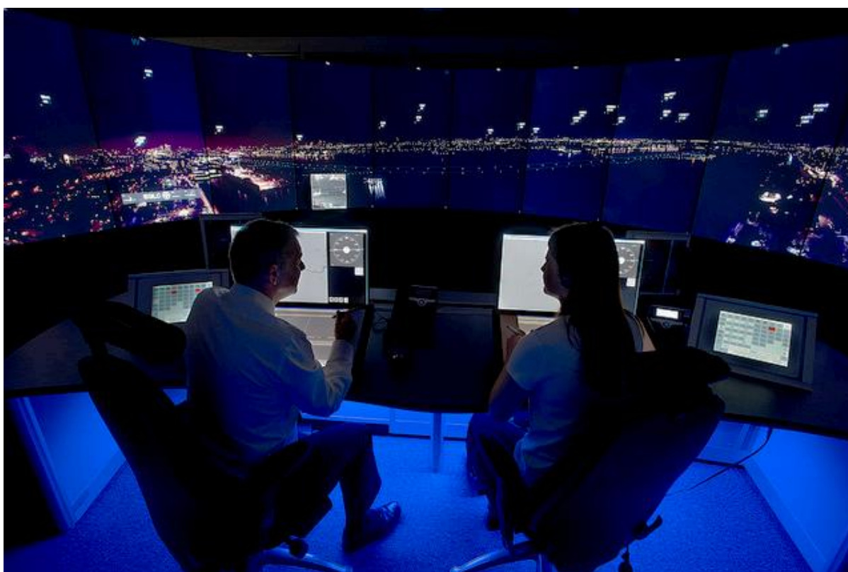
Figure 4.5 Illustration of remote air traffic control tower
