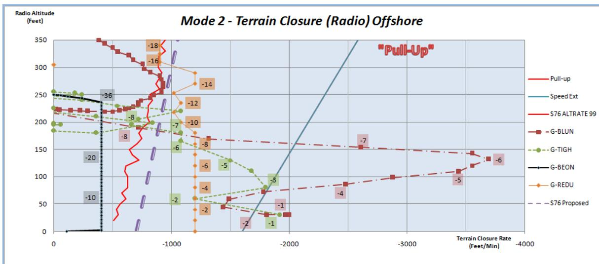
The effect of the modified Mode 2A warning envelope on the warning times for the four example accident cases is shown in the table below. The S76A+ analysis showed slightly higher rates of descent than the EC225 data for each height, which required a corresponding 'shift' in the position
