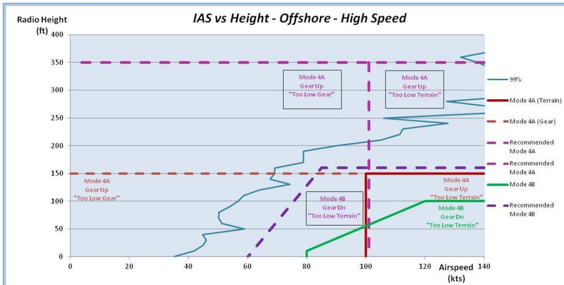
The flight path data for the four accidents has been added to the diagram below. The key to the descent rate plots for the accident data is as follows:
