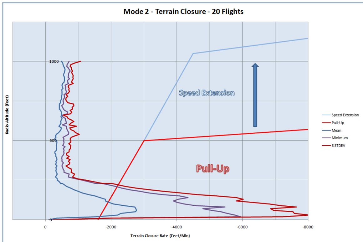
In the above example, it can be seen that the plots did not appear as expected, with the  $3\sigma$  curve exceeding the maximum. This is indicative that the data is not normally distributed, although the small dataset used in pilot study is believed to also have contributed to this result (see Section 5.2.1).
