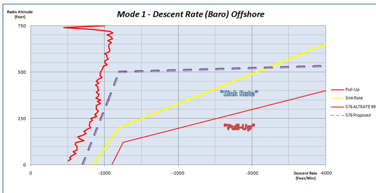
For clarity the second diagram only shows the last 350ft of the rate of descent profile, to which the FDR data from the four accident cases has been added. The key to the descent rate plots for the accident data is as follows:
