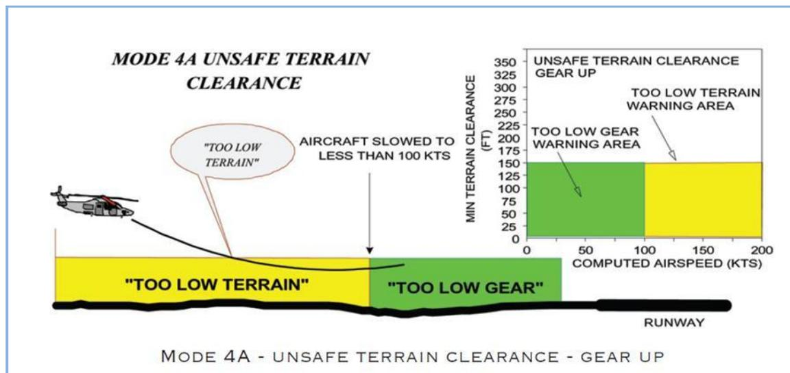
Fixed, non-retractable landing gear aircraft do not provide Mode 4A.
