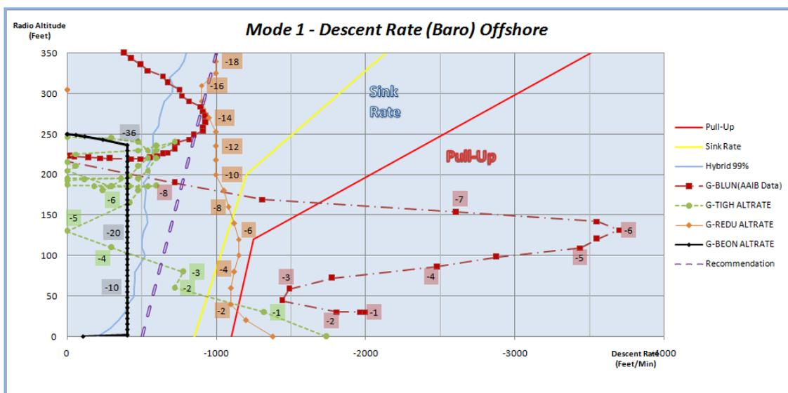
As can be seen, useful warnings are generated by current HTAWS at 7.5 seconds ('Sink Rate') and 7 seconds ('Pull Up') in the case of G-BLUN, and at 7 seconds ('Sink Rate') for G-REDU. With the proposed new warning envelope, the G-BLUN warning time would be improved
