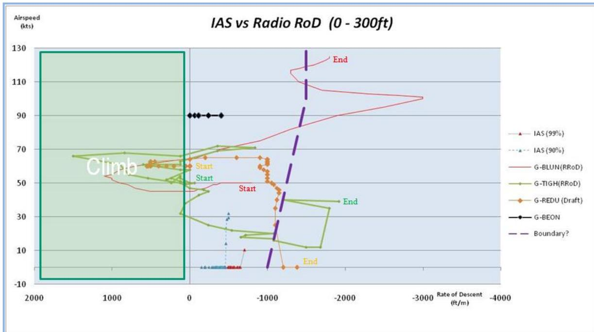
As can be seen, no additional discrimination resulted and, overall, envelopes based on IAS vs RoD did not appear to offer any advantage over existing envelopes.
