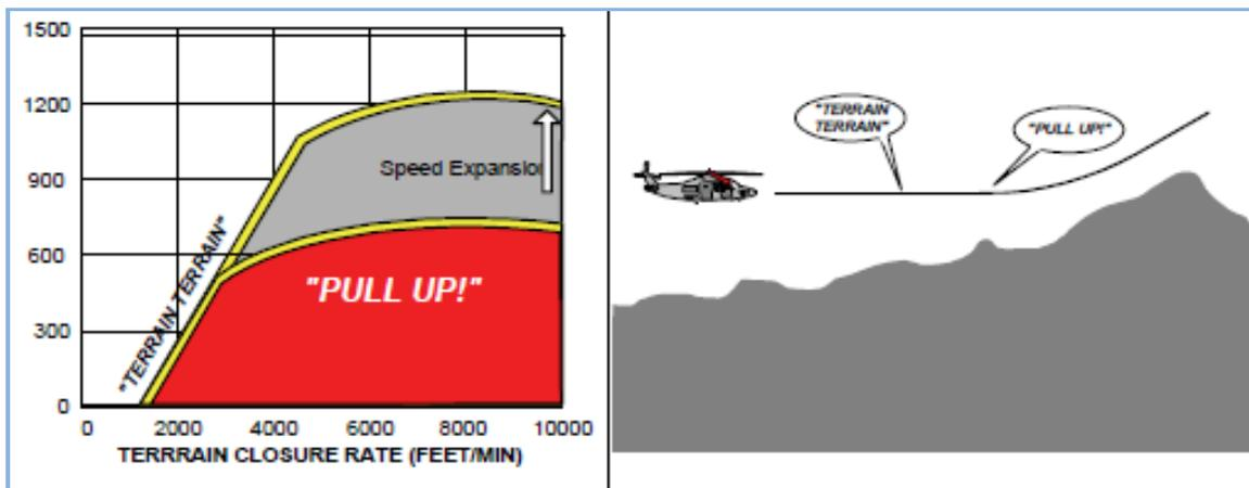
MODE 2A - EXCESSIVE TERRAIN CLOSURE RATE
