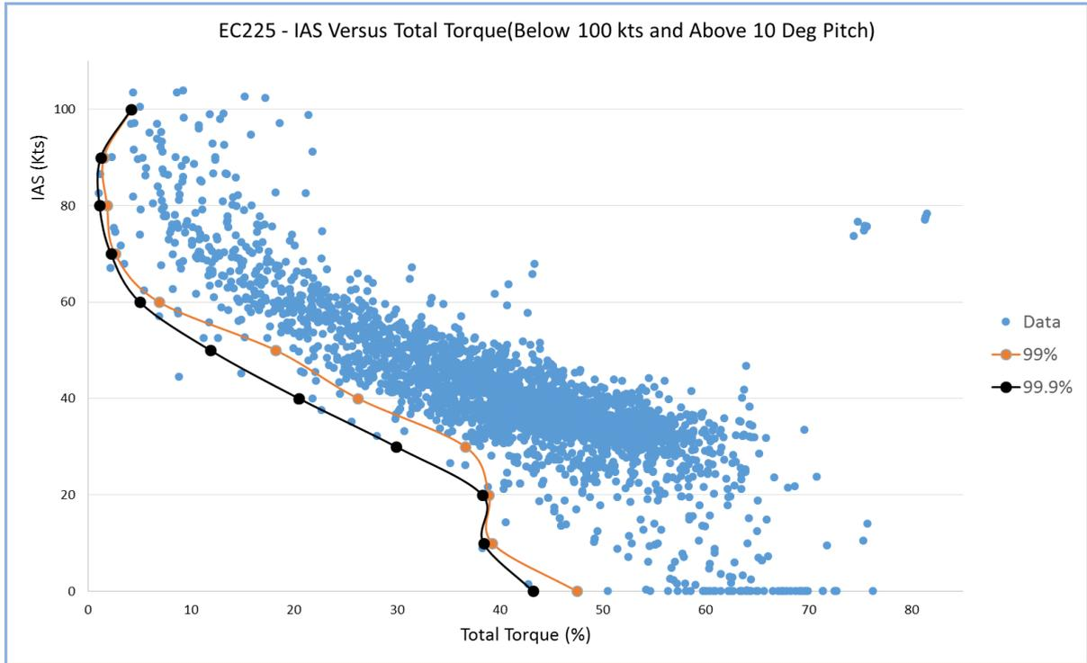
To illustrate the potential that a warning envelope based on airspeed and total torque may have, the 99 percentile envelope was used to determine warning times for the G-BLUN, G-REDU and G-WNSB accidents and an incident provided to the project in confidence (S92 incident). The resultant plot and a table of the warning times are presented below.
