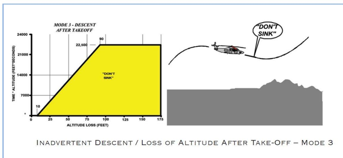
As the pilot adjusts the flight path of the aircraft and a positive rate of climb is re-established, the voice alert “Don’t Sink” will cease and the amber caution annunciation will extinguish. Note:
