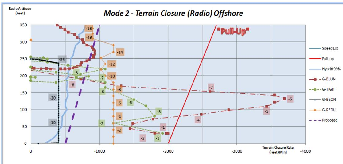
As can be seen, a warning is generated by current HTAWS for one accident case only (G-BLUN) and this is of limited use as it triggers at 7 seconds prior to impact and then ceases three seconds later; the flight crew might interpret this as meaning the danger had passed. With the proposed new warning envelope, the G-TIGH warning time would be increased
