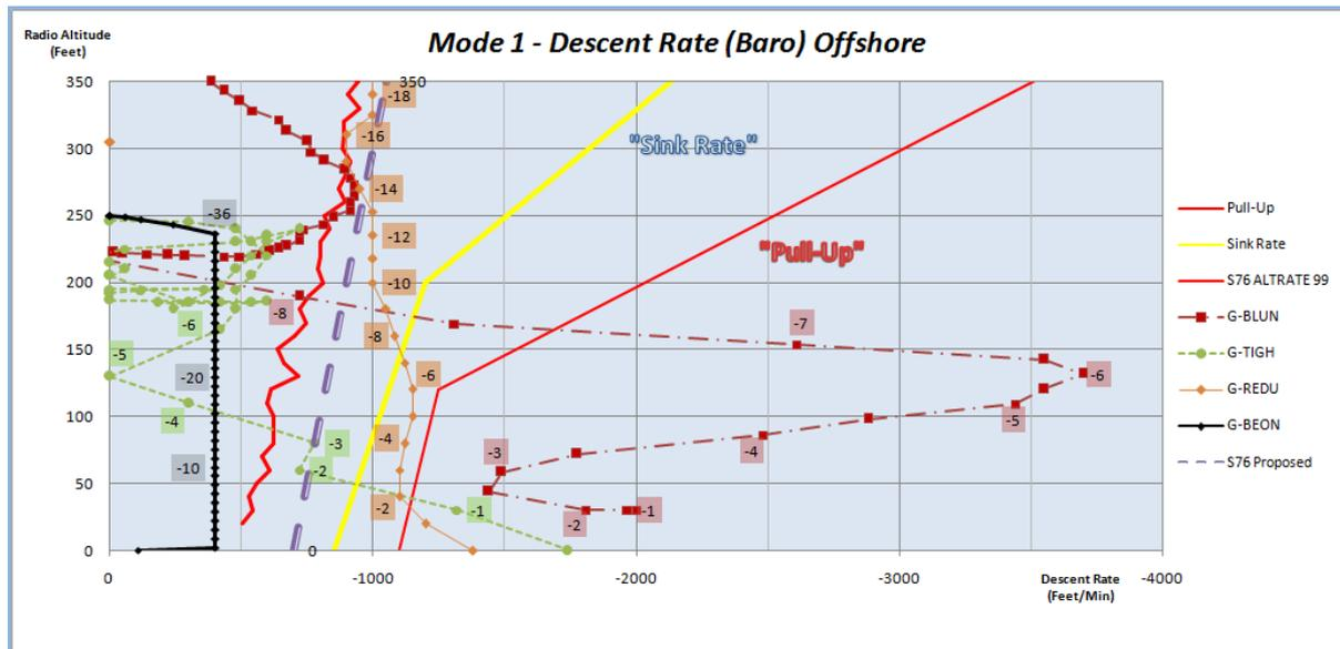
The effect of the modified Mode 1 warning envelope on the warning times for the four example accident cases is shown in the table below. The S76A+ analysis showed slightly higher rates of descent than the EC225 data at each altitude, which required a corresponding 'shift' in the position of the recommended envelope. The impact of this 'shift' was to slightly reduce the improvement in warning time for G-TIGH and G-REDU, as shown in the table below.
