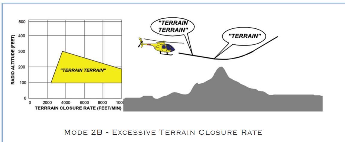
MODE 2B - EXCESSIVE TERRAIN CLOSURE RATE
