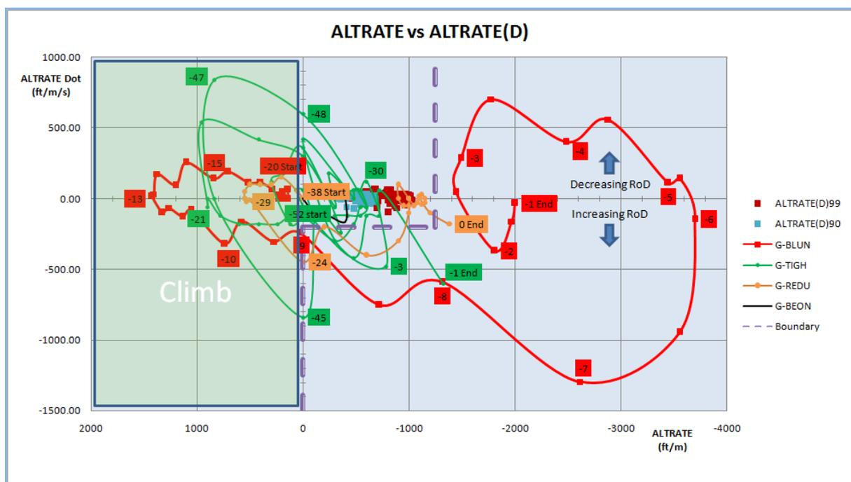
From the above plot, it appears as though normal operations are confined to a relatively small area defined by the cluster of light blue (90%) and red (99%) points to the right of the origin. With this in mind a possible boundary line was drawn which excluded all climbing flight as well as the 99% data and would produce a warning where either rate of descent is abnormally high, or is increasing abnormally.
