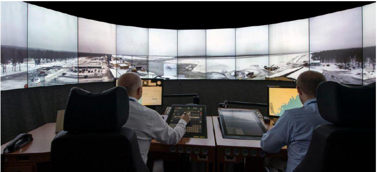
**Figure 7: Remote Tower technology. Picture by Stefan Kalm, copyright Saab AB.**
