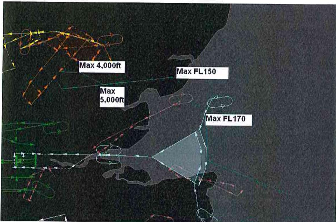
**Figure 2- LAMP Phase1a airspace modelled in AirTop with Stansted CLN easterly and westerly SIDs as well as connecting airway (U)L12 highlighted**
