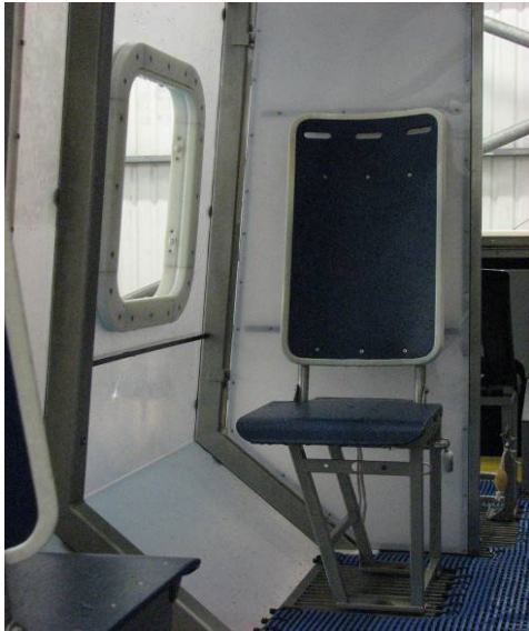
Figure 4: HUET seat position in helicopter simulator
