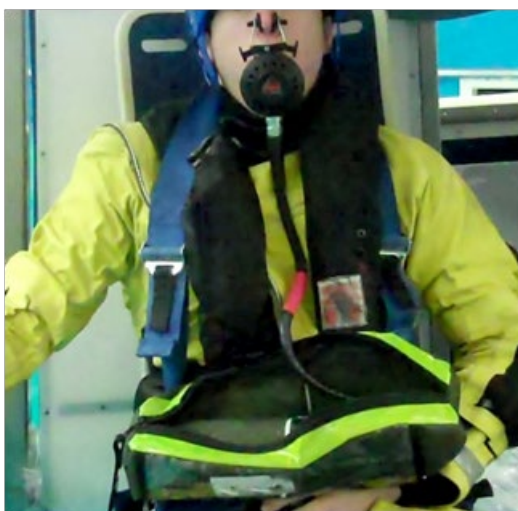
Figure 2: Compressed Air EBS
