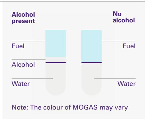
While commercial testing kits are available, testing for ethanol can also be carried out as follows:
