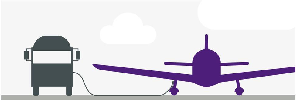
Static electricity can build up during fuelling, especially in cold and dry weather. A static discharge is a potential source of a spark and therefore ignition. To minimise the risk, electrical ‘bonding’ and/or ‘earthing’ is used to neutralise differences in electrical potential between refuelling components or the aircraft. This should ensure that static discharge sparks do not occur.
