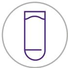
Add water to the tube until it comes to the line. Now fill the tube with your fuel sample until it is near the top.
