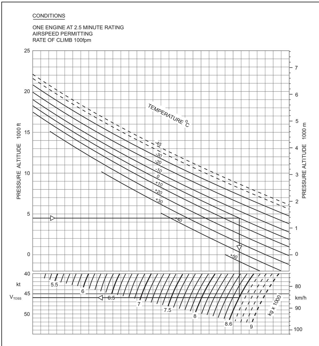
**Figure 3.39** Take-Off Safety Speed ( $V_{TOSS}$ ) Determination
