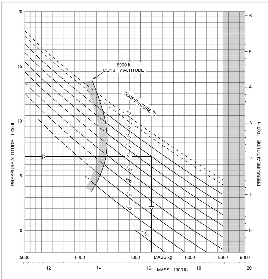
**Figure 3.36** Maximum Permissible Take-Off Mass on Helipad
