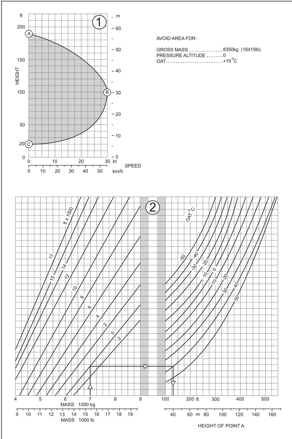
**Figure 3.5** Airspeed-Height Envelope
