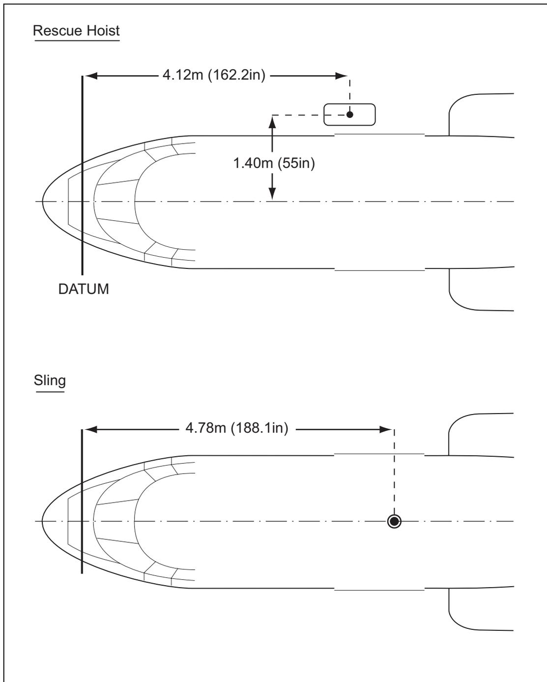
**Figure 3.26** Longitudinal and Lateral Location of External Loads
