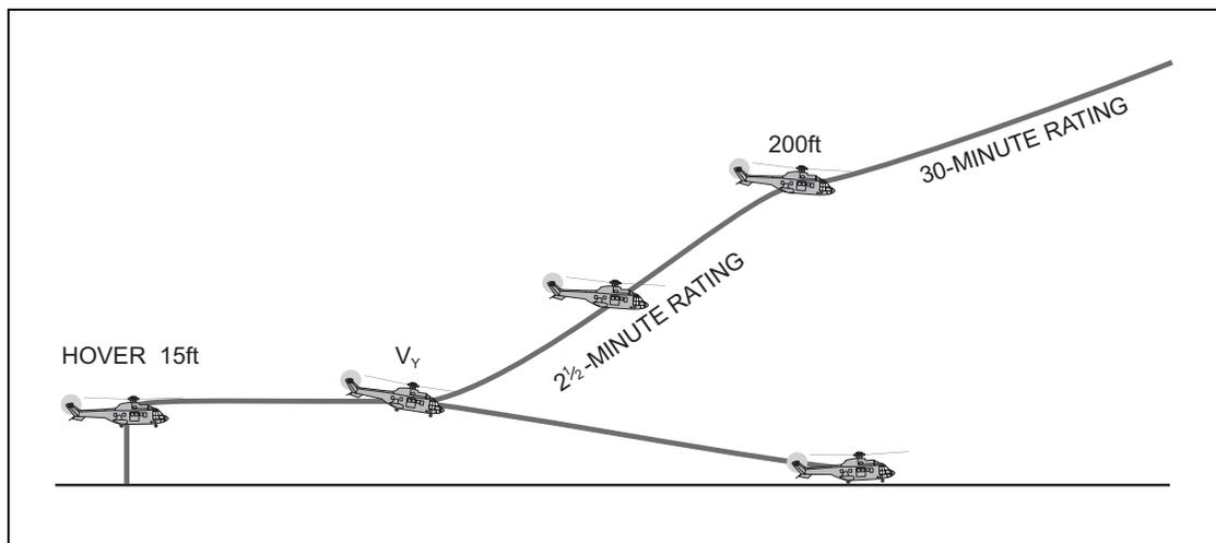
**Figure 3.33** Engine Failure at Take-Off – Procedure No. 2
