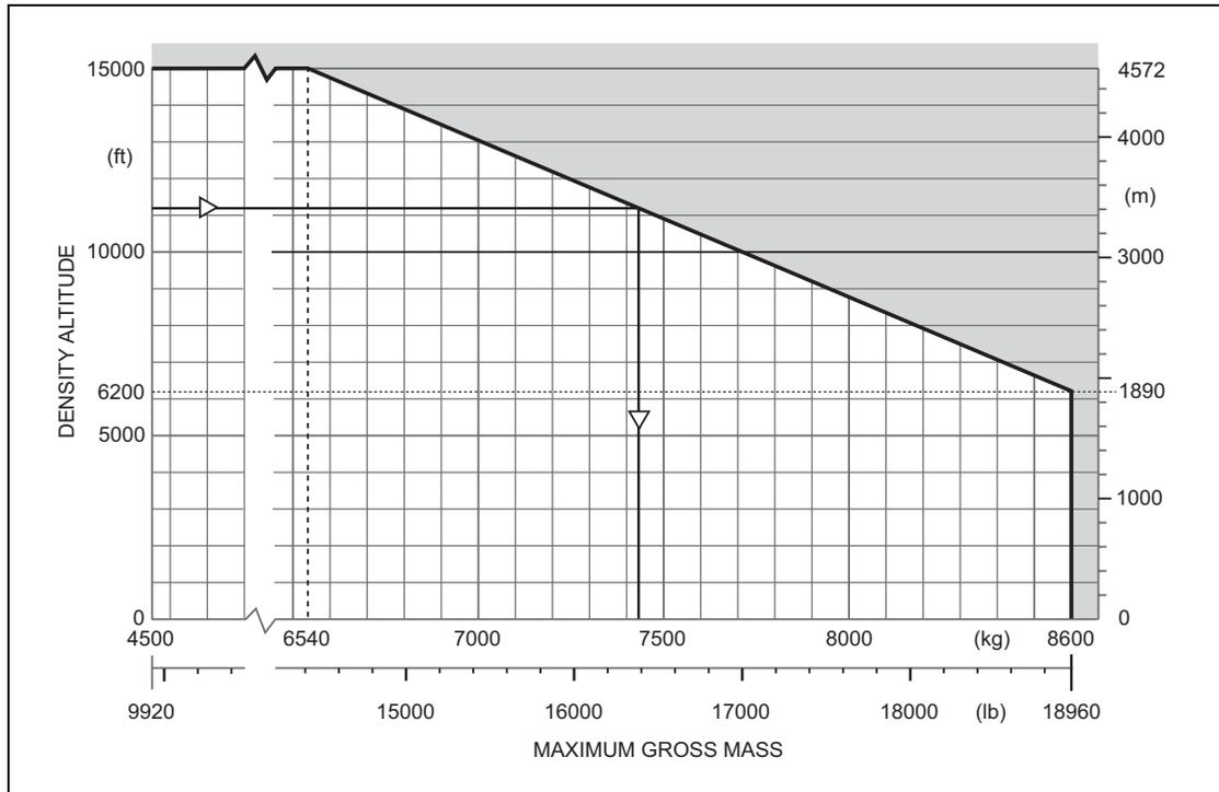
**Figure 3.2** Mass Limitations for Take-Off and Landing with Internal Loads
