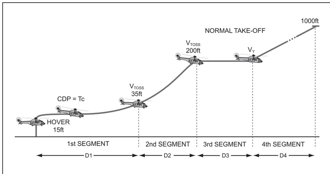
**Figure 3.30** Normal Take-Off – Procedure No. 1
