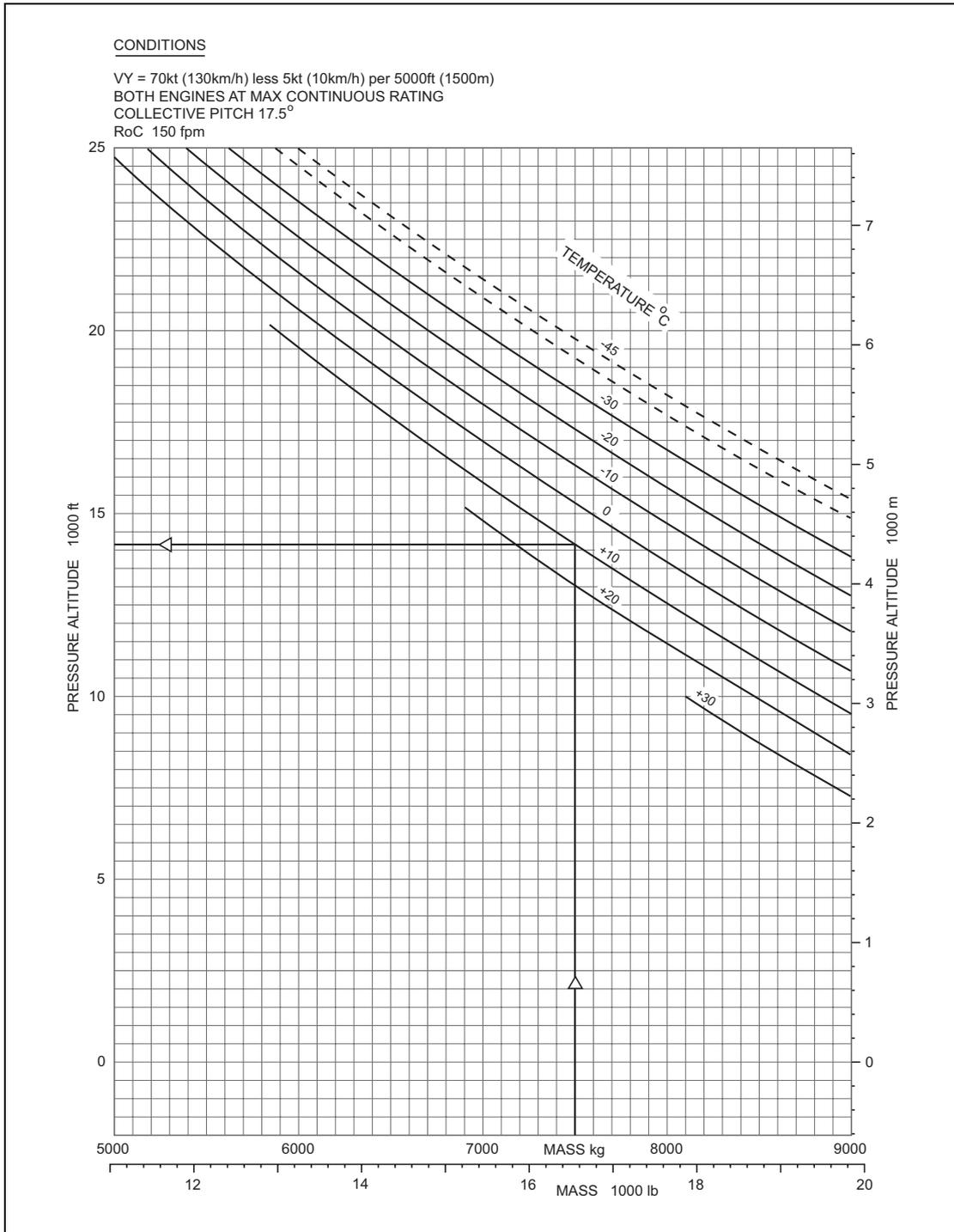
**Figure 3.16** Service Ceiling – Two Engines
