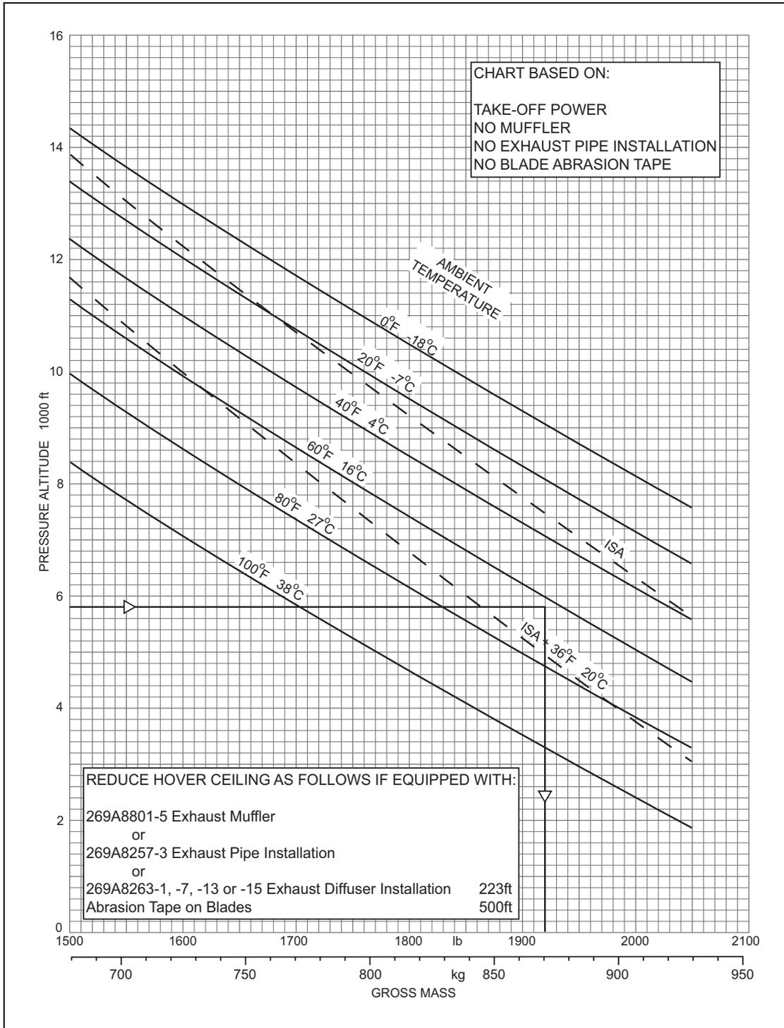
**Figure 2.7** Hover Ceiling v. Gross Mass (2-ft Skid Height, 3,200 rpm, 80% Relative Humidity) IGE
