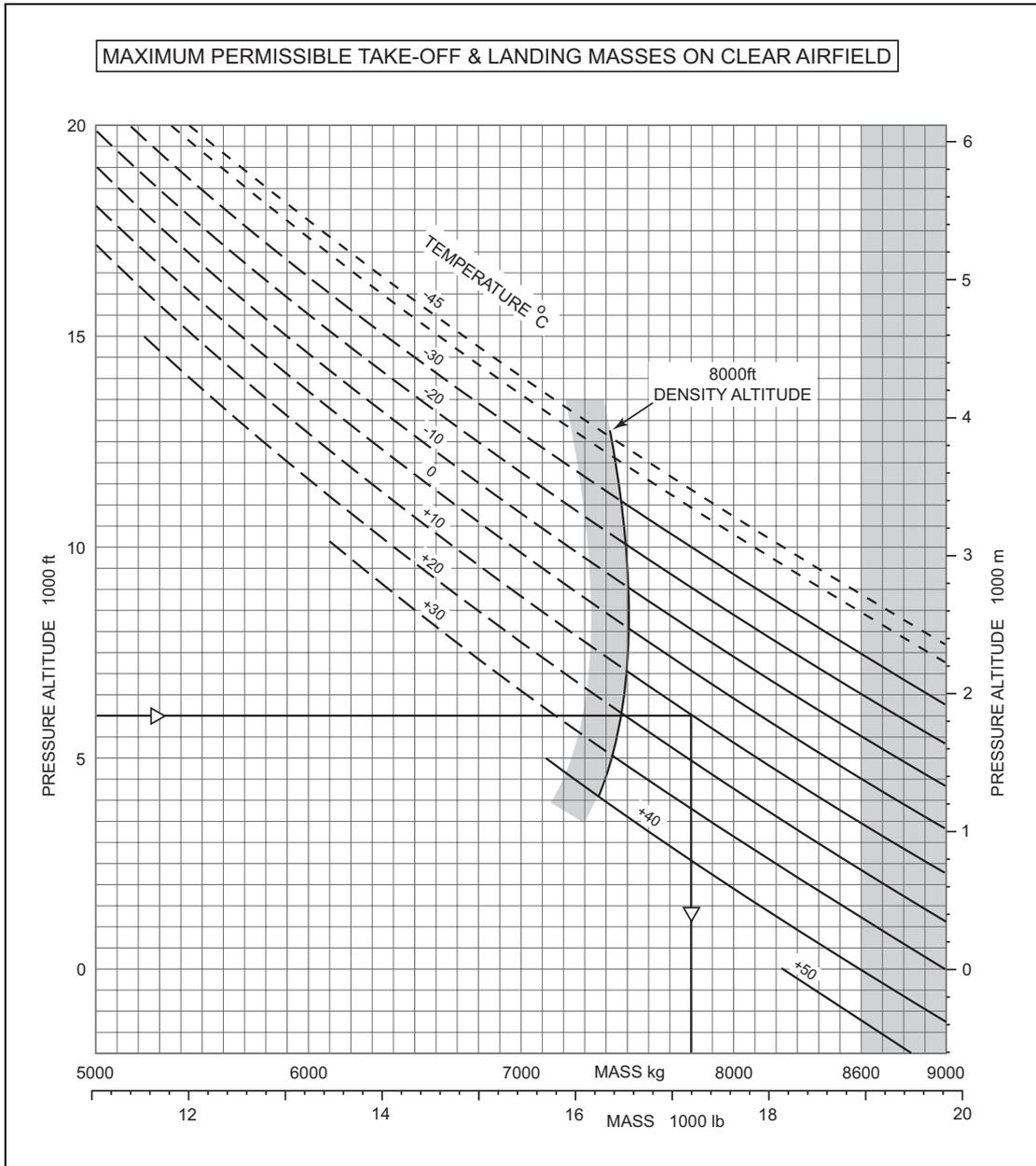
**Figure 3.29** Maximum Permissible Take-Off and Landing Masses on Clear Airfield
