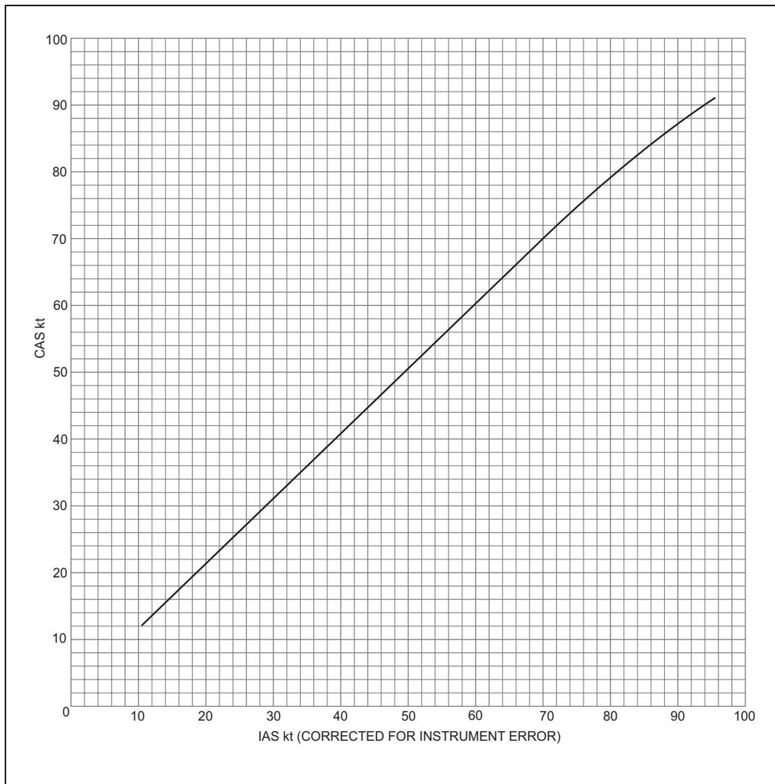
**Figure 2.2** Airspeed Calibration Curve
