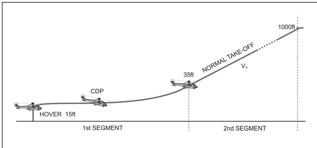
**Figure 3.31** Normal Take-Off – Procedure No. 2
