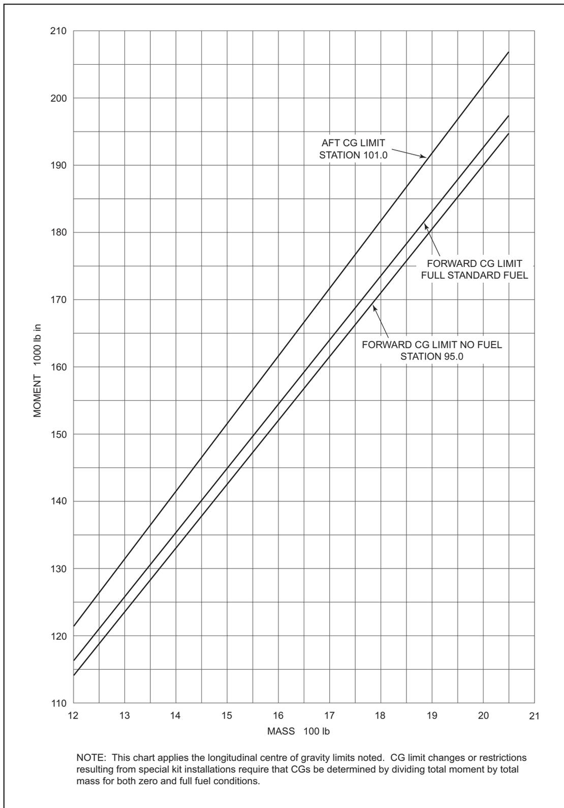
**Figure 2.15** Mass and Moment Loading Chart – Longitudinal Limitations
