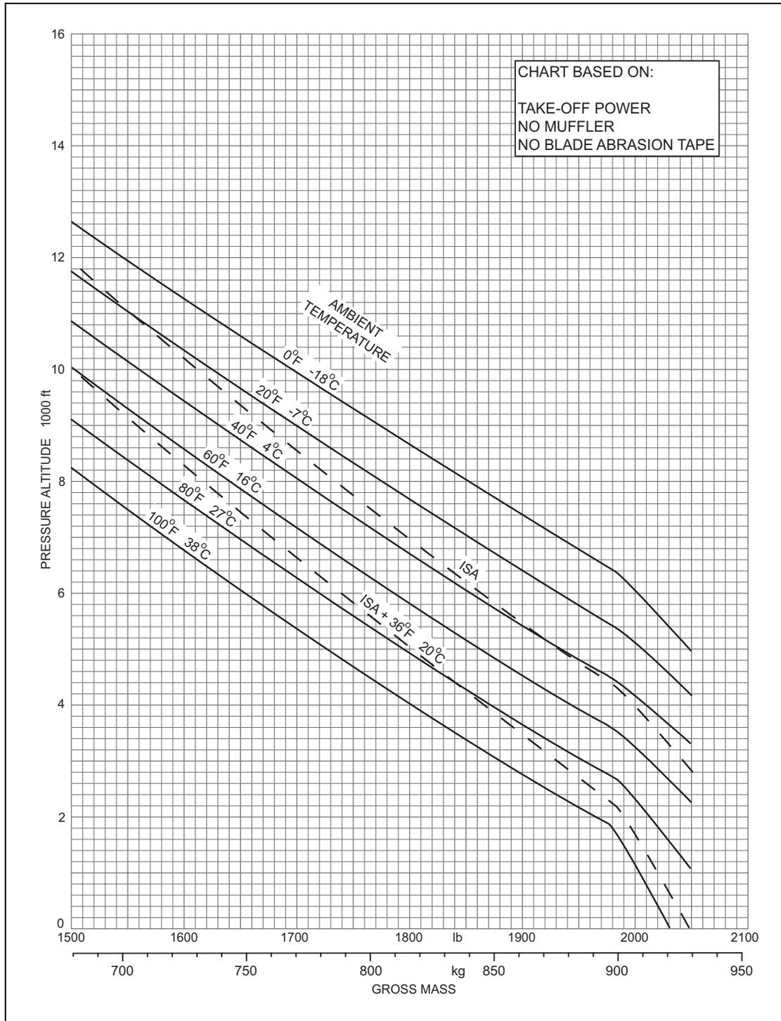
**Figure 2.18** Hover Ceiling v. Gross Mass (3,200 rpm) out of Ground Effect
