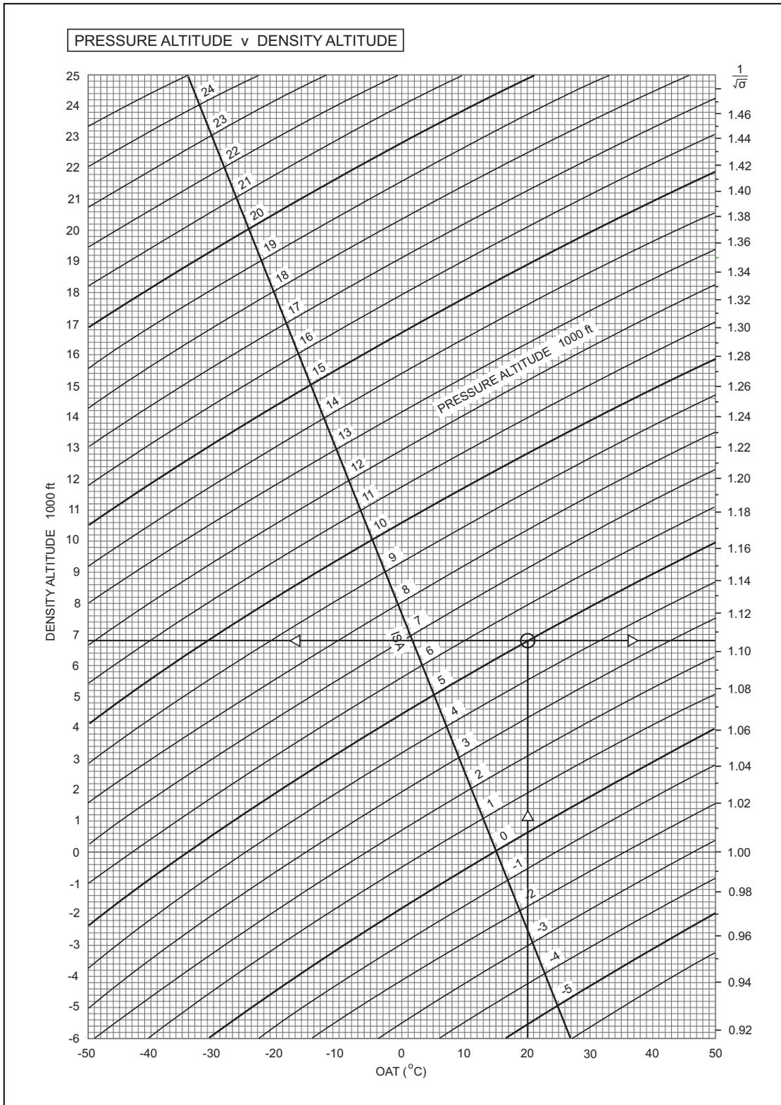
**Figure 1.1** Pressure Altitude v. Density Altitude Chart
