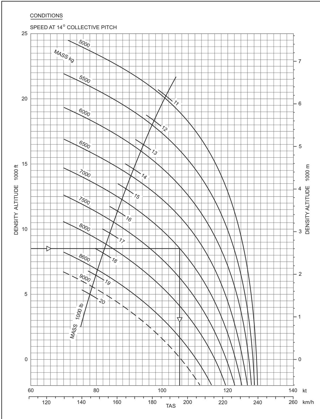
**Figure 3.28** Speed in Level Flight in Icing Conditions – Two Engines
