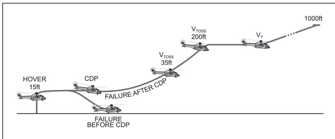
**Figure 3.32** Engine Failure at Take-Off – Procedure No. 1
