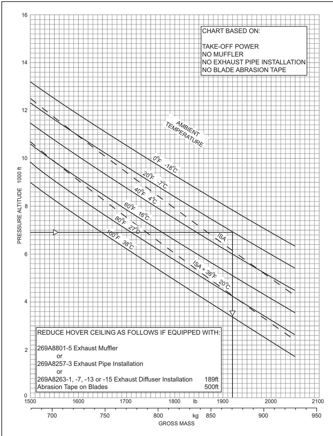
**Figure 2.8** Hover Ceiling v. Gross Mass (2-ft Skid Height, 3,000 rpm) IGE
