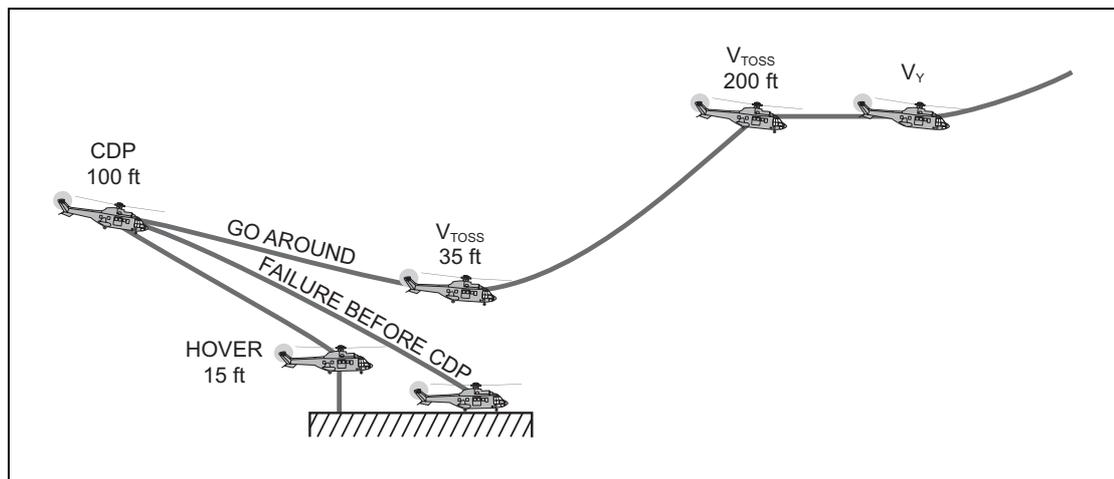
**Figure 3.38** Engine Failure at Take-Off from Helipad
