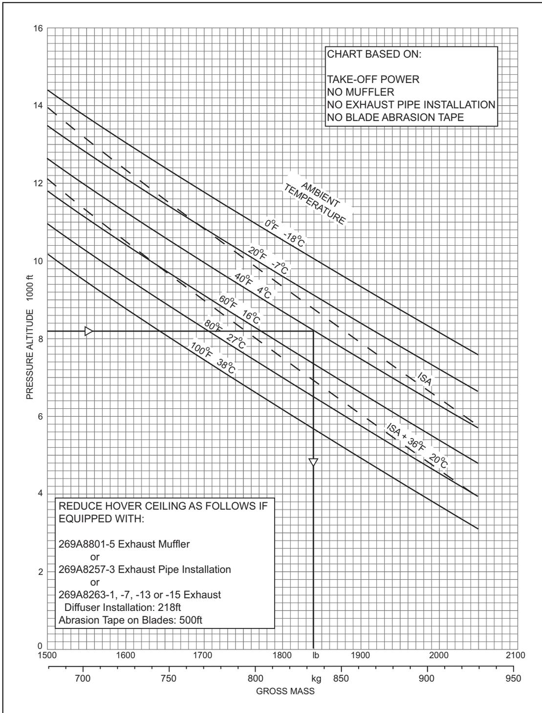
**Figure 2.6** Hover Ceiling v. Gross Mass (2-ft Skid Height, 3,200 rpm) IGE
