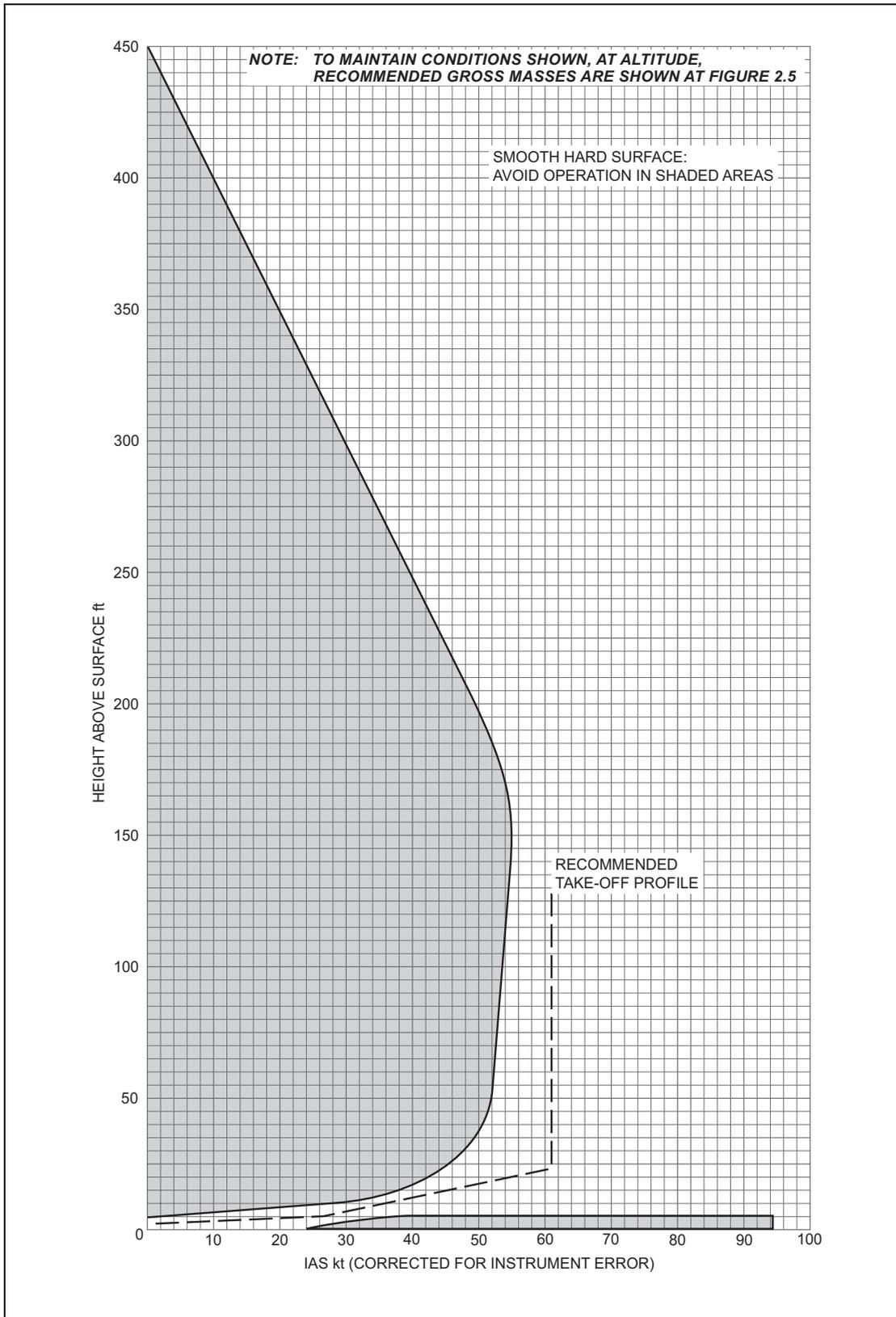
**Figure 2.4** Height v. Velocity at Sea Level
