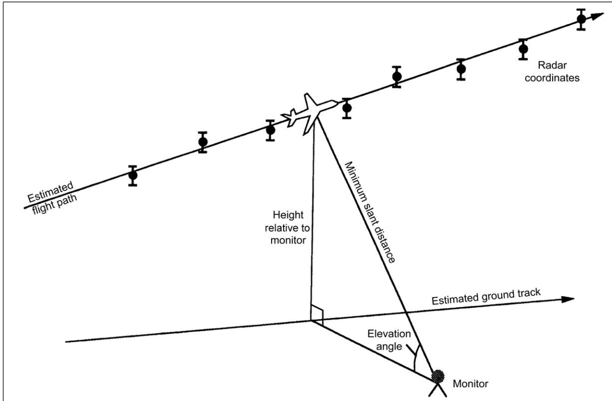
**Figure 8** Calculation of Source-to-Receiver Geometry
