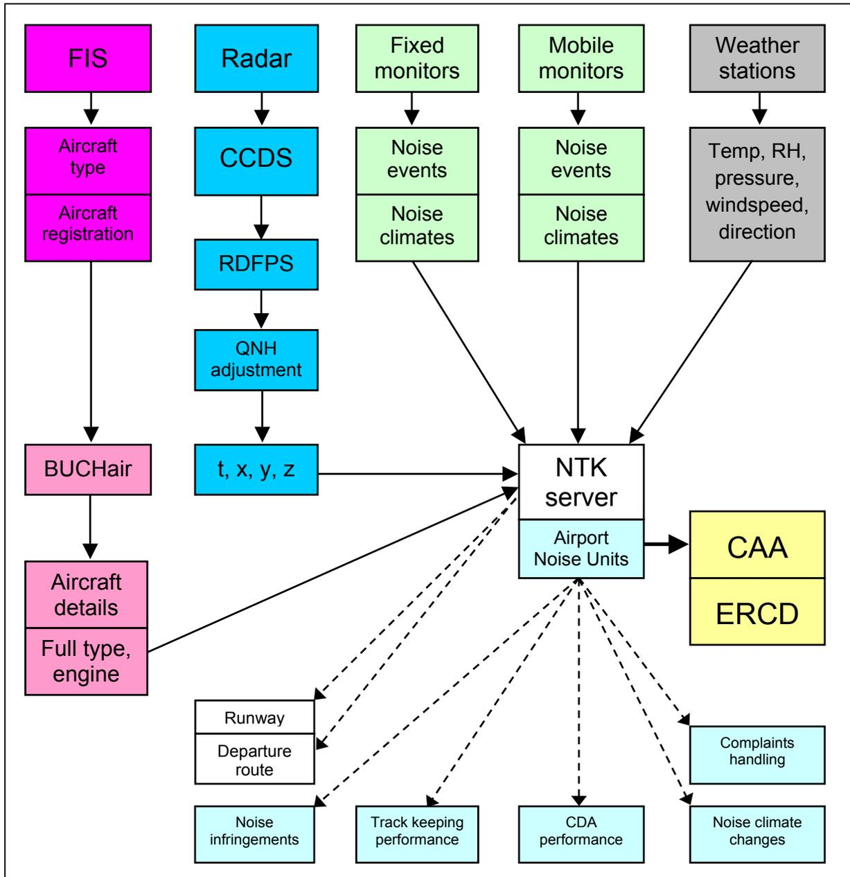
Figure A1 Data Inputs to and Typical Outputs from the NTK System
