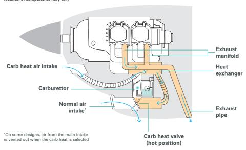
When carburettor heat selected to hot, the engine power will reduce slightly, due to the reduced density of hot air. This loss in power should not be confused with the effects of carburettor icing.
