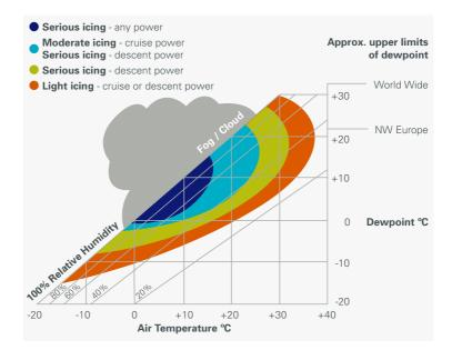
The chart above shows the wide range of ambient conditions conducive to the formation of carburettor icing for a typical light aircraft piston engine. Note the greater risk of serious icing at descent power.
