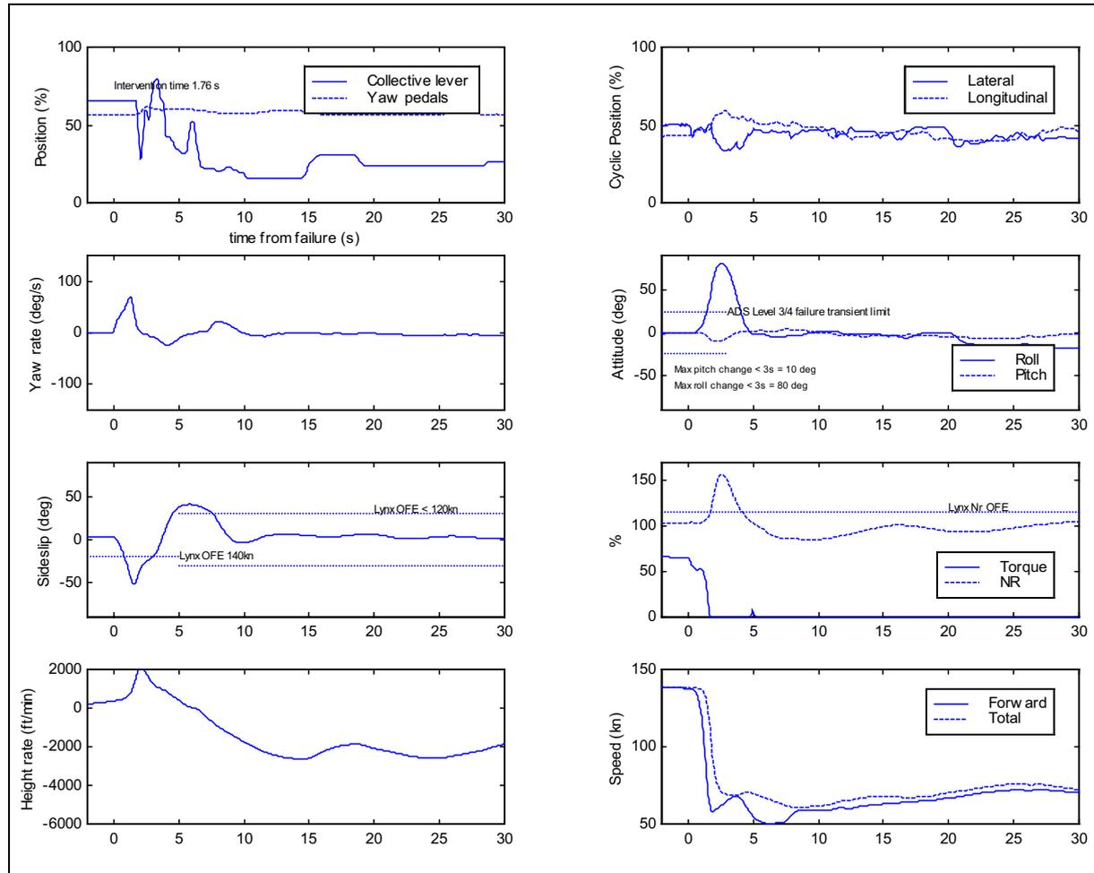
**Figure 6-30** Time histories for transient phase of TRDF at high speed (P3, drag chute)
