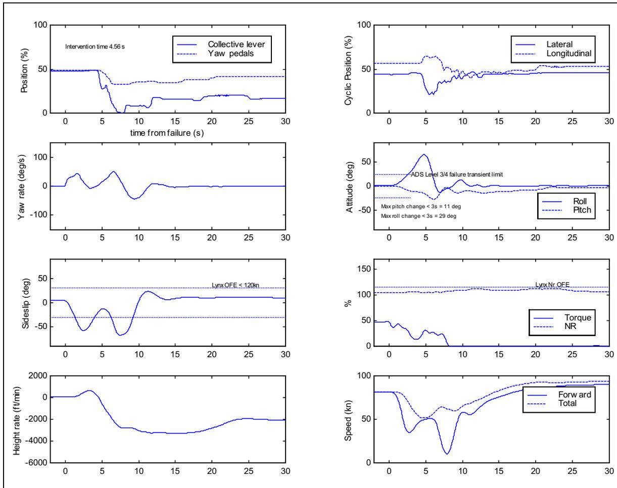
**Figure 6-45** Time histories for transient phase of TRDF at mid speed (P3, articulated MR, enlarged fin, delayed reaction)
