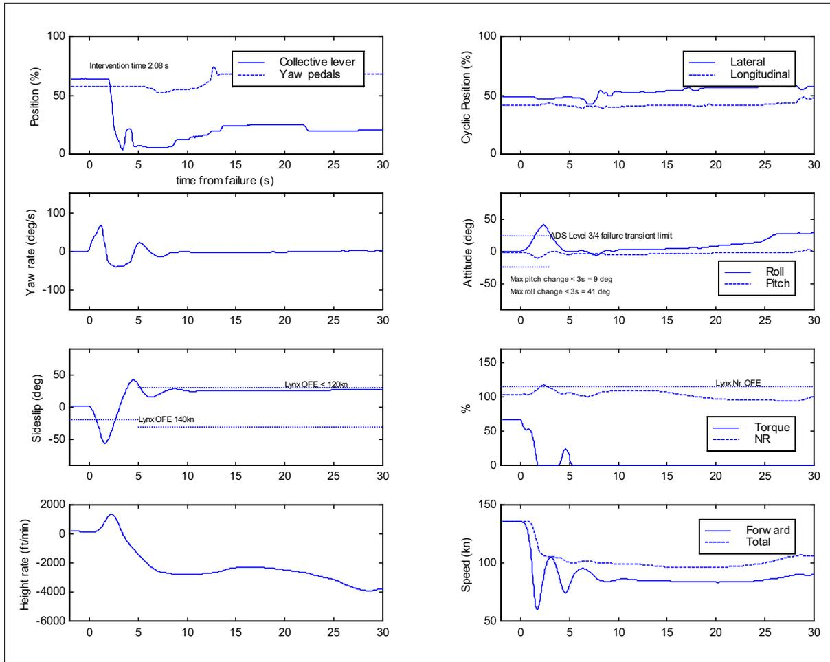
**Figure 6-32** Time histories for transient phase of TRDF at high speed (P2, AFCS authority)
