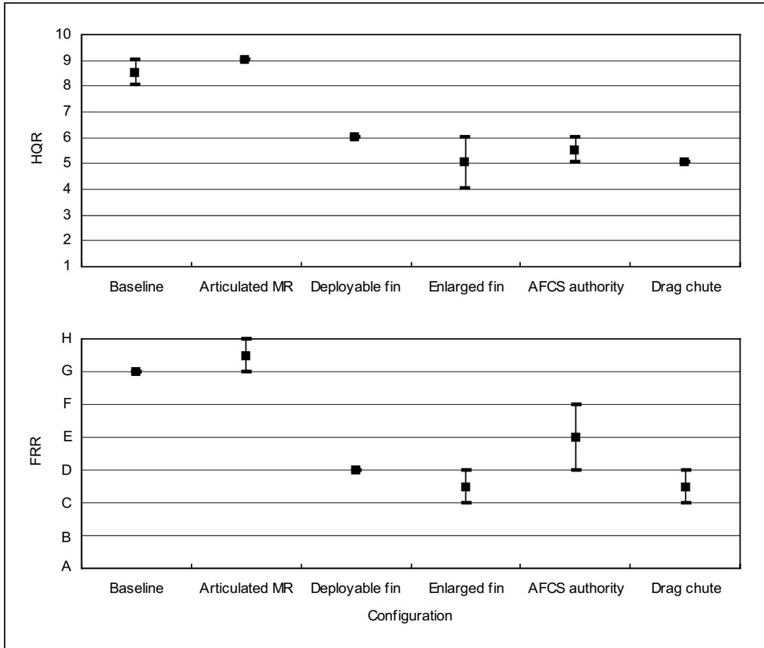
**Figure 6-35** Pilot ratings for transient phase of TRDF at high speed
