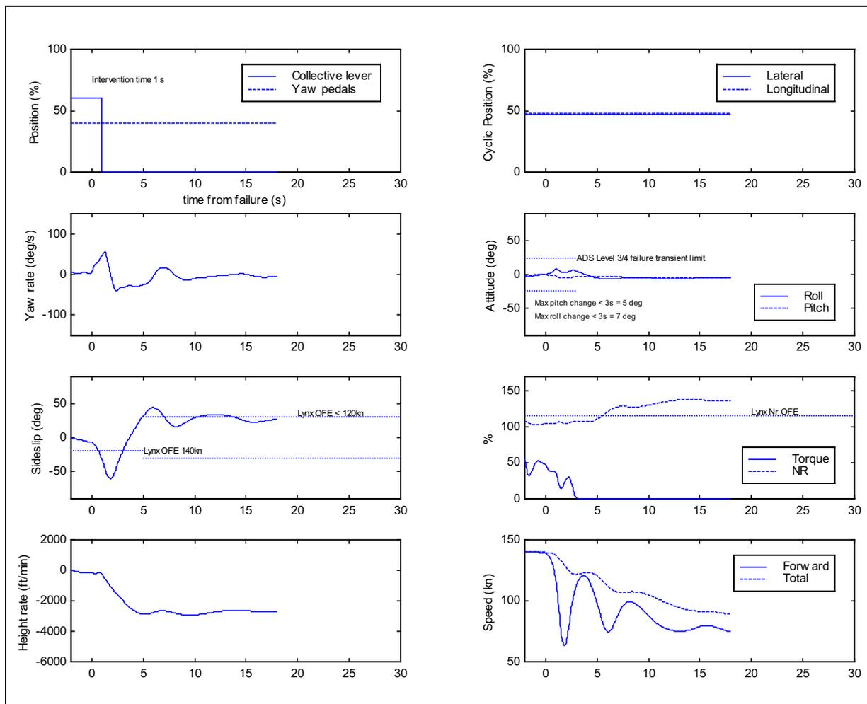
**Figure 2-1** Off-line simulation of 140 kn TRDF with 1 s PIT
