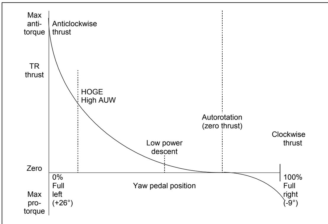
**Figure B-1** TR thrust variation with pedal position
