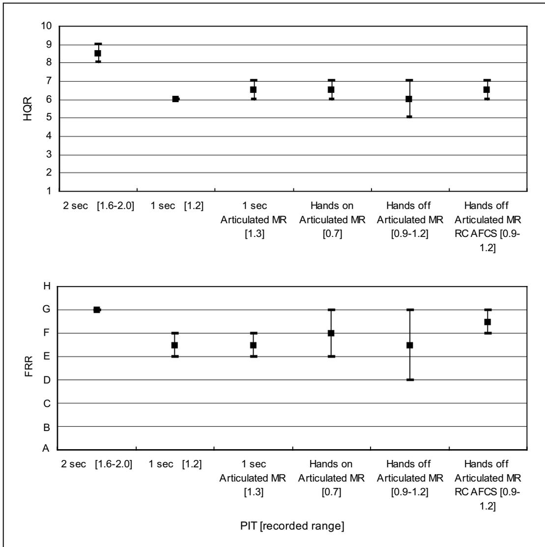
**Figure 6-36** Pilot ratings for various PITs for transient phase of TRDF at high speed
