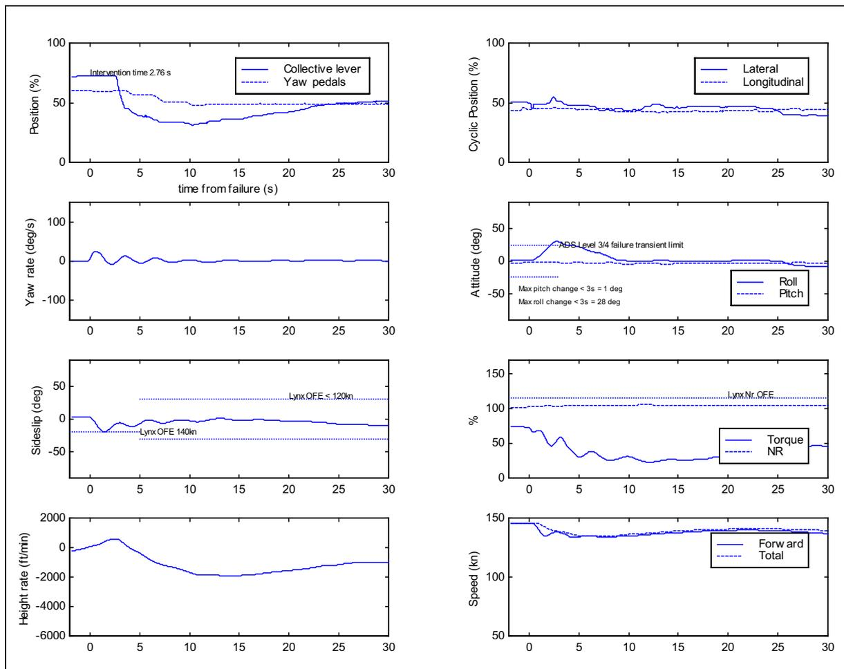
**Figure 6-4** Time histories for transient phase of TRDF at high speed (P1, MYR 2)
