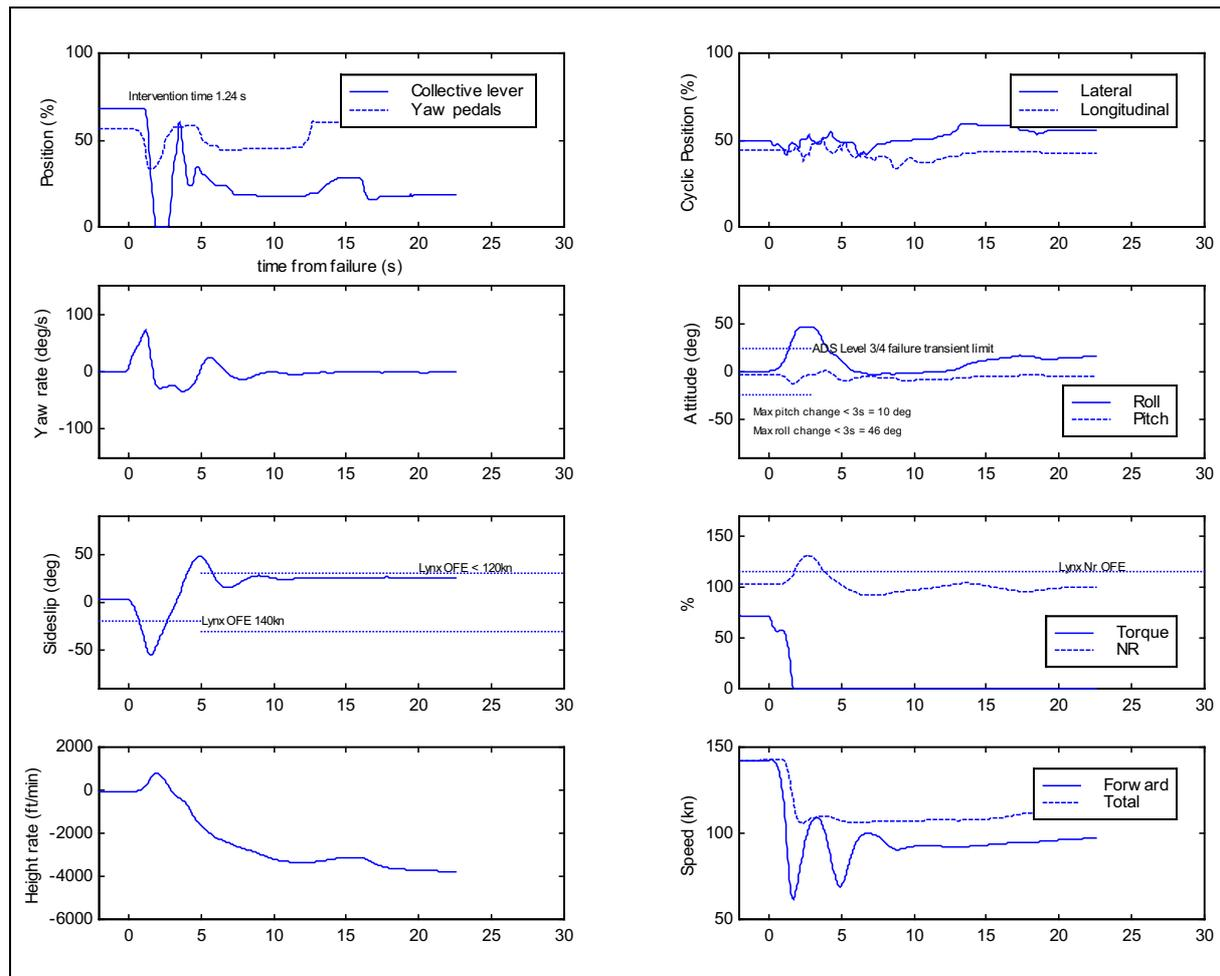
**Figure 6-33** Time histories for transient phase of TRDF at high speed (P2, warning device)
