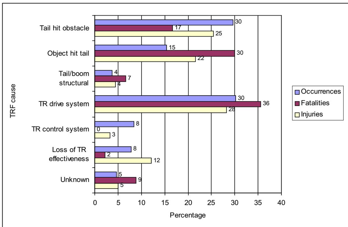
**Figure 2-5** Distribution of TRF causes (all aircraft)
