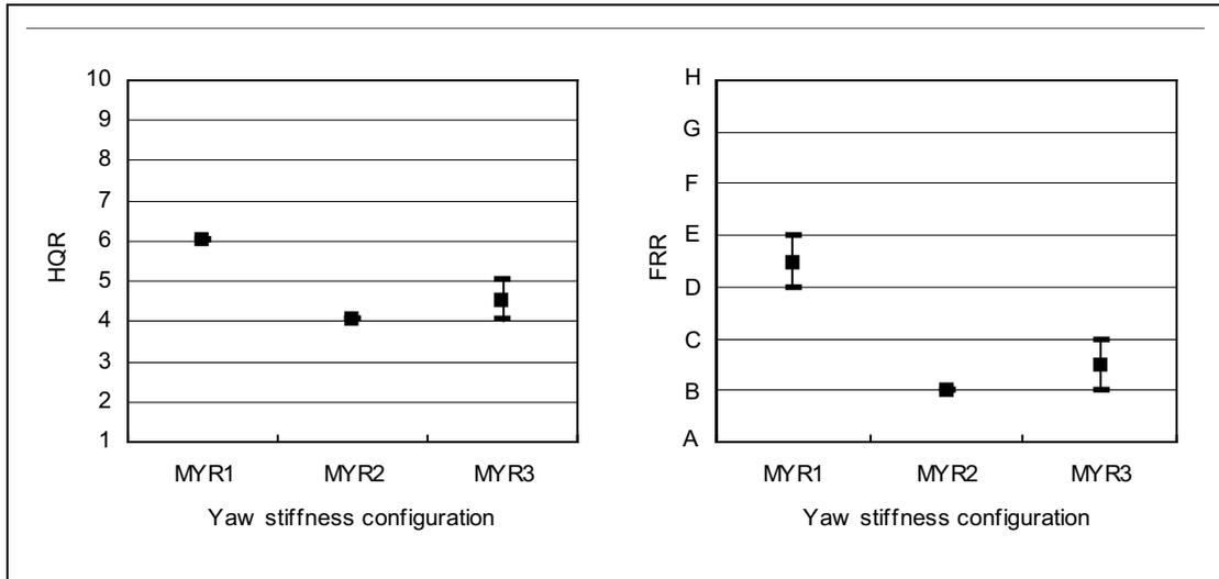
**Figure 6-18** Pilot ratings for transient phase of LP TRCF at high speed
