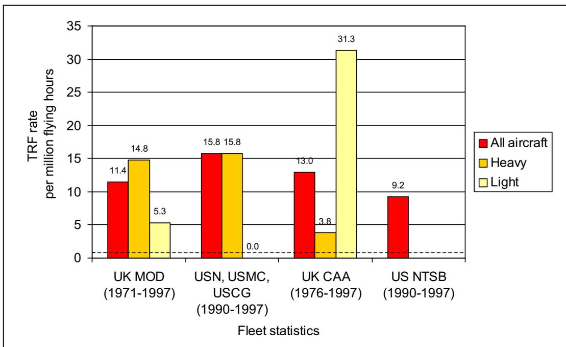
**Figure 2-4** TRF accident rates for UK and US fleets
