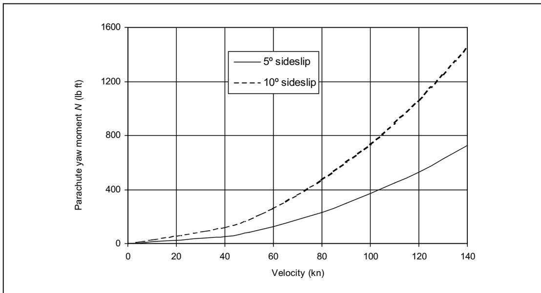
**Figure 5-5** Parachute restoring moment for a Lynx-sized aircraft
