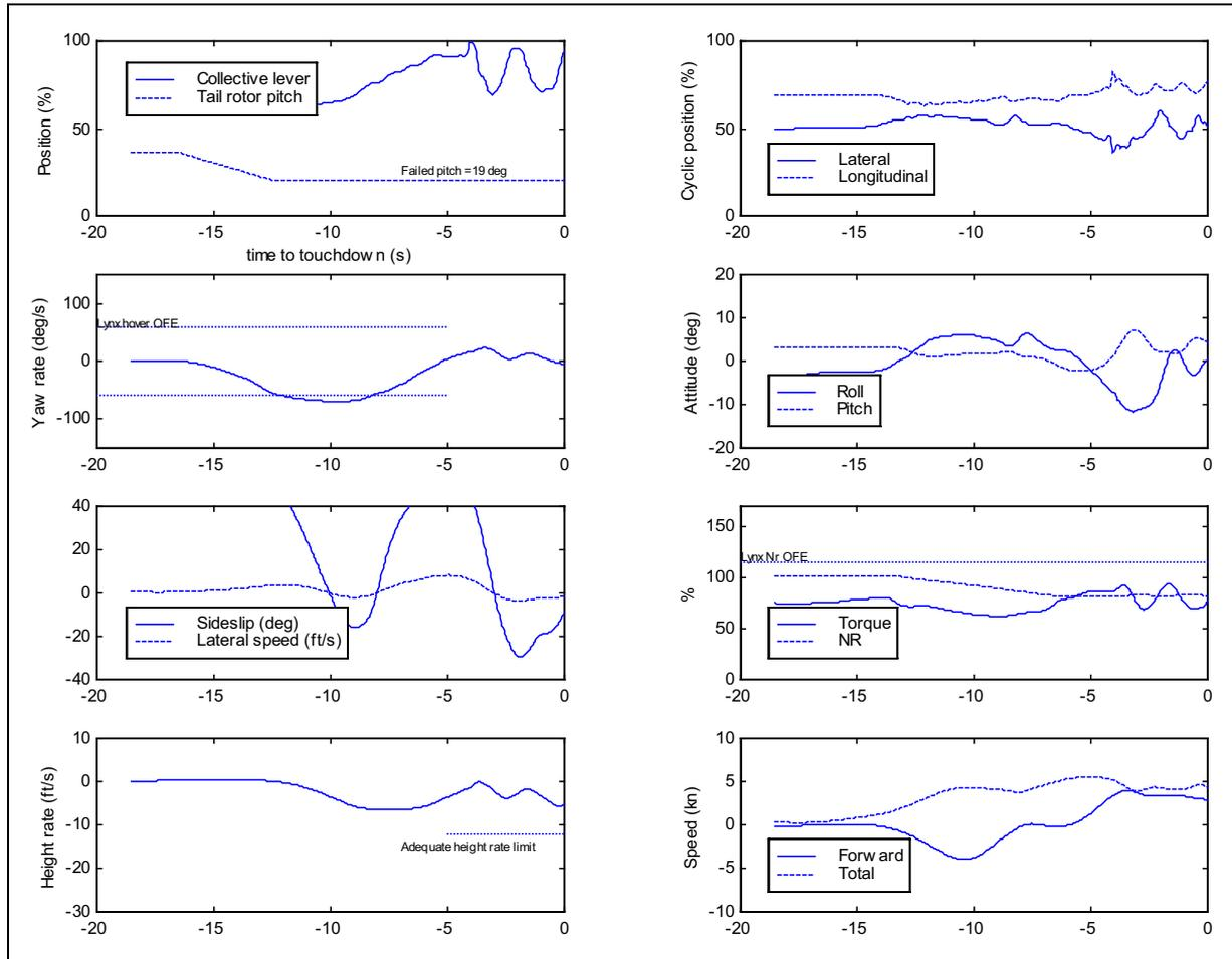
**Figure 6-48** Time histories for transient phase of HP TRCF in the hover (19x, P3, NR control, reduced weight)
