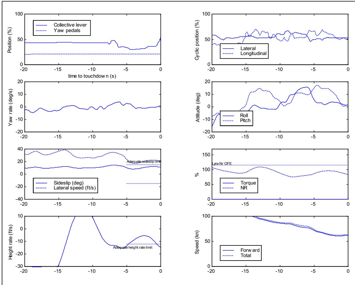
**Figure 6-29** Time histories for landing phase of TRDF at high speed (P2, deployable fin)
