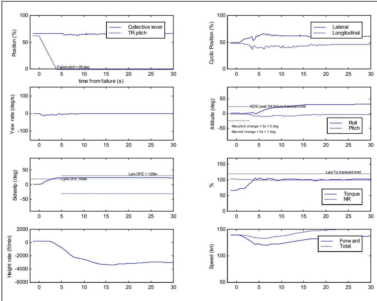
**Figure 6-14** Time histories for transient phase of HP TRCF at high speed (P1, MYR 2)
