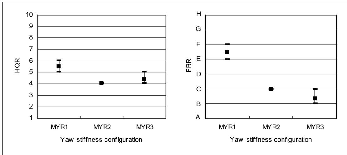
**Figure 6-19** Pilot ratings for transient phase of LP TRCF at mid speed
