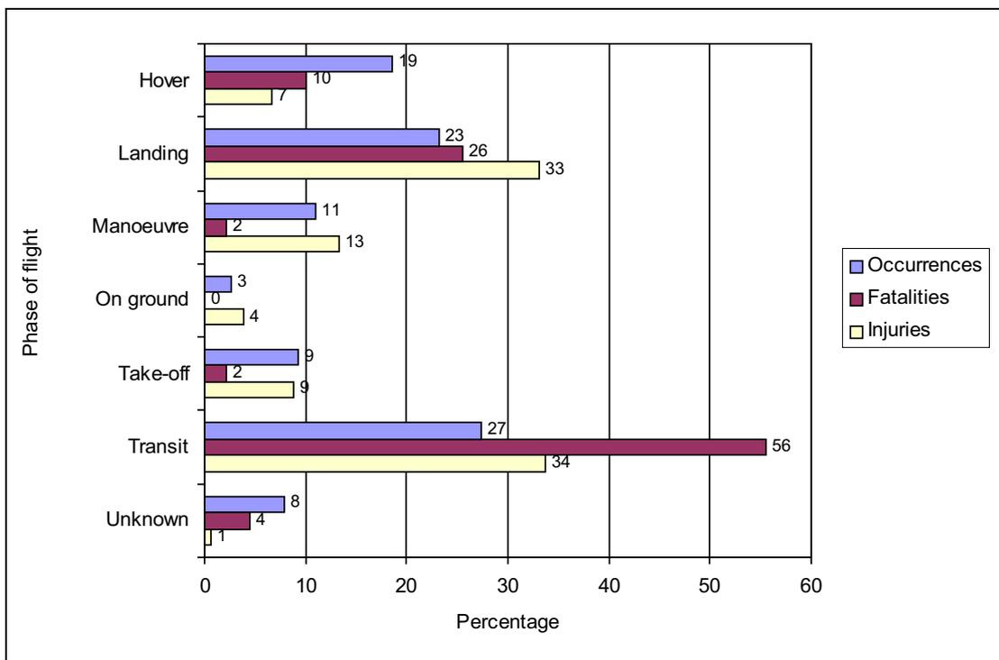
**Figure 2-9** Distribution of TRFs by phase of flight (all aircraft)
