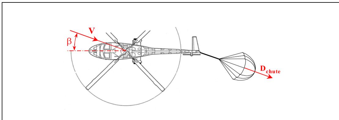
**Figure 5-4** Drag parachute operation
