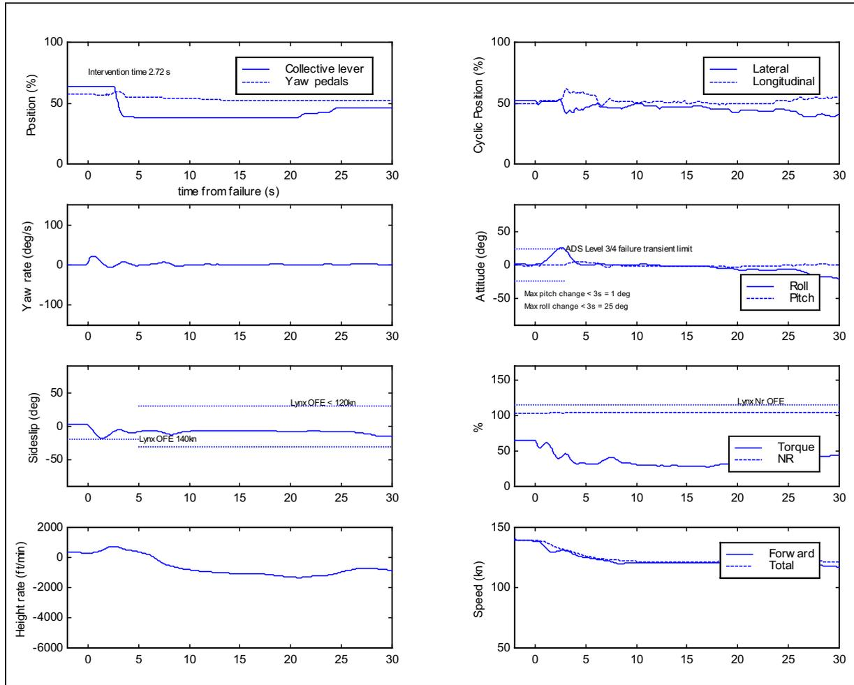
**Figure 6-26** Time histories for transient phase of TRDF at high speed (P2, enlarged fin)
