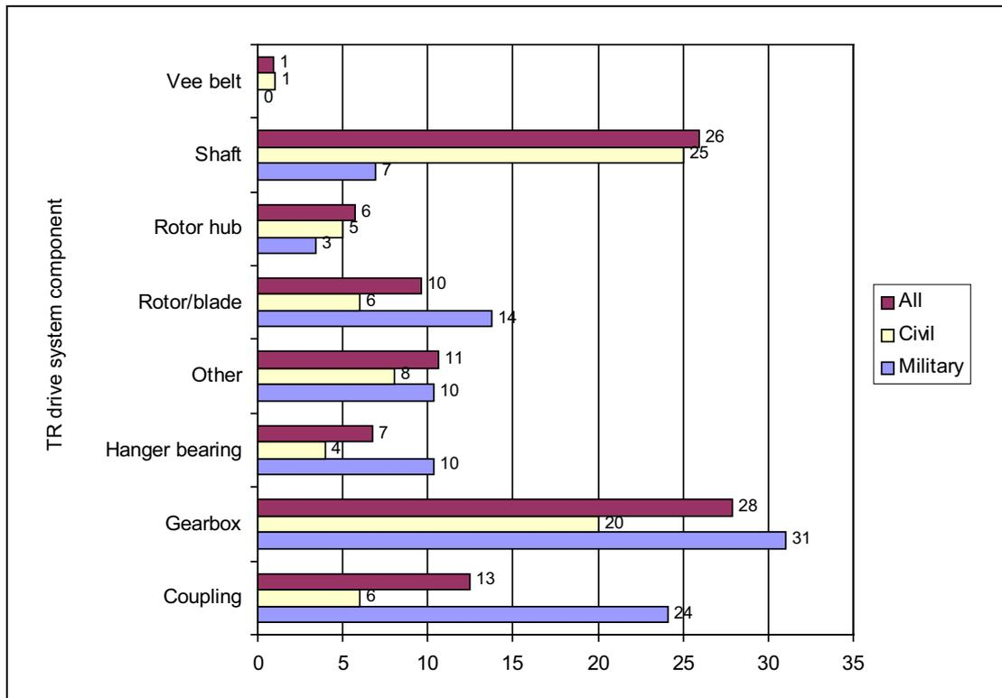
**Figure 2-6** Components of TR drive system causes of TRF (all aircraft)
