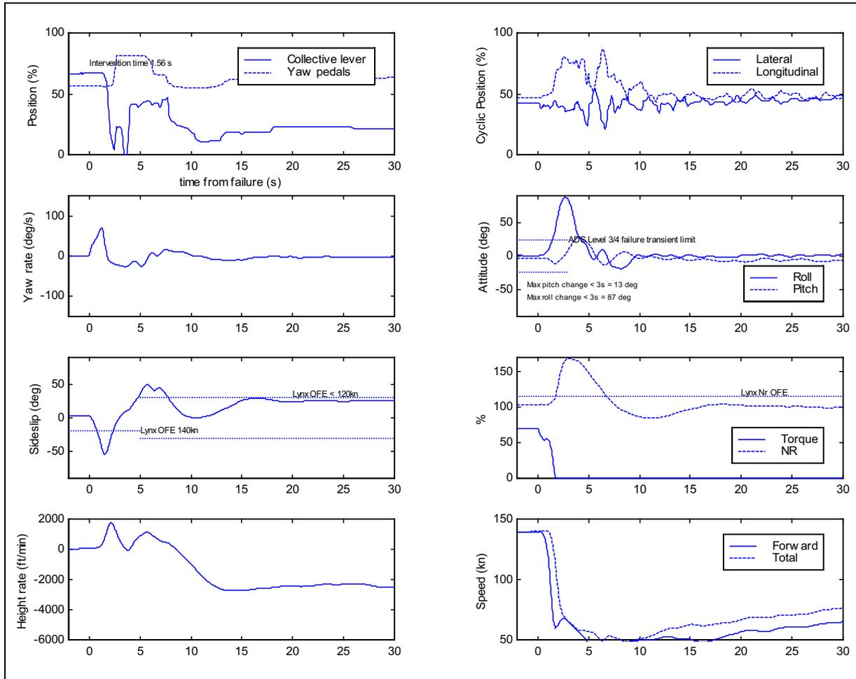
**Figure 6-25** Time histories for transient phase of TRDF at high speed (P3, articulated MR)
