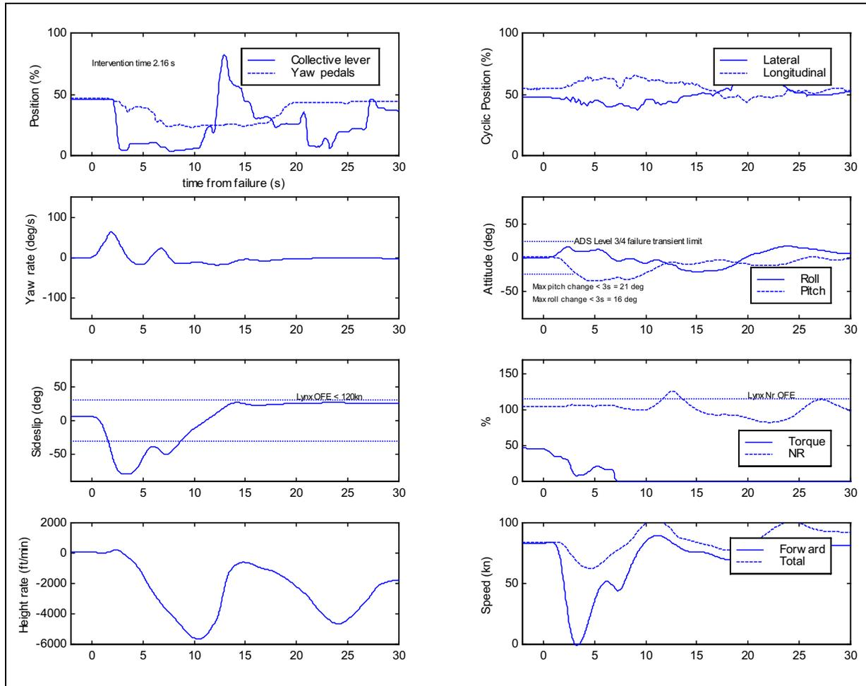
**Figure 6-39** Time histories for transient phase of TRDF at mid speed (P2, RC AFCS)
