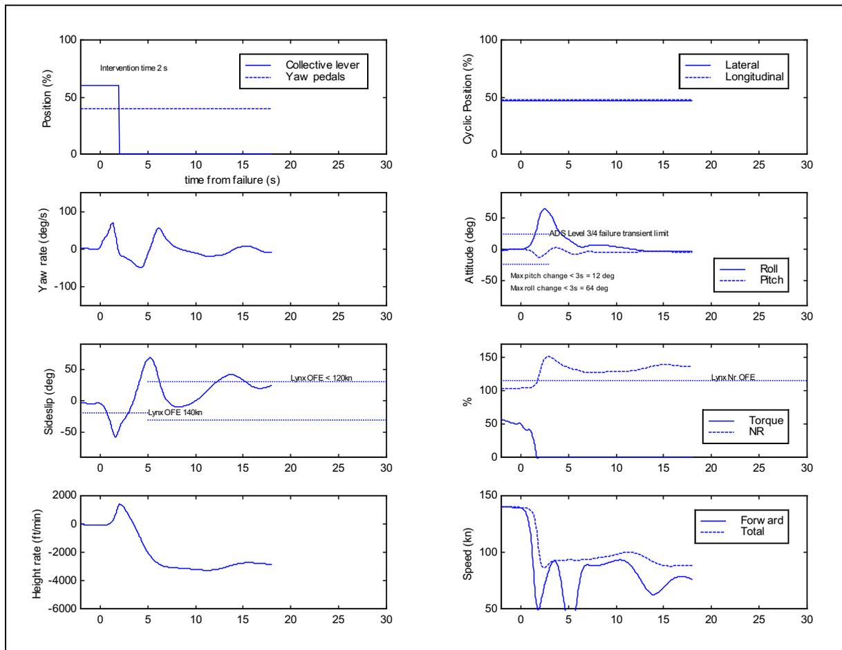
**Figure 2-2** Off-line simulation of 140 kn TRDF with 2 s PIT
