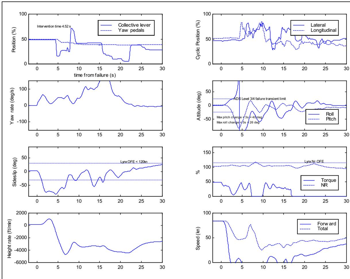
**Figure 6-40** Time histories for transient phase of TRDF at mid speed (P3, delayed reaction)
