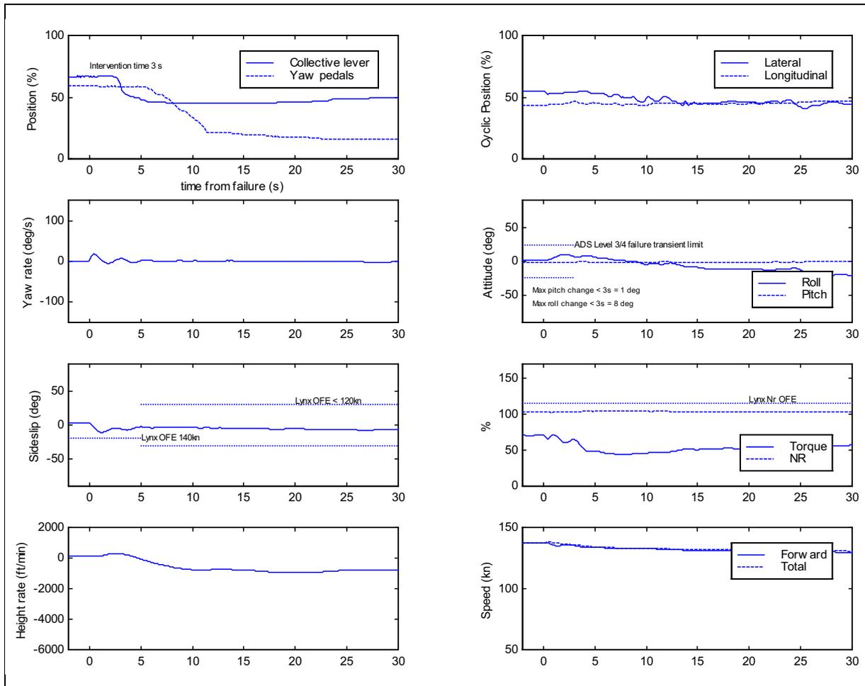
**Figure 6-5** Time histories for transient phase of TRDF at high speed (P2, MYR 3)
