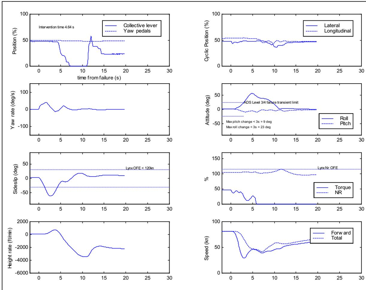
**Figure 6-41** Time histories for transient phase of TRDF at mid speed (P2, enlarged fin, delayed reaction)
