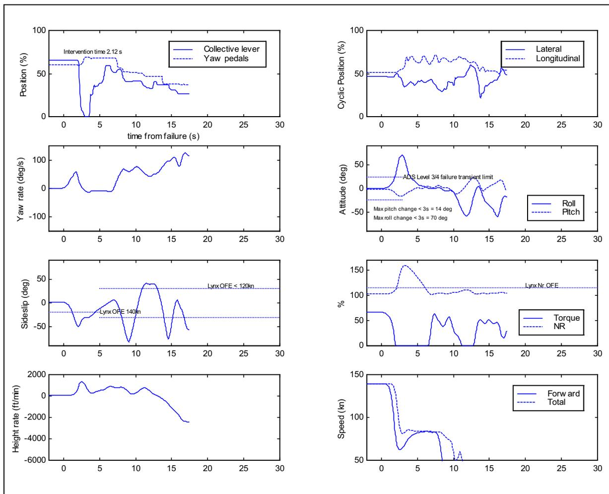
Figure 6-3 Time histories for transient phase of TRDF at high speed (P3, MYR 1)
