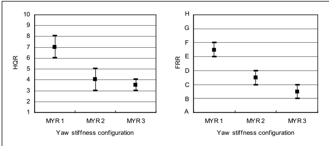
**Figure 6-8** Pilot ratings for manoeuvre phase of TRDF at mid speed
