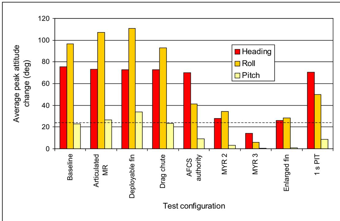
**Figure 6-34** Transient attitudes for TRDF at high speed
