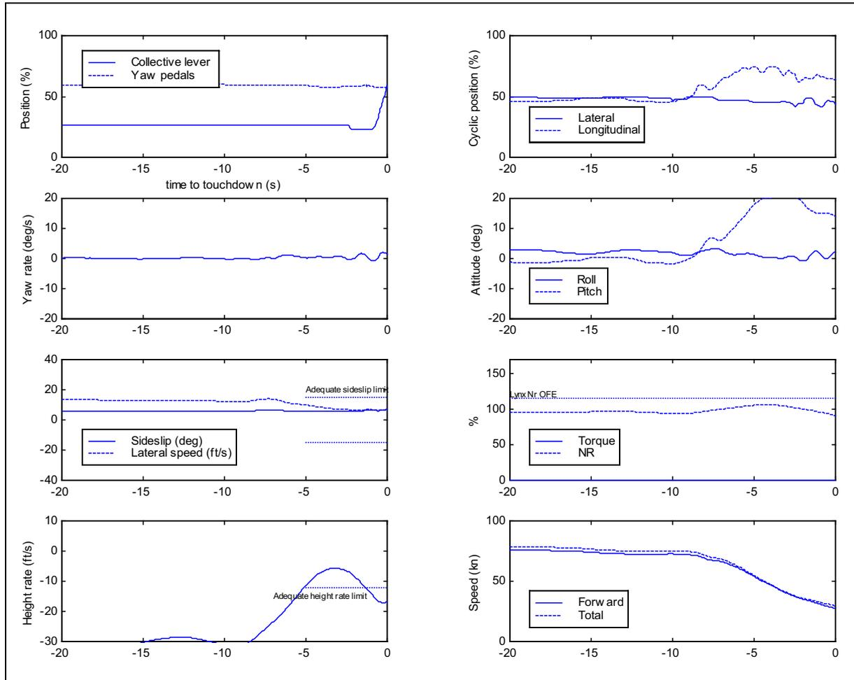
**Figure 6-31** Time histories for landing phase of TRDF at high speed (P3, drag chute)
