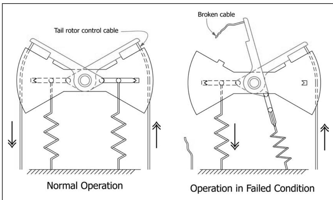
**Figure 5-1** TR redundant cable
