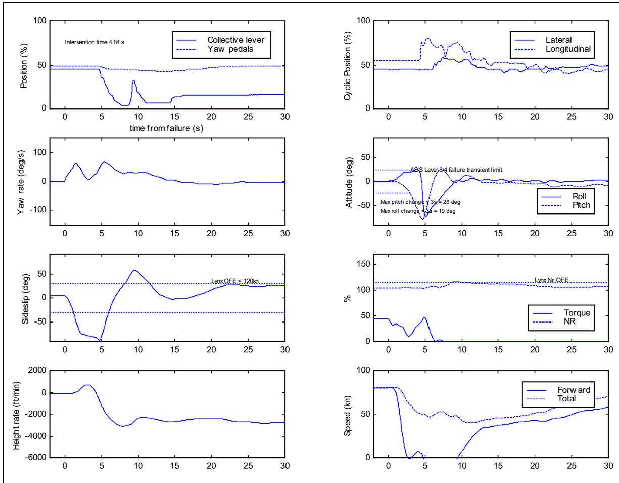
**Figure 6-44** Time histories for transient phase of TRDF at mid speed (P3, articulated MR, delayed reaction)
