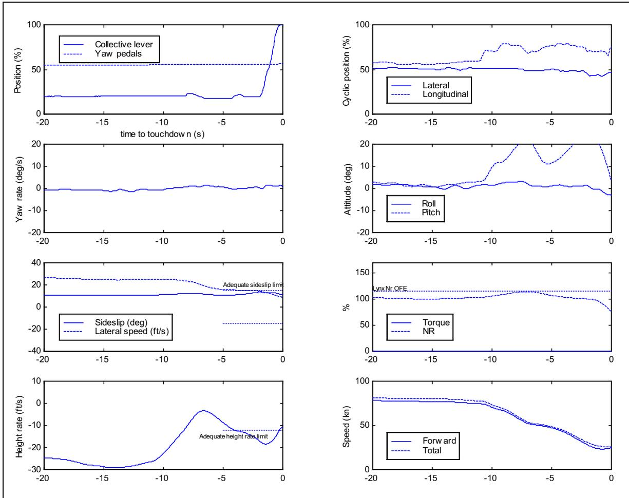
**Figure 6-27** Time histories for landing phase of TRDF at high speed (P3, enlarged fin)
