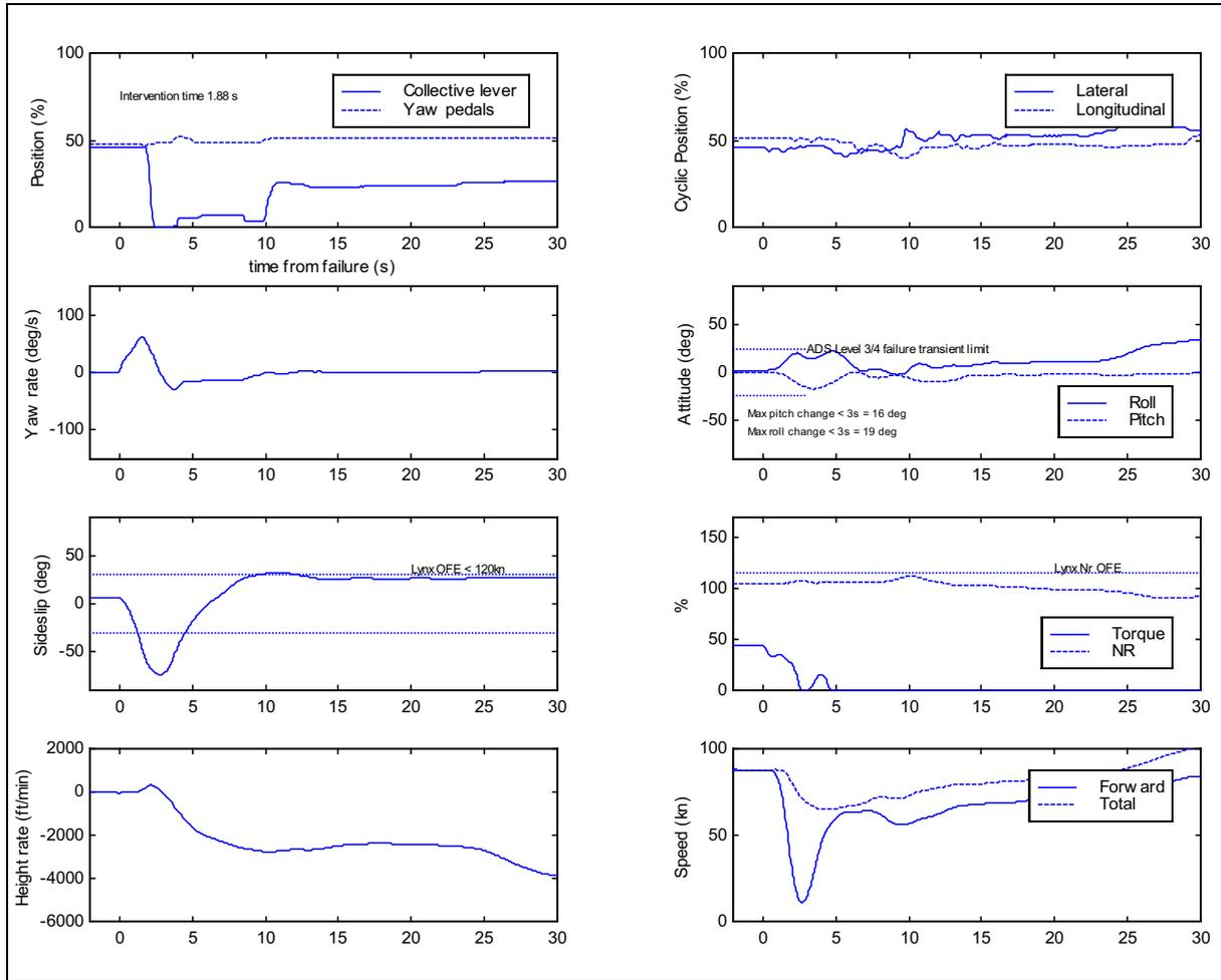
**Figure 6-42** Time histories for transient phase of TRDF at mid speed (P2, articulated MR)
