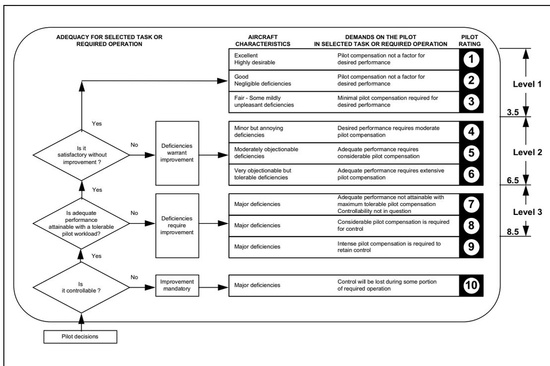
**Figure 3-1** Cooper-Harper HQR scale
