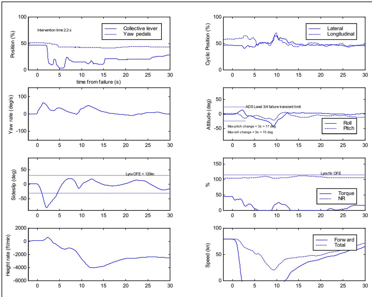
**Figure 6-38** Time histories for transient phase of TRDF at mid speed (P3, drag chute)
