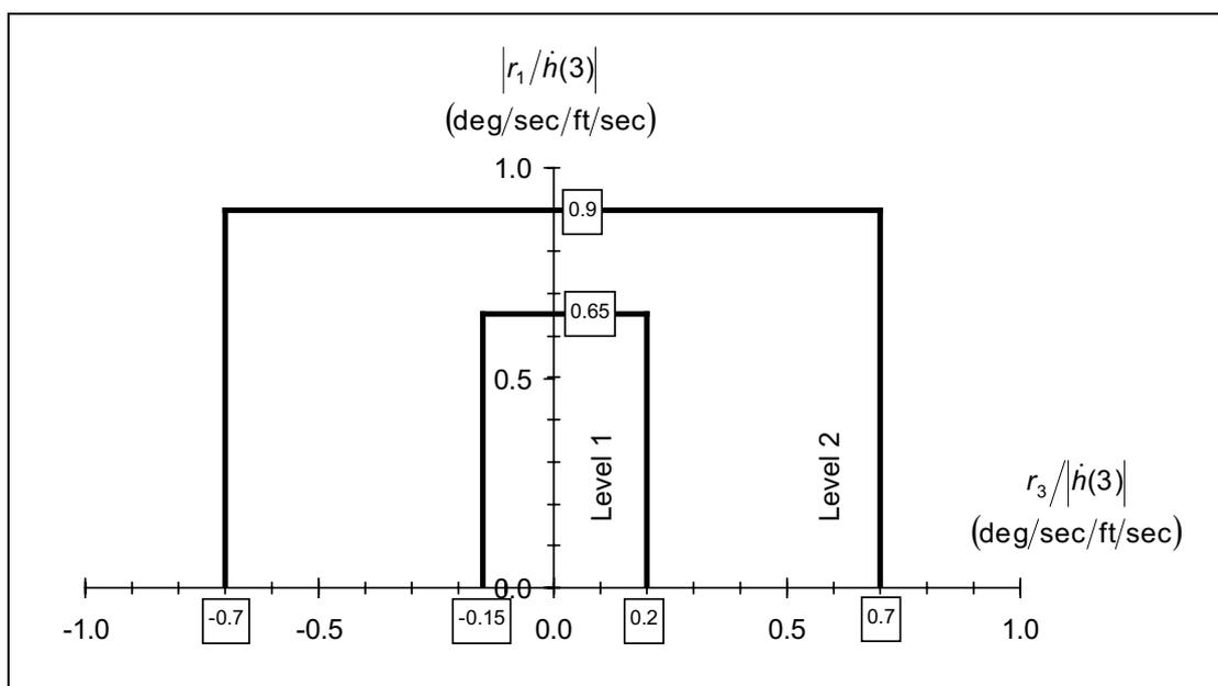
**Figure 3-2** ADS-33D collective to yaw coupling requirements
