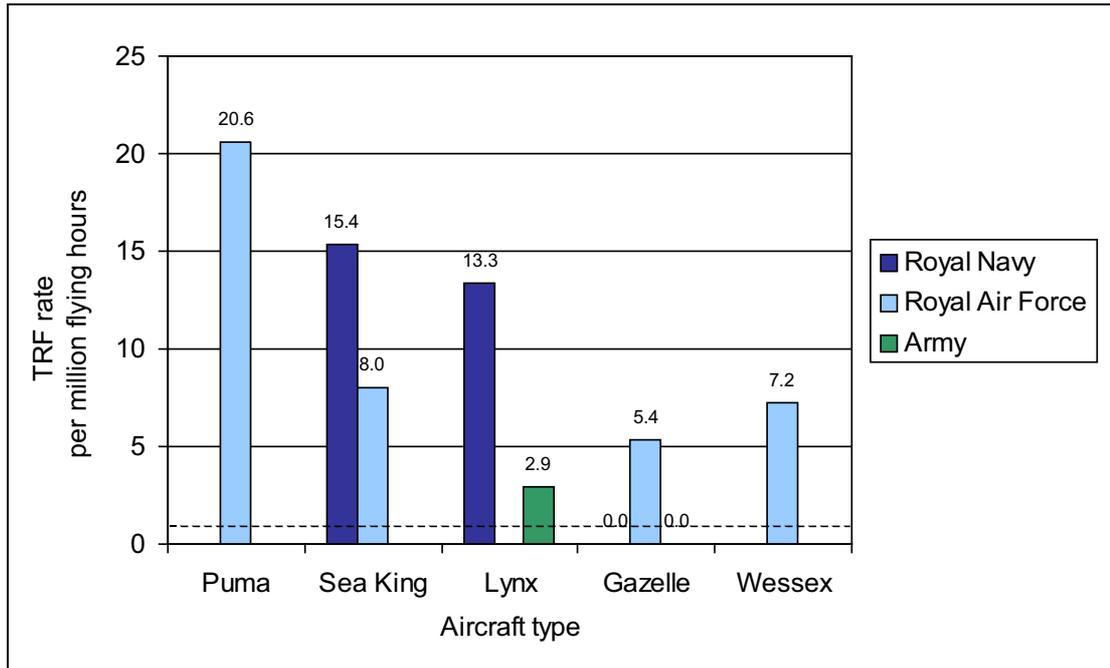
**Figure 2-3** TRAC UK MOD technical TRF occurrences by type
