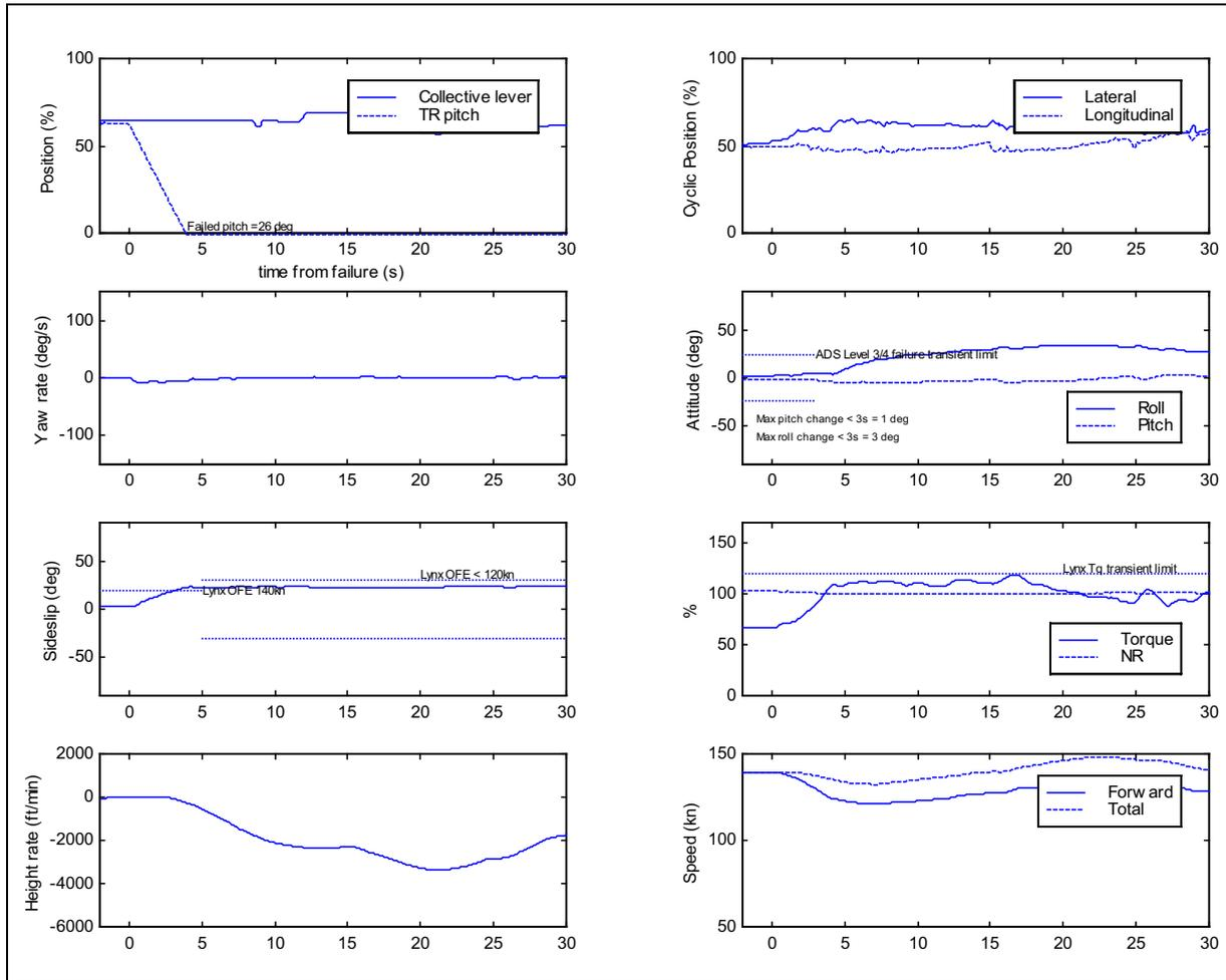
**Figure 6-15** Time histories for transient phase of HP TRCF at high speed (P1, MYR 3)
