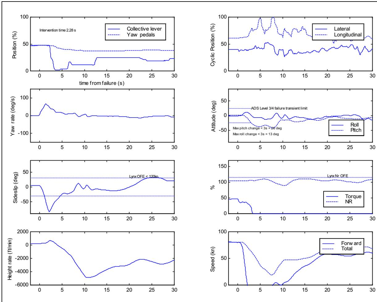
**Figure 6-43** Time histories for transient phase of TRDF at mid speed (P3, articulated MR, RC AFCS)
