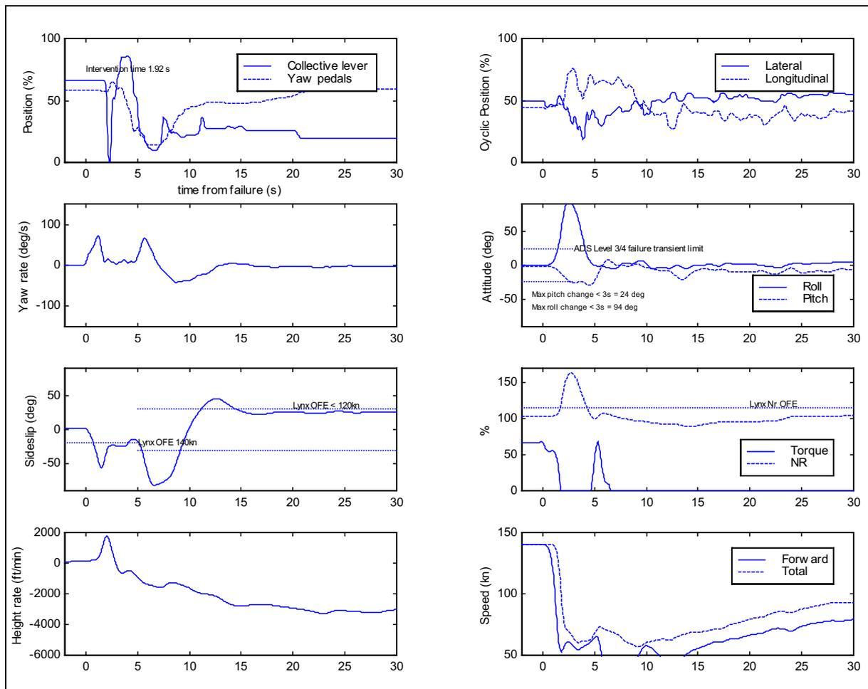
**Figure 6-23** Time histories for transient phase of TRDF at high speed (P3, baseline)
