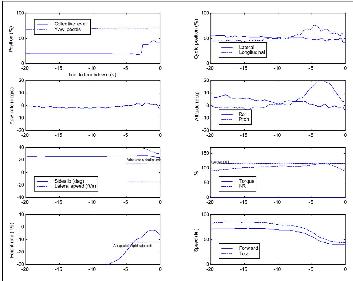
**Figure 6-24** Time histories for landing phase of TRDF at high speed (P3, baseline)
