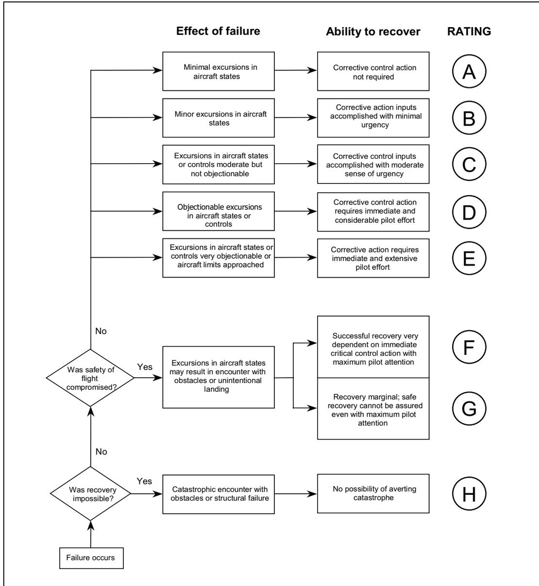
Figure 6-2 Failure/recovery rating scale
