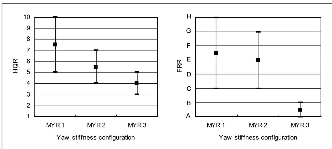
**Figure 6-9** Pilot ratings for landing phase of TRDF at mid speed
