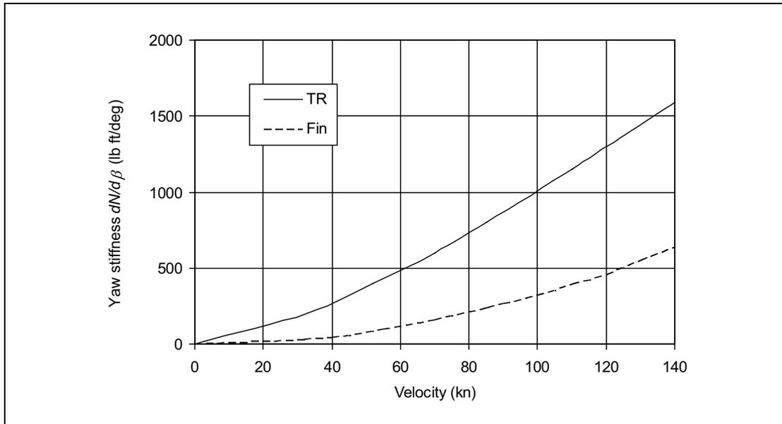
**Figure 5-2**  $dN/d\beta$  for a Lynx-sized aircraft
