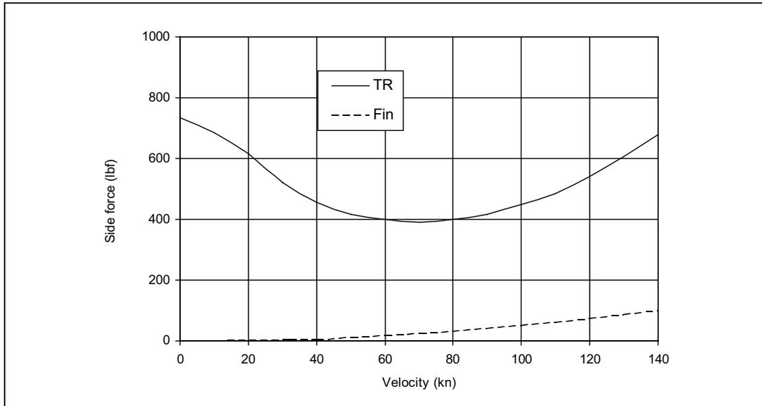
**Figure 5-3** Fin lift and net TR thrust requirement for Lynx-sized aircraft
