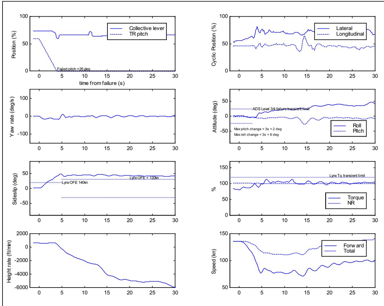
**Figure 6-13** Time histories for transient phase of HP TRCF at high speed (P2, MYR 1)
