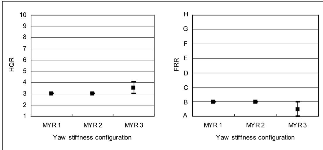
**Figure 6-22** Pilot ratings for landing phase of TP TRCF
