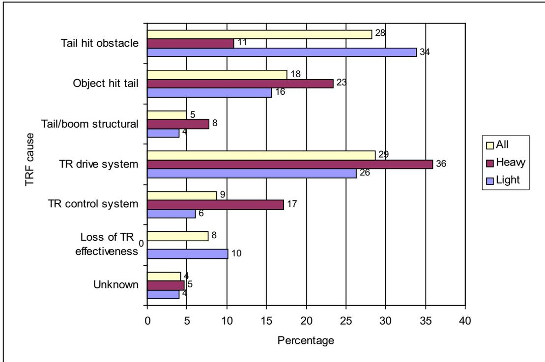
Figure 2-7 Distribution of TRF causes (civil aircraft)
