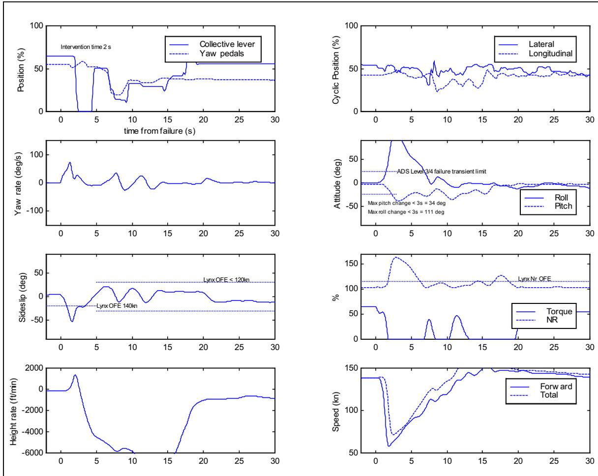
**Figure 6-28** Time histories for transient phase of TRDF at high speed (P2, deployable fin)
