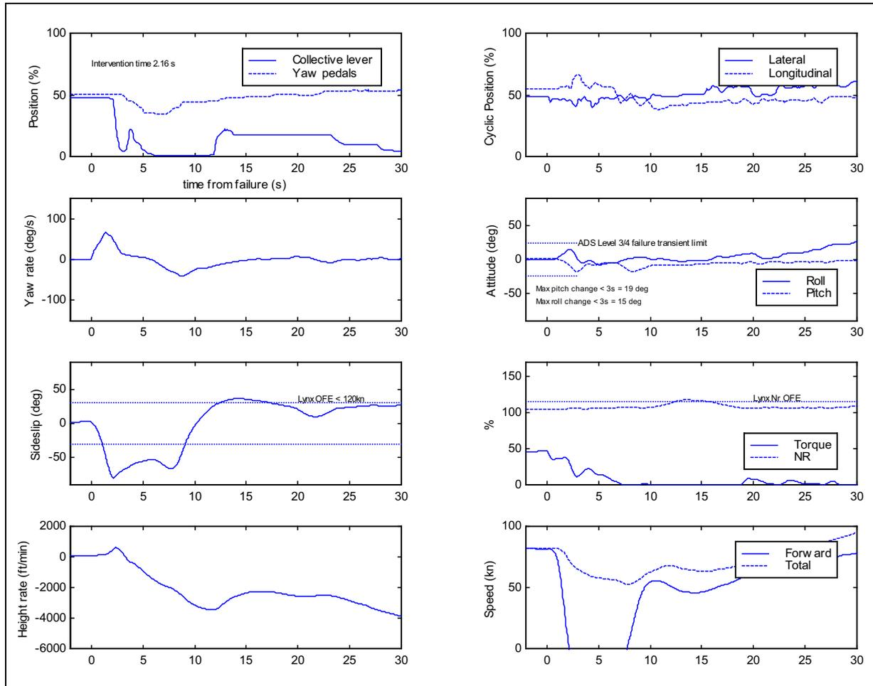
**Figure 6-37** Time histories for transient phase of TRDF at mid speed (P3, baseline)
