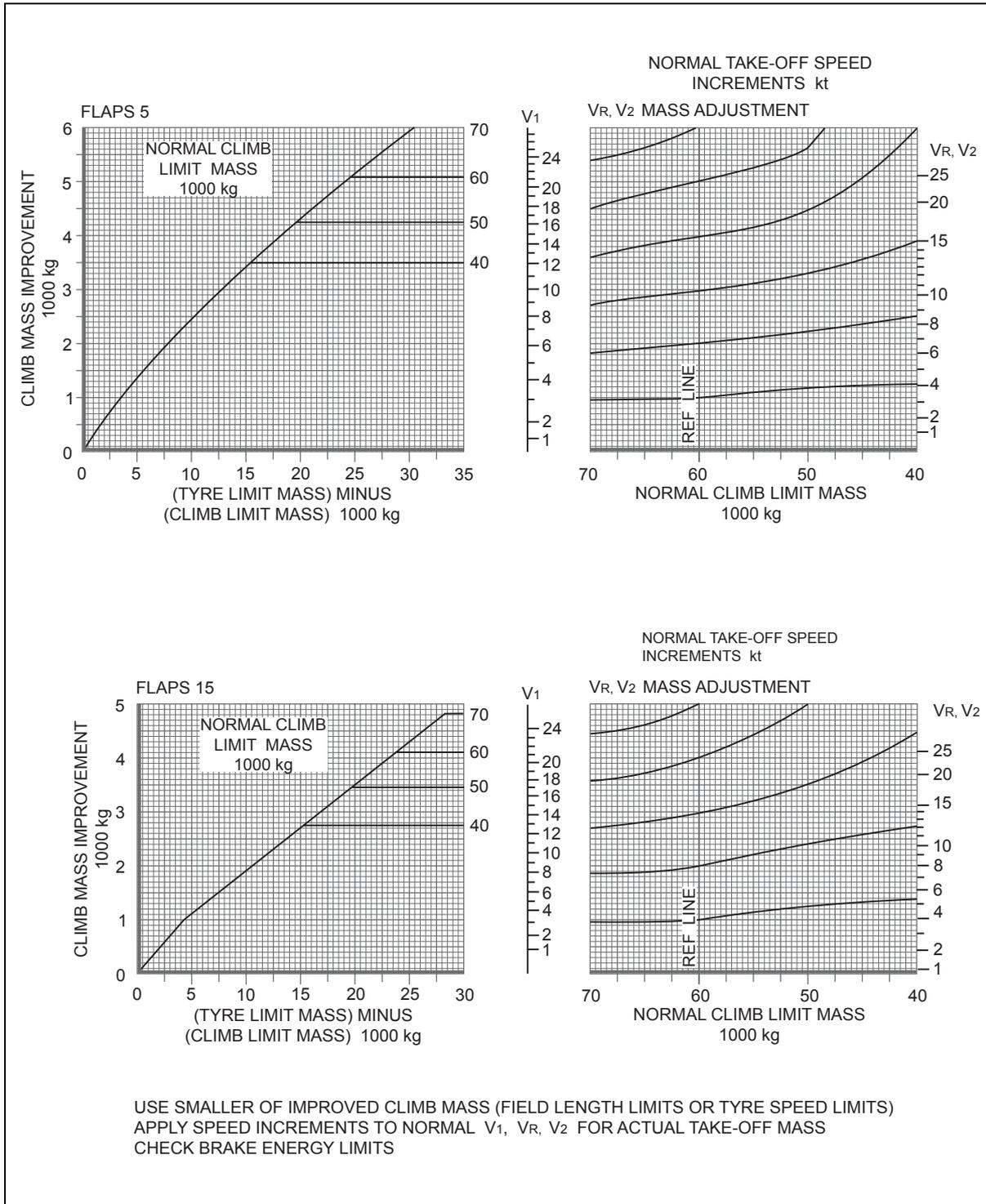
**Figure 4.16** Improved Climb Performance – Tyre Speed Limit
