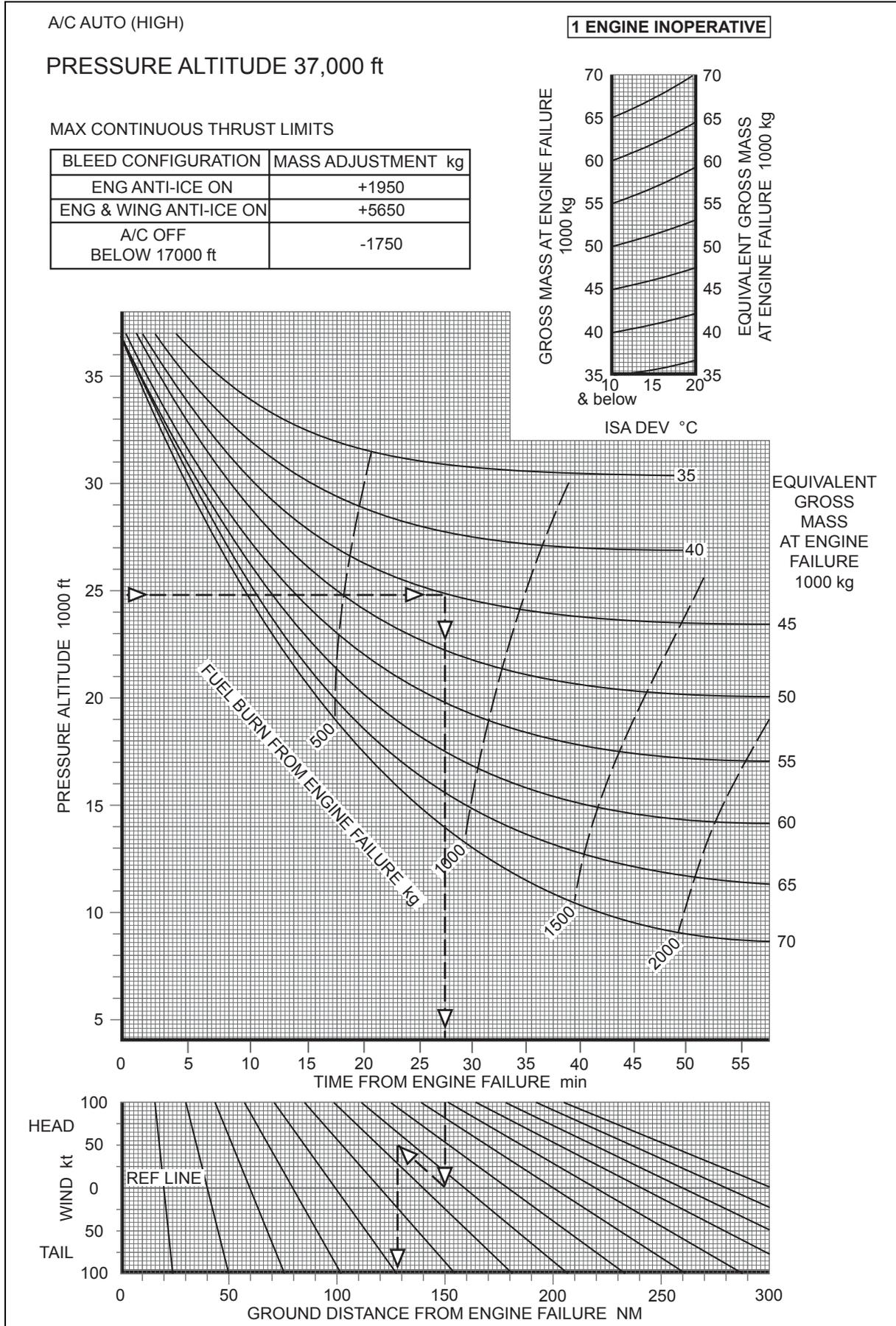
**Figure 4.24** Driftdown Profiles – Net Flight Path
