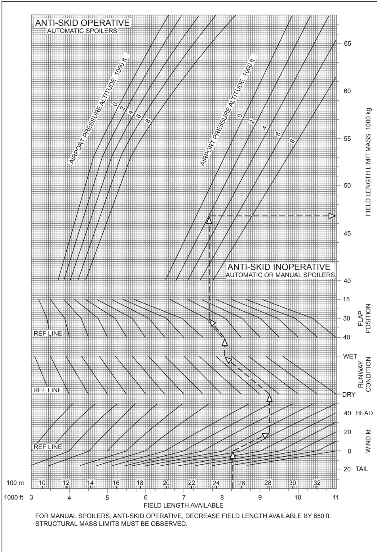
**Figure 4.28** Landing Performance – Field Length Limit
