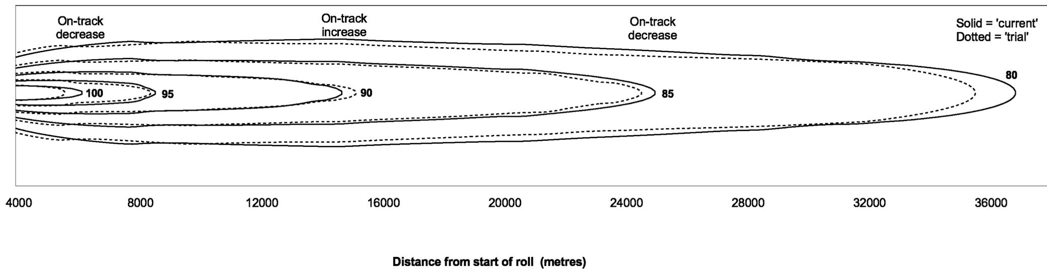
**Figure 3 - Boeing 747-100 Departures (at 93% MTOW): comparison of SEL footprints for IATA 'current' and 'trial' procedures (footprints corresponding to Figure 2)**
