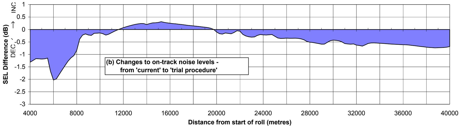
**Figure 2 - Boeing 747-100 departures (at 93% MTOW): effect of changing from 'current' to 'trial' procedure (IATA case)**
