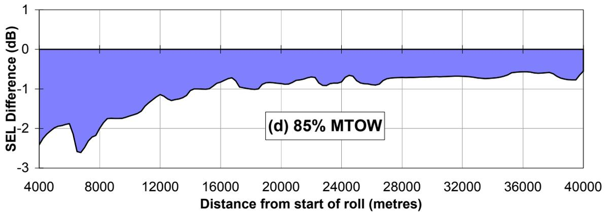
**Figure 6 - Boeing 747-100 departures using ICAO A procedure: effect of restoring take-off thrust from flexible to full**
