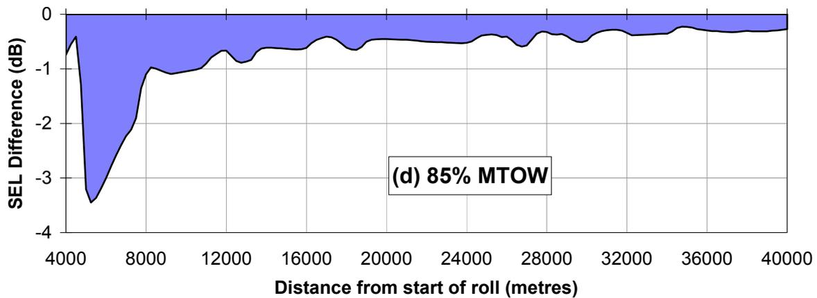
**Figure 10 - Chapter 3 Boeing 747-200 departures: effect of restoring full take-off thrust and lowering cutback height from 1500 ft to 1000 ft**
