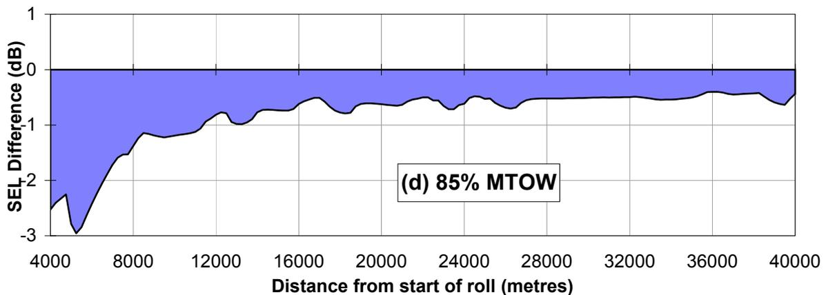
**Figure 8 - Boeing 747-100 departures: effect of restoring full take-off thrust and lowering cutback height from 1500 ft to 1000 ft**
