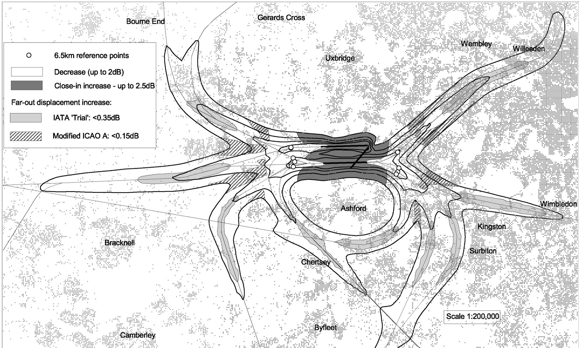
**Figure 16 - B747-100 departures from Heathrow: relative Leq contours for IATA 'current' operating procedure. Contours are at 5 dB intervals. Leq changes caused by altering operating procedure are indicated by shading (IATA 'trial') and hatching (Modified ICAO A). Base map shows runways, nominal flight tracks and population pattern.**
