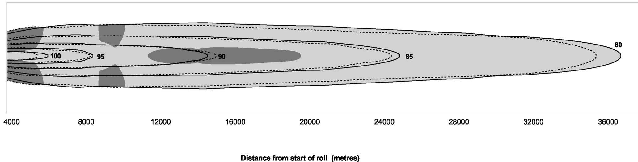
**Figure 15 - Boeing 747-100 departures: comparison of SEL footprints (in increasing 5 dB steps starting at 80 dBA) for IATA 'current' (unbroken) and 'trial' (dashed) procedures - dark shading shows where SEL is increased under 'trial' procedure, light shading shows where SEL is decreased.**
