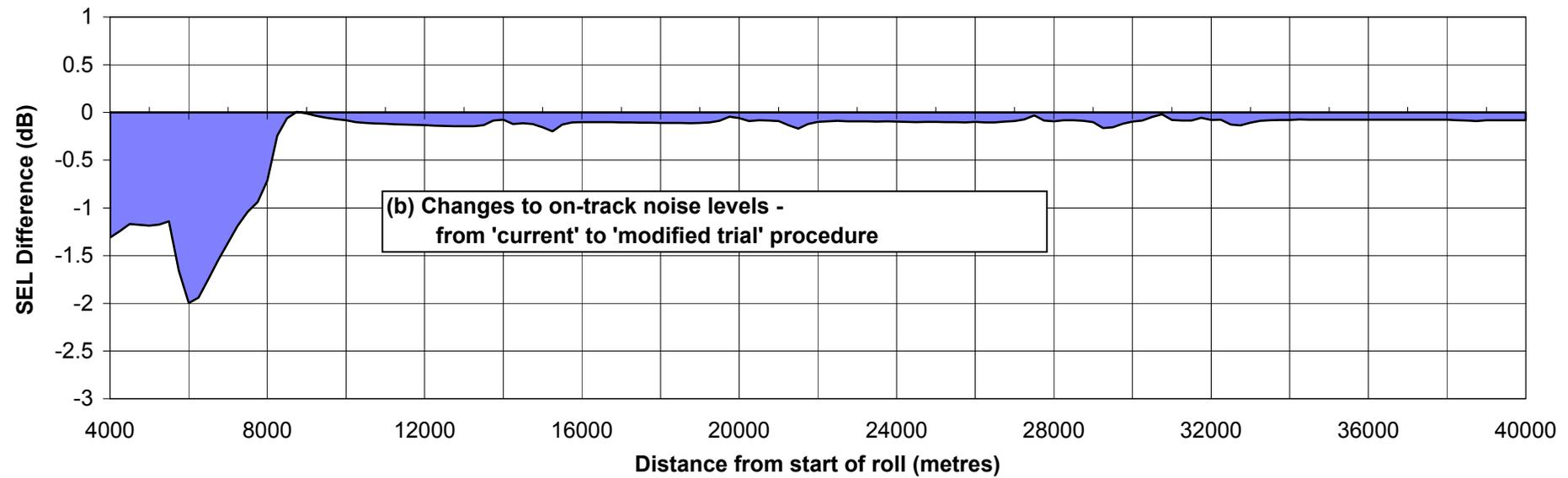
**Figure 5 - Boeing 747-100 departures at 93% MTOW: effect of changing from 'current' to 'modified trial' procedure**
