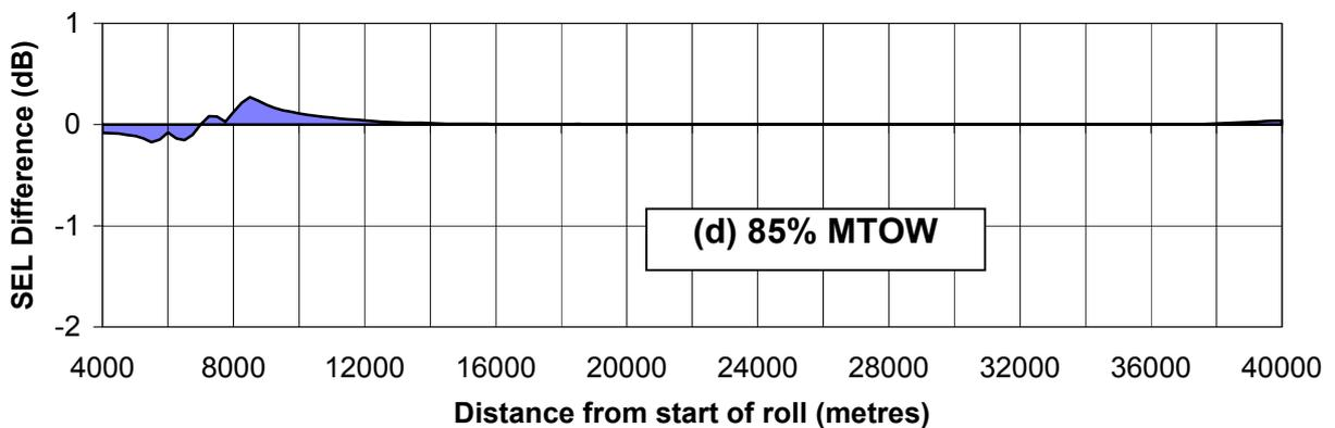
**Figure 1 - Boeing 747-100 departures using flexible take-off thrust: effect of lowering cutback height from 1500 ft to 1000 ft (as a single measure) on on-track noise levels. (Cutback thrust = maximum climb thrust)**
