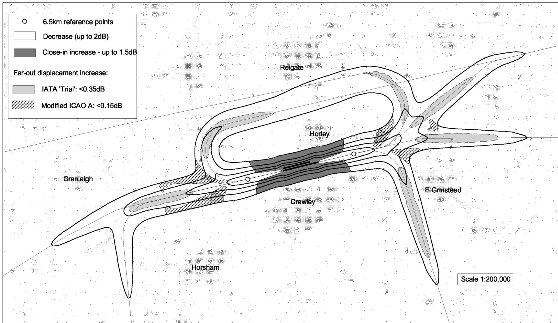
**Figure 17 - B747-100 departures from Gatwick: relative Leq contours for IATA 'current' operating procedure. Contours are at 5 dB intervals. Leq changes caused by altering operating procedure are indicated by shading (IATA 'trial') and hatching (Modified ICAO A). Base map shows runways, nominal flight tracks and population pattern.**
