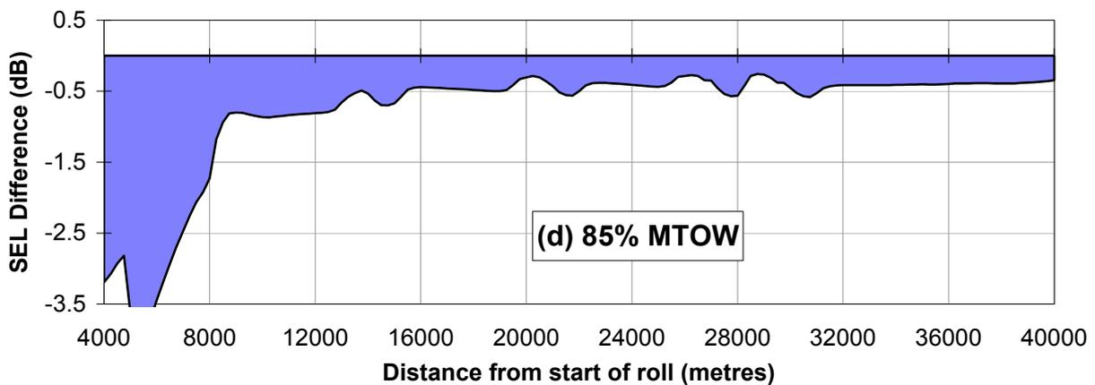
**Figure 9 - Chapter 2 Boeing 747-200 departures: effect of restoring full take-off thrust and lowering cutback height from 1500 ft to 1000 ft**
