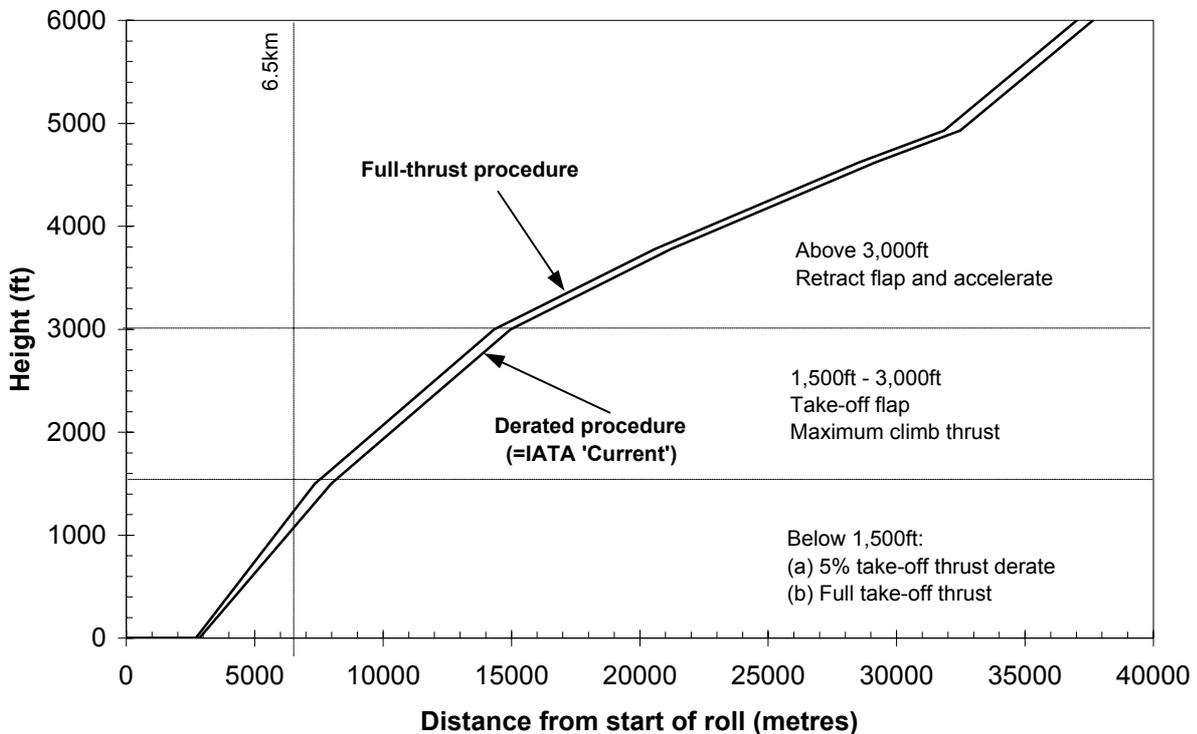
(b) 'Current procedure' - comparison of full and derated take-off thrust
