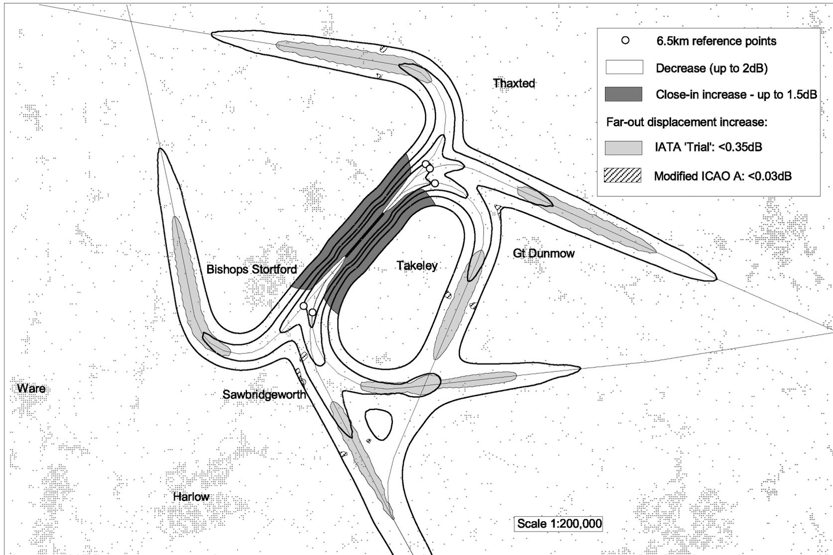
**Figure 18 - B747-100 departures from Stansted: relative Leq contours for IATA 'current' operating procedure. Contours are at 5dB intervals. Leq changes caused by altering operating procedure are indicated by shading (IATA 'trial') and hatching (Modified ICAO A). Base map shows runways, nominal flight tracks and population pattern.**
