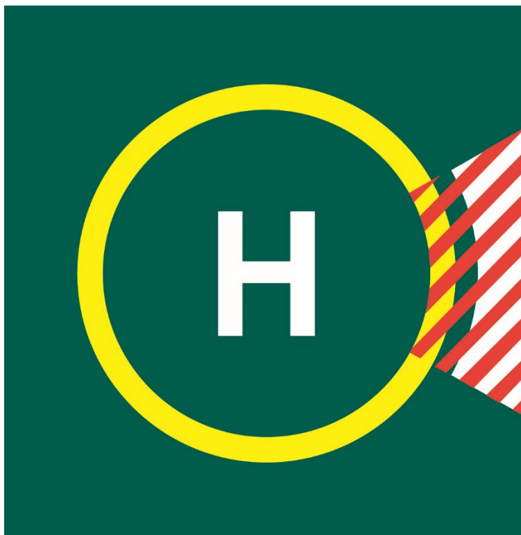
Figure 6: Example of prohibited landing heading marking
