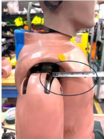
Figure 4 - Hybrid II Marker Positioning on the ATD Shoulder
