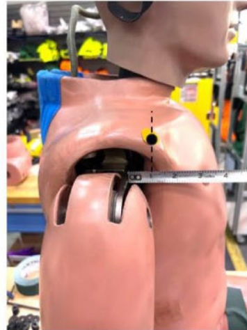
Figure 4 - Hybrid II Marker Positioning on the ATD Shoulder
