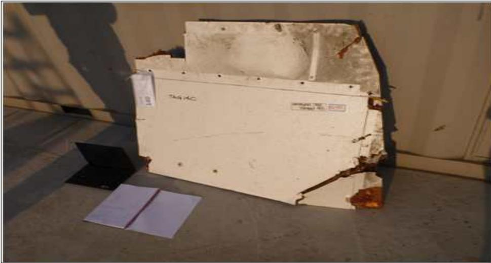
[Figure 37] Upper Deck Interior Panel with the Area of Sooting
