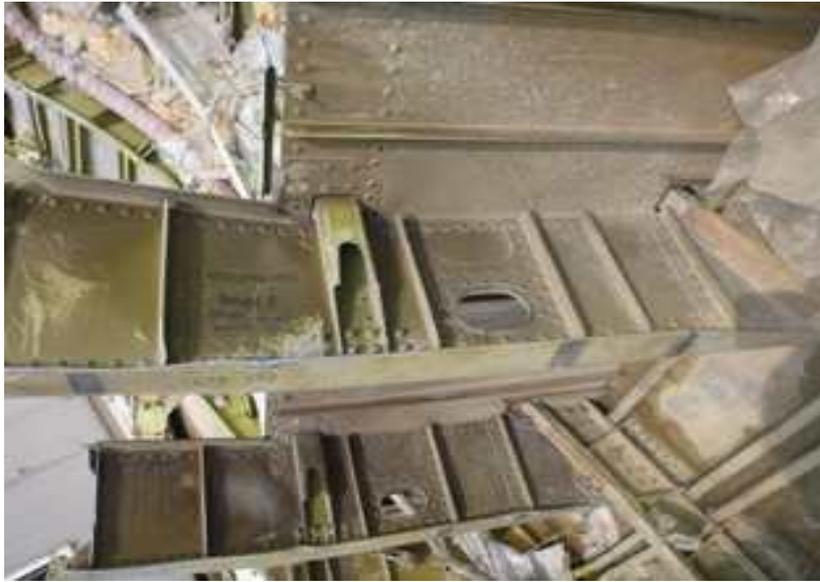
[Figure 43] Upper Deck Floor Beam at FS520
