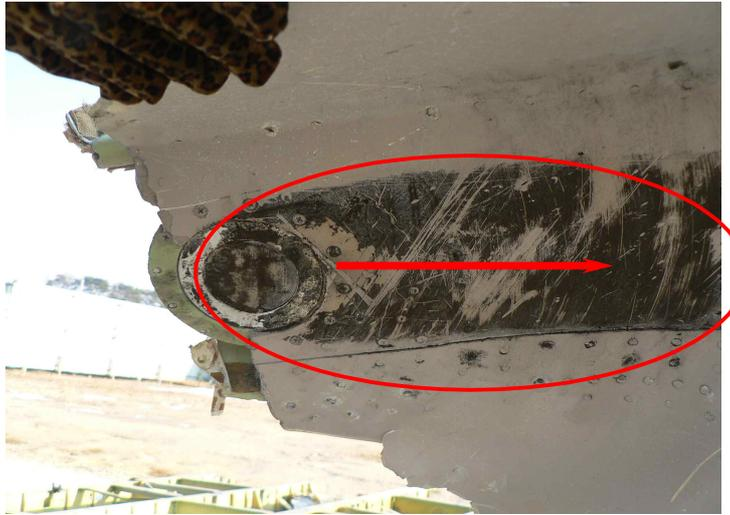
[Figure 19] Sooting on the Exterior Skin of Cockpit Smoke Evacuation Shutter
