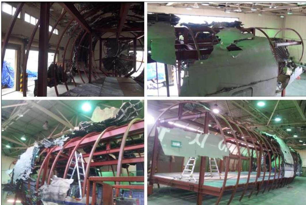
[Figure 45] Wreckage Reconstruction
