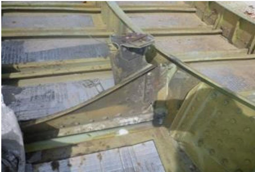
[Figure 44] Farthest Forward Evidence of Thermal Damage at FS580
