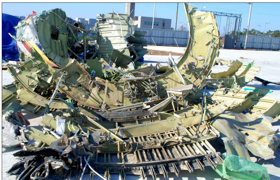
[Figure 29] Section 48 of the Aft Fuselage
