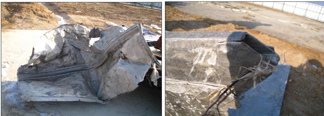
[Figure 38] Inside (Left) & Outside (Right) of the ULD Container
