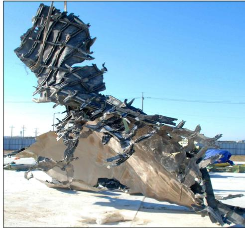
[Figure 26] Fire Damage to the Skin Between FS2180 & FS2360
