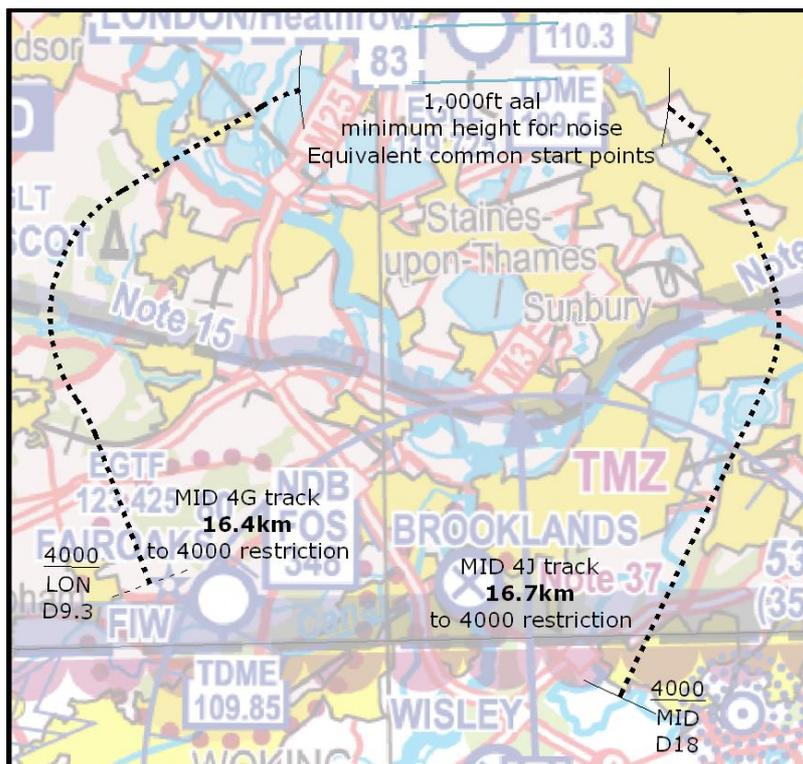
**Figure 6 Equivalent track lengths to 4,000ft**
