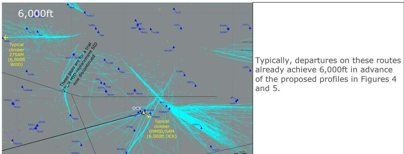
**Figure 7 Heathrow departures radar data samples 4,000ft/5,000ft/6,000ft**
