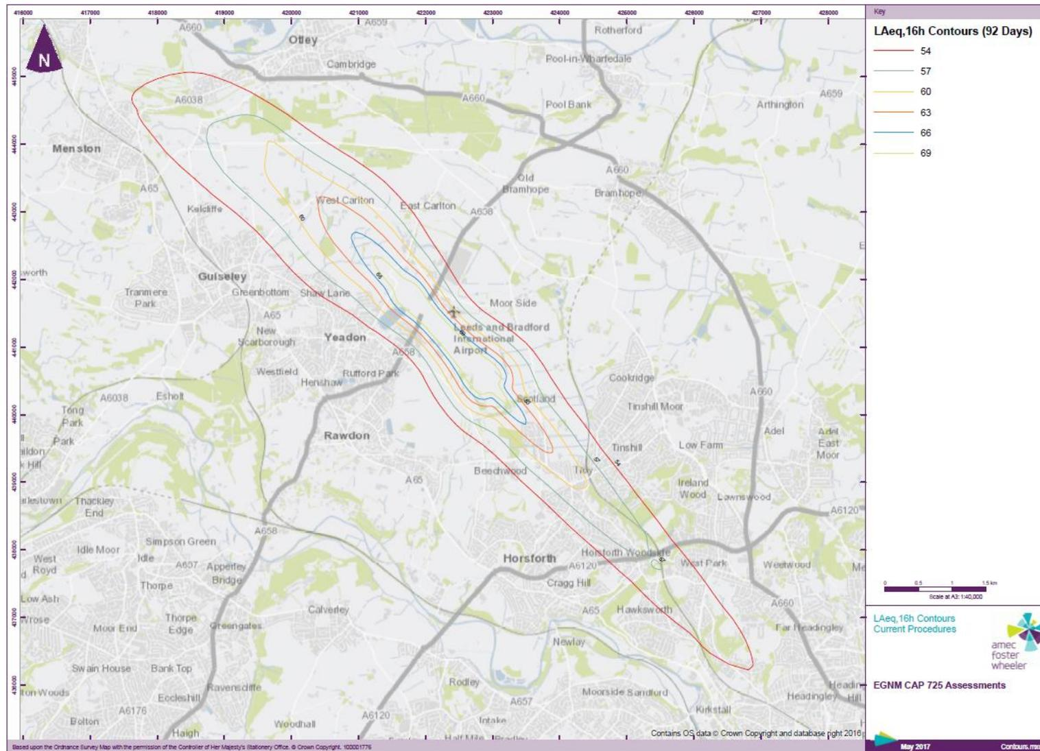
Figure 12 - Noise Contours for Existing Traffic Levels.
