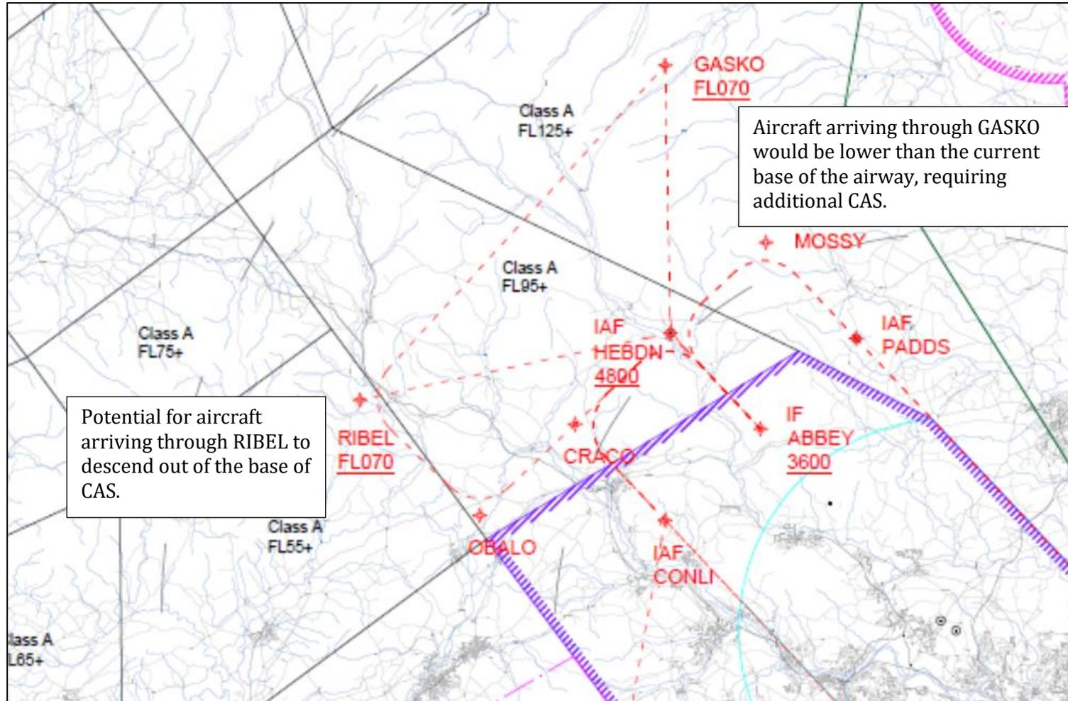
Figure 3. Design Iteration for Arrivals Direct from GASKO Inbound to Runway 14
