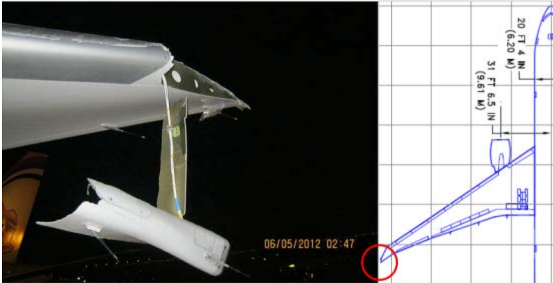
Figure 3 B777 LH Wingtip Damage
