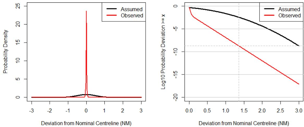
Figure 2: Comparison of assumed Gaussian distribution versus observed double-exponential distribution.
