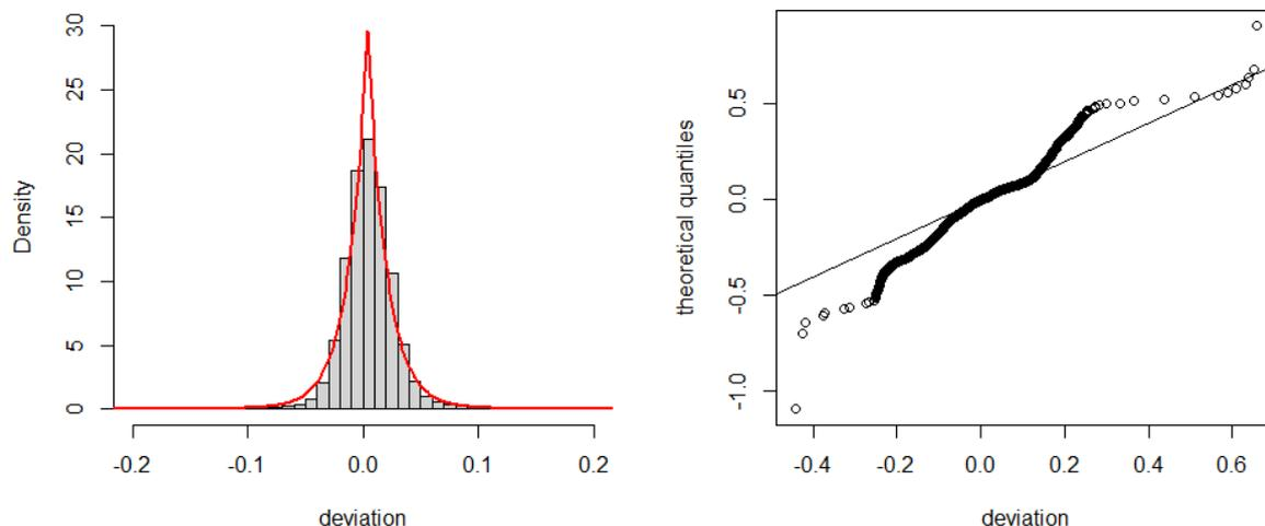
Figure 1: RNAV1 straight leg deviation data (histogram) with fitted distribution (red line); quantile-quantile plot showing conservatism of fitted distribution in the tails.
