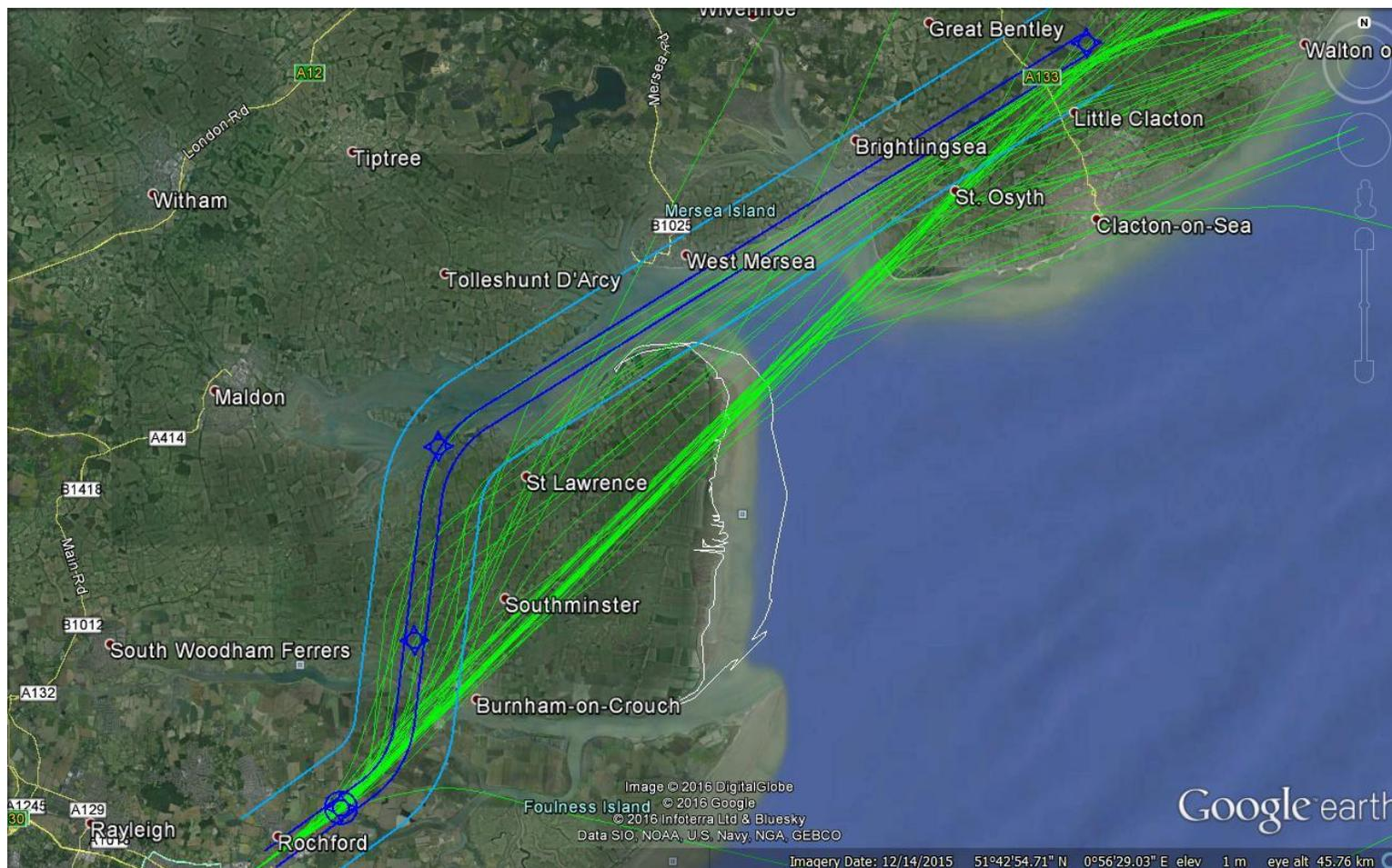
Diagram showing the anticipated maximum track dispersion ( $\pm 0.2\text{NM}$ ; dark blue) and the maximum navigation tolerance ( $\pm 1.0\text{NM}$ ; light blue) for the CLN 1G SID against historic NTK tracks (green) for departing aircraft July/August 2015.
