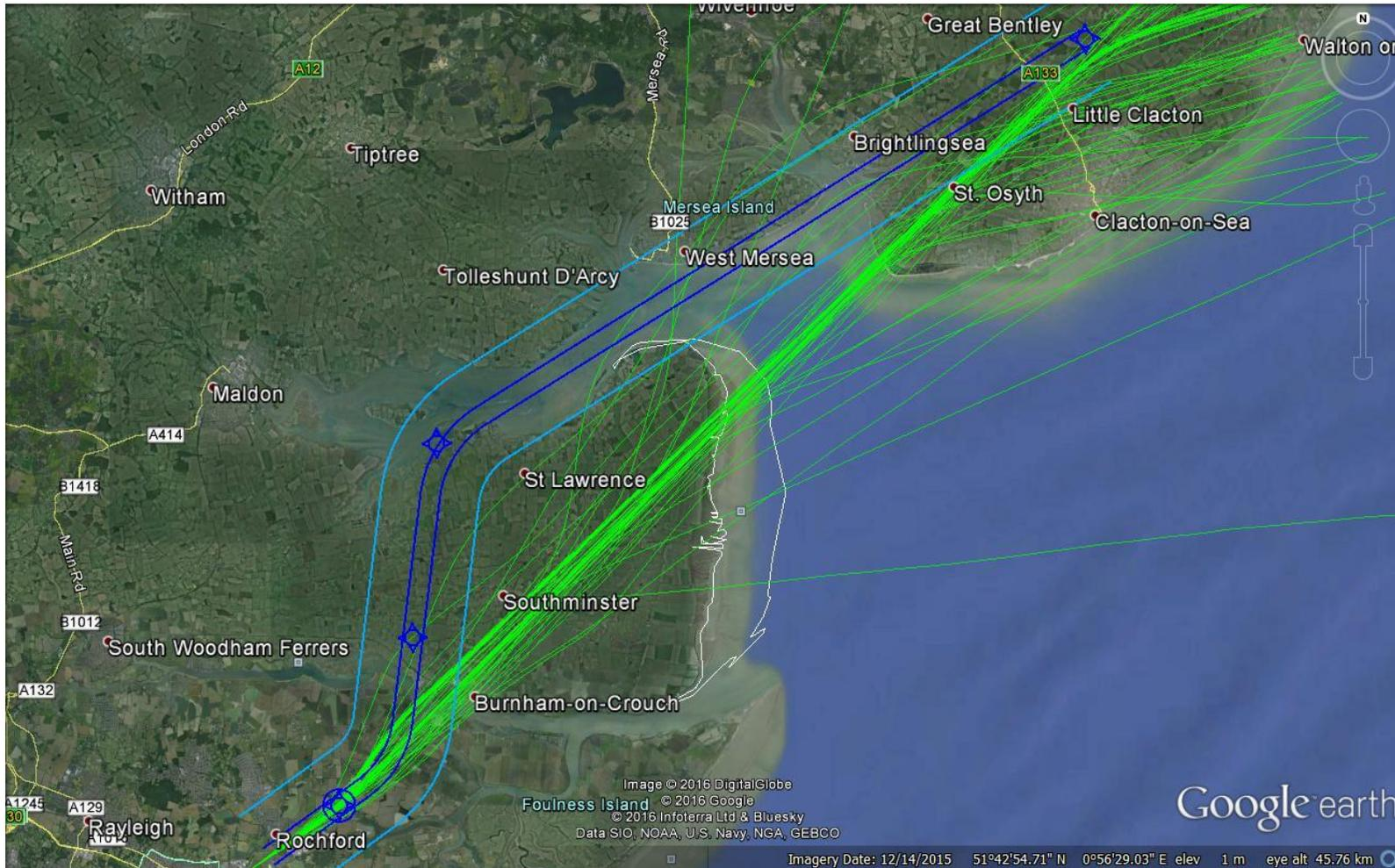
Diagram showing the anticipated maximum track dispersion ( $\pm 0.2\text{NM}$ ; dark blue) and the maximum navigation tolerance ( $\pm 1.0\text{NM}$ ; light blue) for the CLN 1G SID against historic NTK tracks (green) for departing aircraft July/August 2014.
