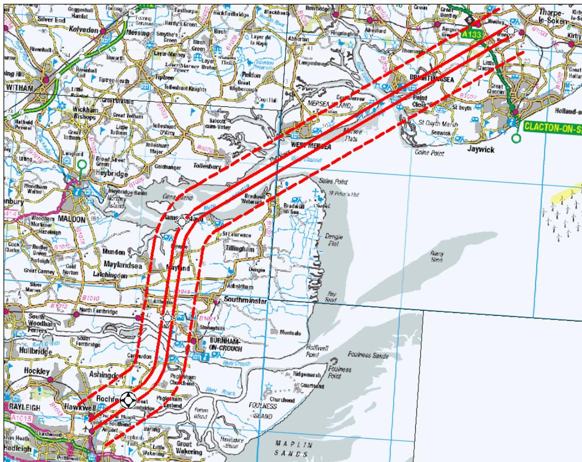
**CLN 1G SID:** Diagram showing the anticipated maximum track dispersion ( $\pm 0.2\text{NM}$ ; solid red lines) and the maximum navigation tolerance ( $\pm 1.0\text{NM}$ ; dashed red lines) overlaid on Ordnance Survey map.
