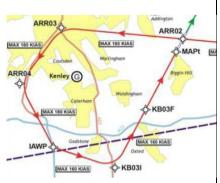
Following this, all future designs of the Runway 03 procedure incorporated a 30° turn at the Final Approach Fix (FAF) KB03F, which allowed the nominal track (but not the entirety of the protection on 8 Jan 2018 ftp://rms.ftp@37.1.99.153/D oc 8 - Comments on the Report issued by the CAA on 8 Jan 2018.pdf
