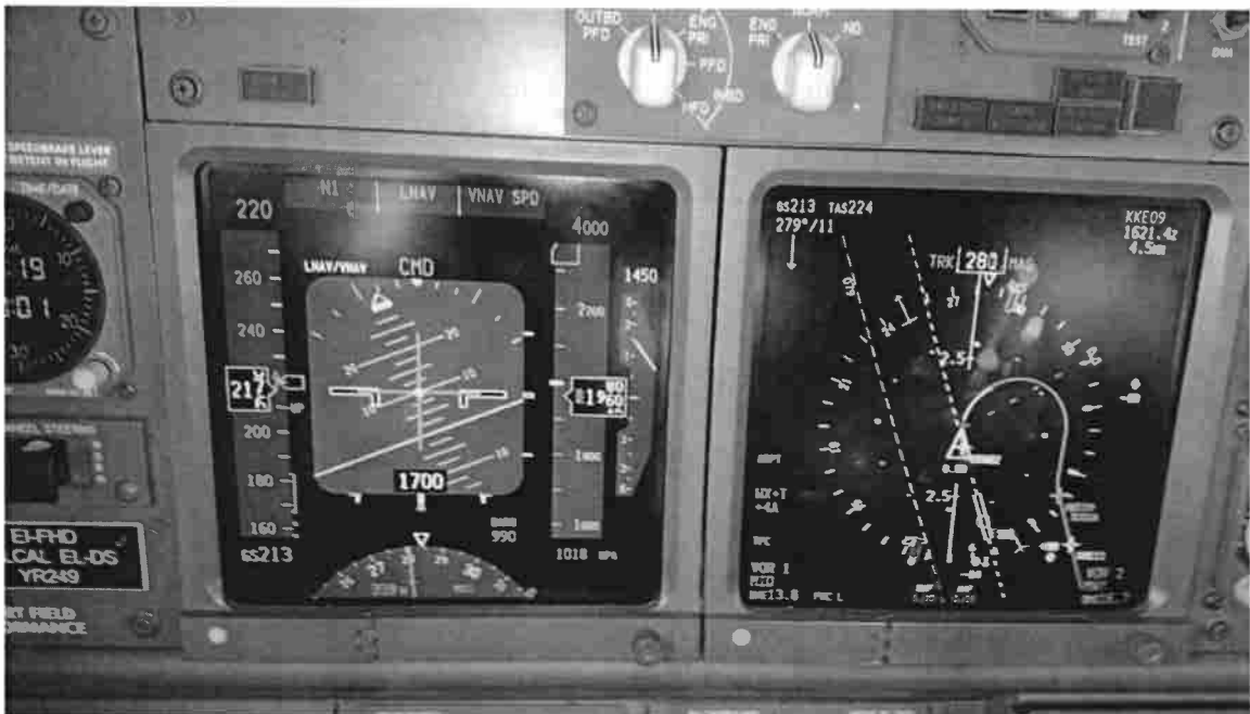
Flap UP and just started the turn. No change regarding the magenta line and the wind is not an issue. Bank angle 21°.
