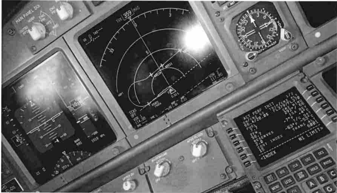
Still on the ground. The T/O mass 66.4 tons and I checked the flap 40 speed 139kts, UP speed 209 kts, could be an option but we did not use it.
