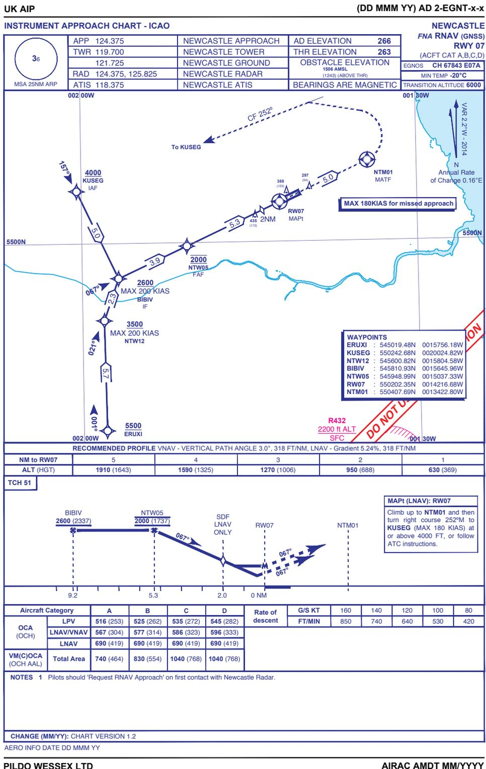
Figure 3 Draft aviation charts for proposed NIA RNAV (GNSS) procedure to runway 07
