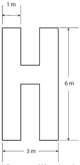
indicates an area which must be used only for the taking off and landing of helicopters.
