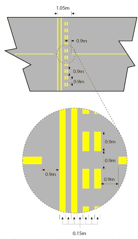
signify the designated visual holding position associated with a runway beyond which no part of a flying machine or vehicle must project in the direction of the runway without permission from the air traffic control unit at the aerodrome during the notified hours of watch of that unit.
