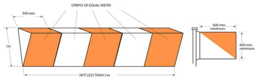
indicate the boundary of an area unfit for the movement of aircraft.
