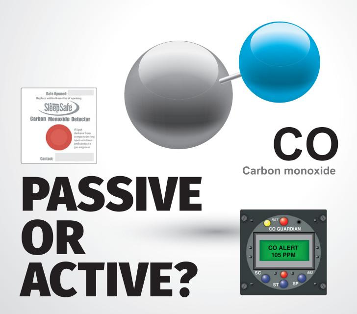
For many years pilots have been using 'passive' carbon monoxide detectors in the cockpit, but 'active' electronic sensors are becoming less expensive and more available
