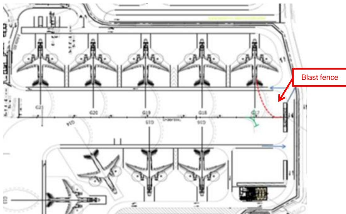
**Figure 1.** Configuration of the Golf Stands showing red, nose gear stop green, and the location of the jetblast fence
