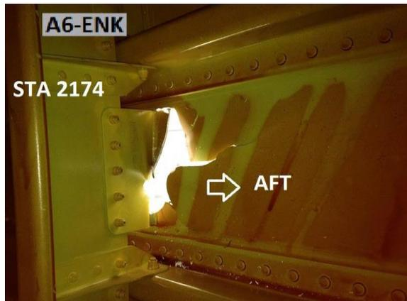
Figure 4. Internal view of fuselage damage
