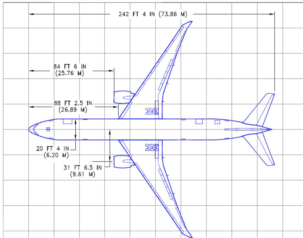
Figure 8. General arrangement – Boeing B777-300
