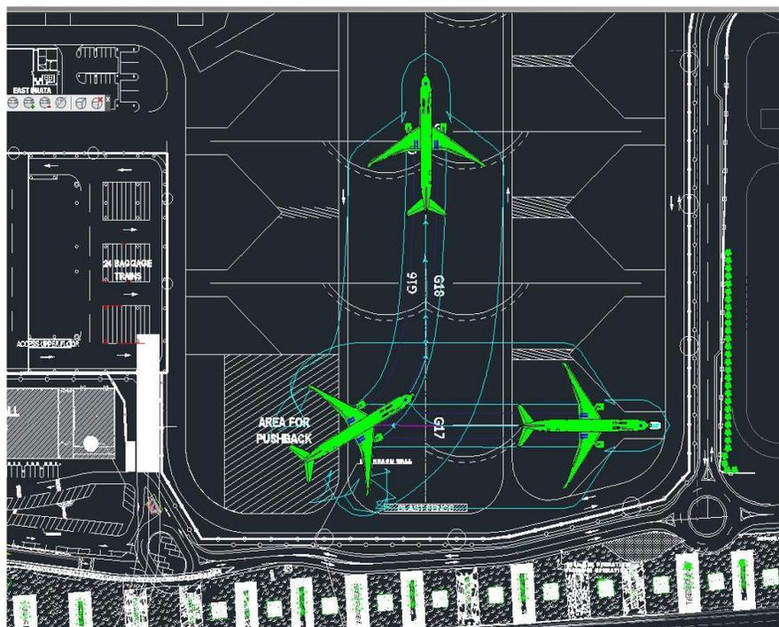
**Figure 11.** Approved pushback sequence off Stand G17 into the hatched area directly behind Stand G17, and then pull forward to the engine start line
