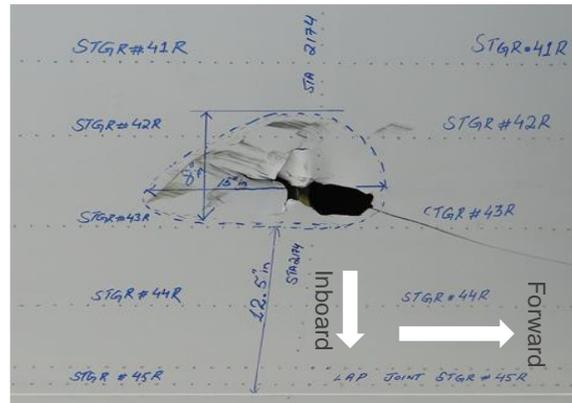
Figure 3. Detail and location of fuselage damage
