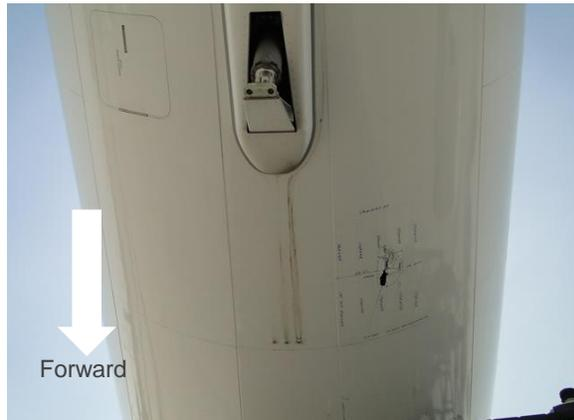
Figure 2. Damage to aft fuselage
