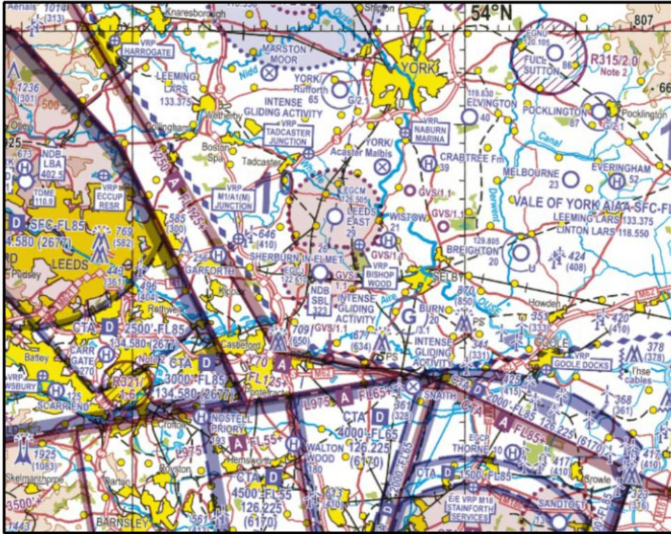
Sherburn has three runway orientations. The most used runway is the hard surface runway that is aligned 28/10 (roughly east/west). It is to both ends of this runway that the IAPs are to be established.
