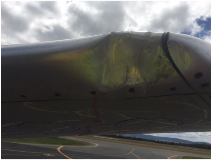
Figure 9: Damage to VUP left horizontal stabiliser
