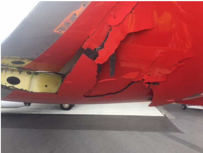
Figure 8: Damage to YFT left winglet
