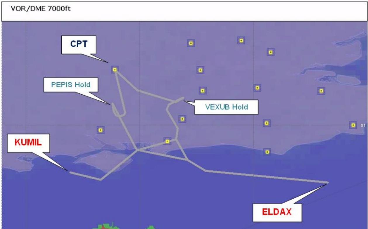
Figure 2: Current VOR/DME Position-Fixing Capability from NATS en-route ground-based Navigational Aids supporting the new Farnborough STARs (7000 ft)
