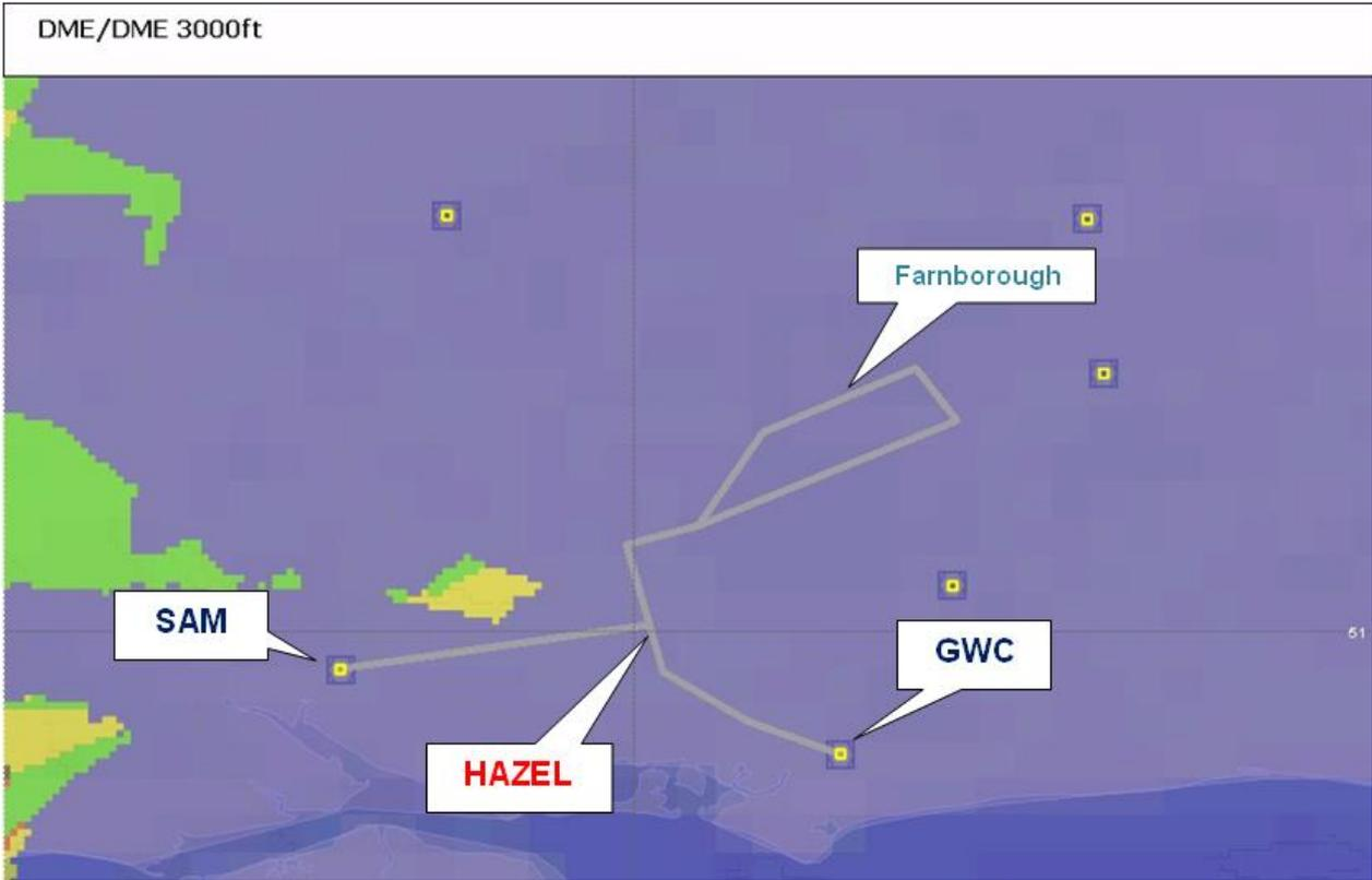
Figure 6: Current DME/DME Position-Fixing Capability from NATS en-route ground-based Navigational Aids supporting the new Farnborough SIDs (3000 ft)
