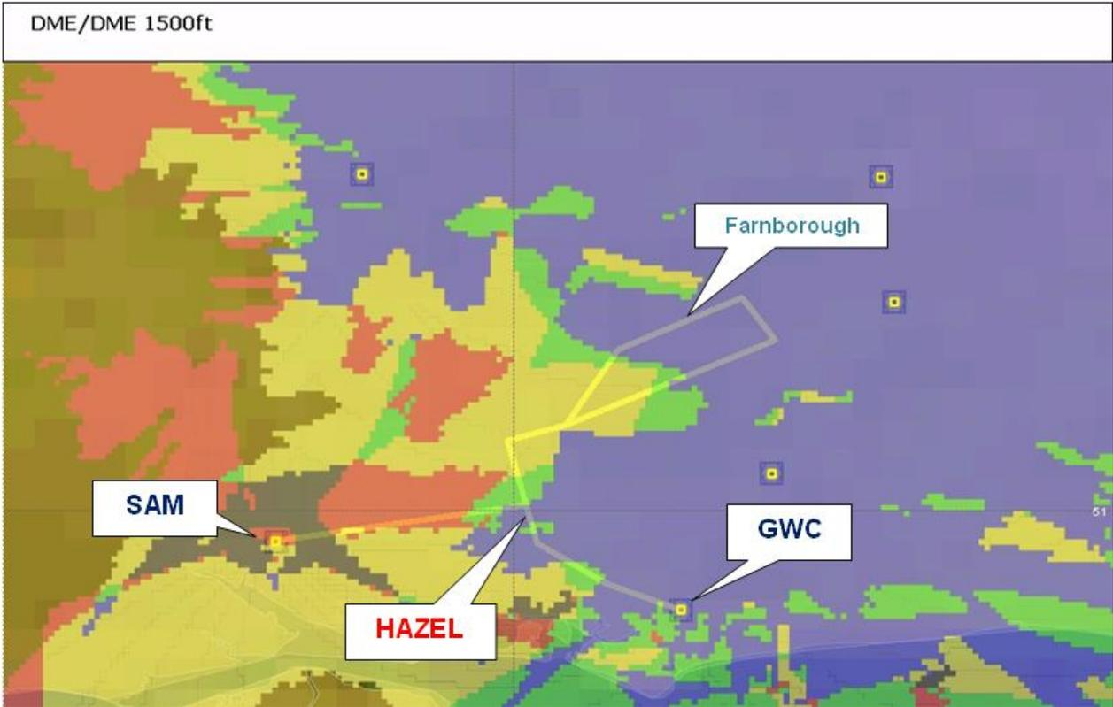
Figure 5: Current DME/DME Position-Fixing Capability from NATS en-route ground-based Navigational Aids supporting the new Farnborough SIDs (1500 ft)
