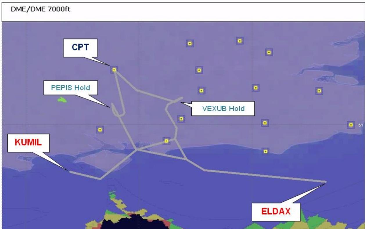
Figure 4: Current DME/DME Position-Fixing Capability from NATS en-route ground-based Navigational Aids supporting the new Farnborough STARs (7000 ft)
