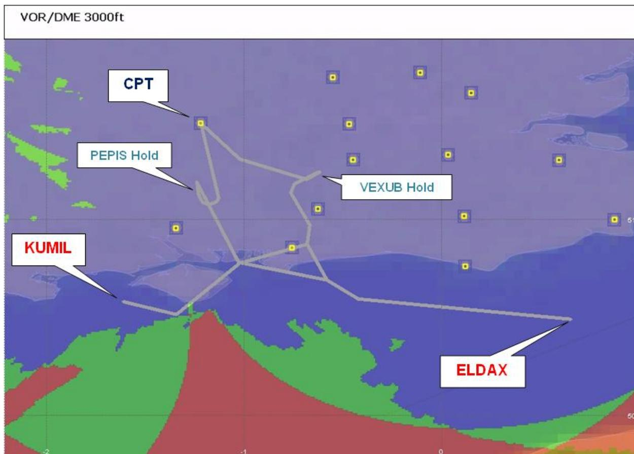
Figure 1: Current VOR/DME Position-Fixing Capability from NATS en-route ground-based Navigational Aids supporting the new Farnborough STARS (3000 ft)
