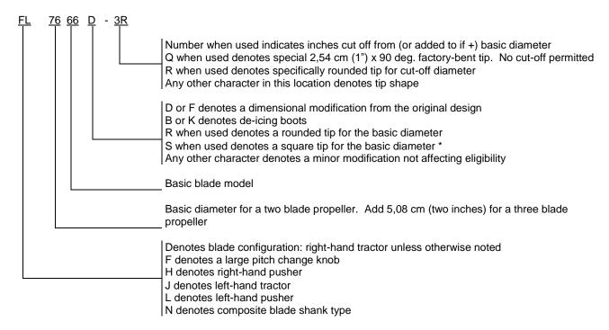
\* Blades may incorporate either round or square tips, yet may not be marked with an "R" or "S" in their model designation. This character is used to distinguish between two or more tip shapes available at the same diameter. Certain blades use "S" o denote shot peening of the exterior surface.
