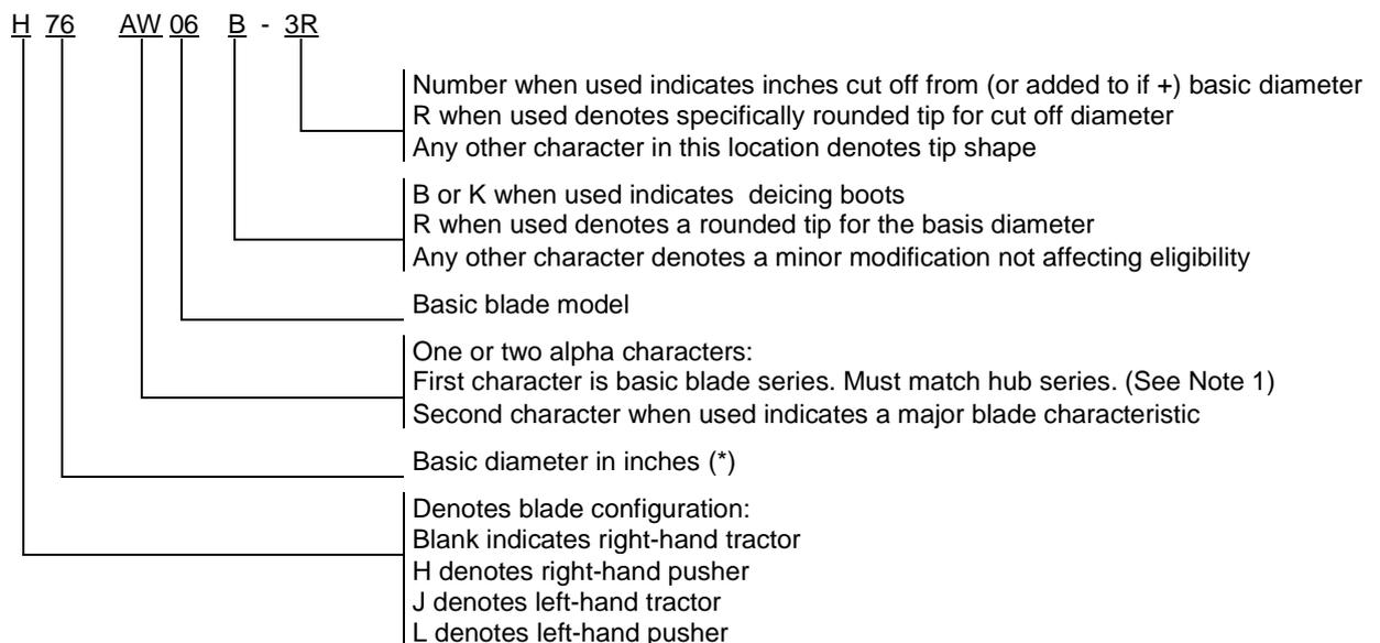
(\*): Diameter limits are nominal diameters of the assembled propeller. They do not include the +/- 0,32 cm (one eighth inch) manufacturing tolerance the FAA allows for propellers with basic diameter less than 426,72 cm (14 feet).
