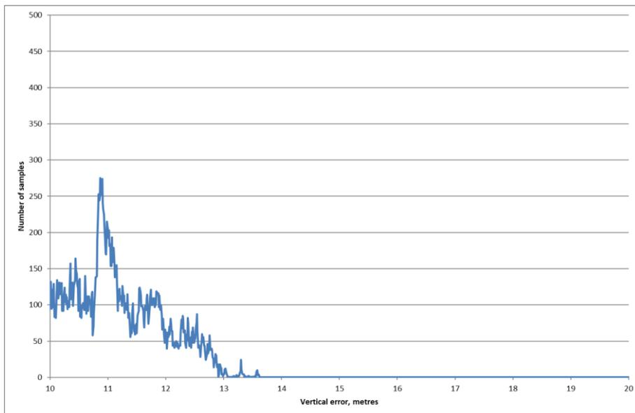
**Figure 3-4: Vertical Error Distribution above 10m for Monitoring Period**
