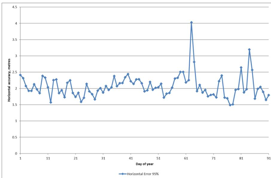
**Figure 3-5: Horizontal Position Accuracy (95%) for Monitoring Period**
