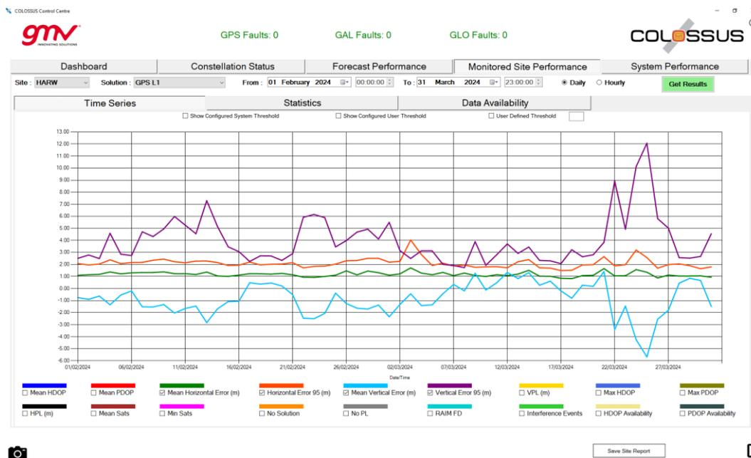
**Figure 5-4: Daily Horizontal and Vertical Error Statistics for GPS L1 during Q1 2024**
