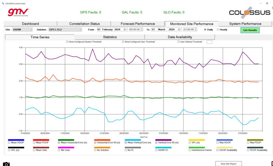
**Figure 5-5: Daily Horizontal and Vertical Error Statistics for GPS L1/L2 during Q1 2024**
