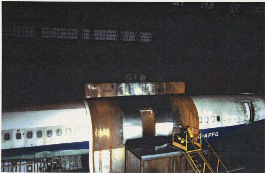
(a) The exterior of the fuselage showing the fire tray and the protected opening, prior to ignition
