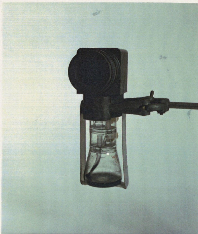
Figure B4 May multi-stage impactor containing trapped smoke particles of less than 2.0\ \mu\text{m} diameter
