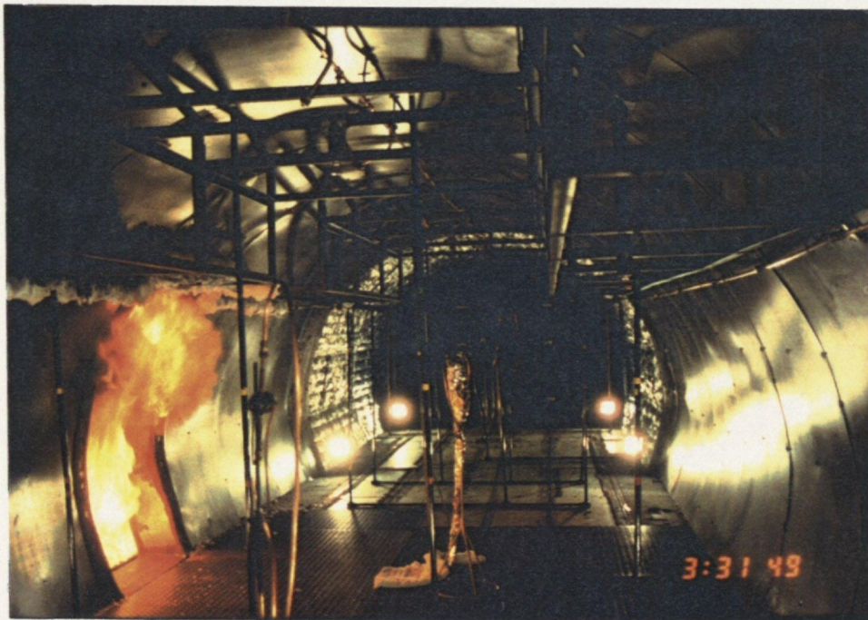
(b) The interior of the fuselage showing the additional fire protection in the vicinity of the fire opening
