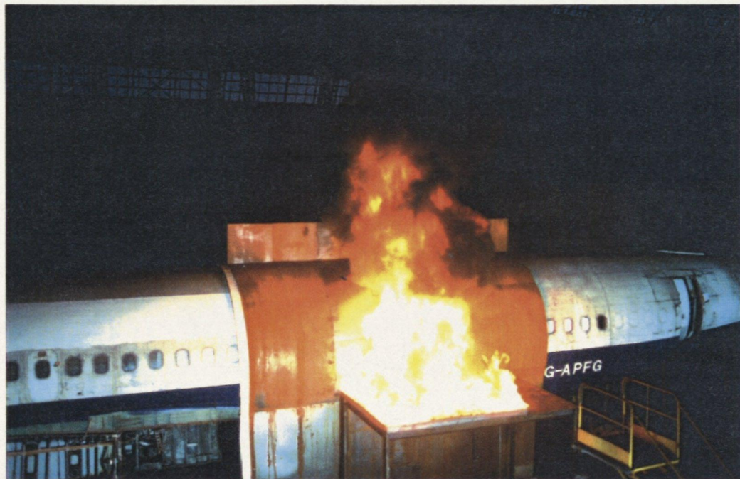
(b) The exterior of the fuselage showing the fuel tray and protected opening, after the fire has become established
