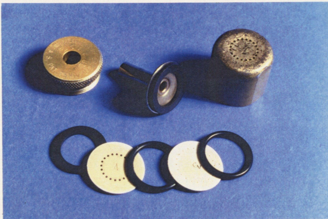
Figure B1 The Andersen mini-sampler - particle size analyser for solid aerosols
