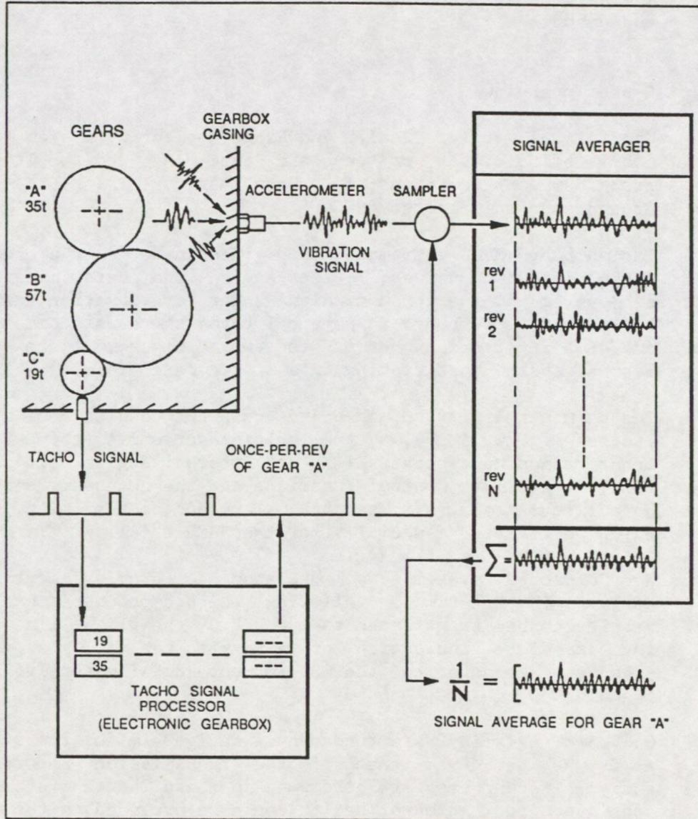
FIGURE 2.2 : Gear signature acquisition
