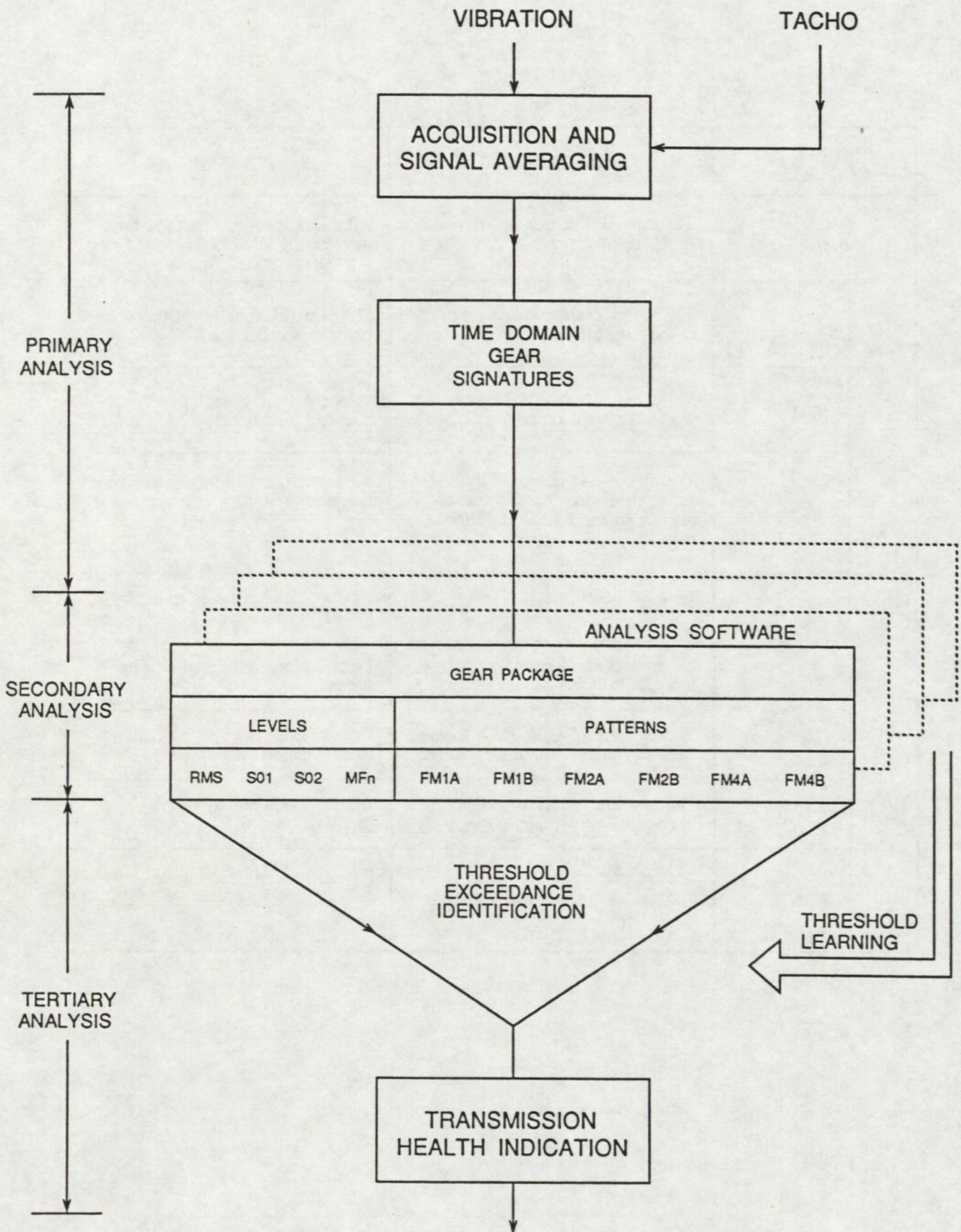
FIGURE 2.1 : HUMS vibration analysis processes
