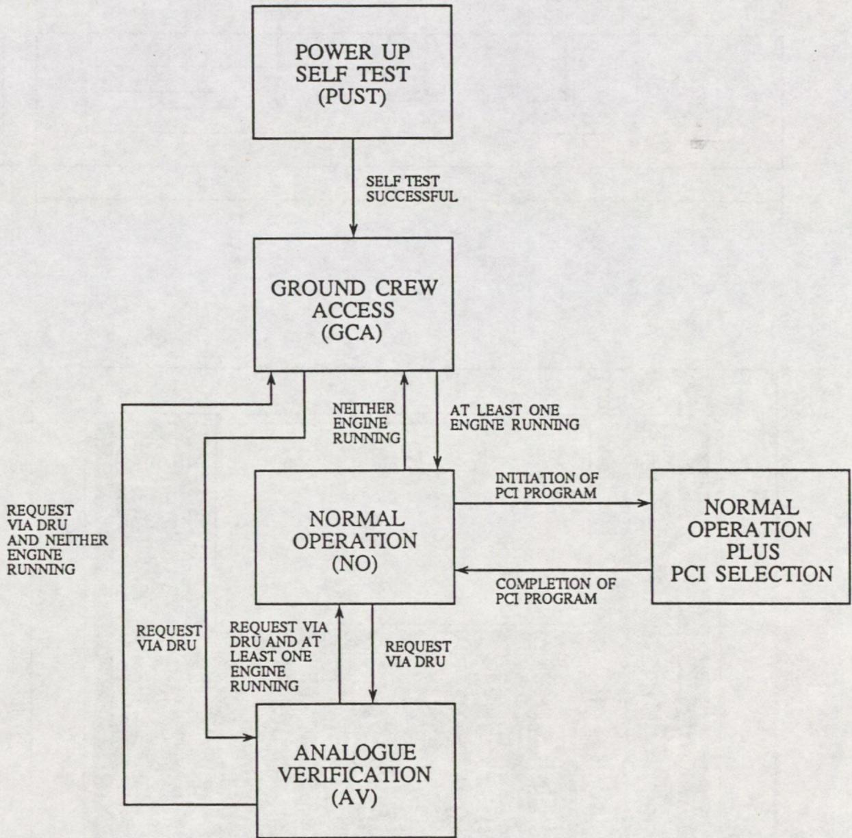
FIGURE 4.1 : Operating mode transition diagram
