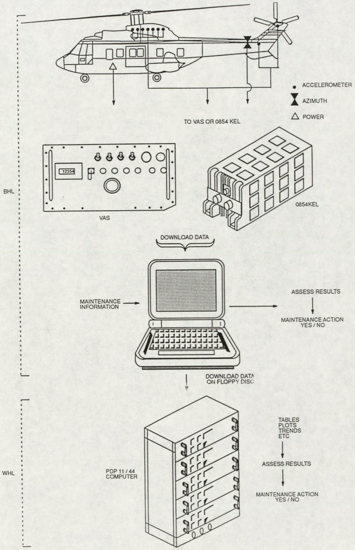
Figure 8 – BHL Super Puma – System Components
