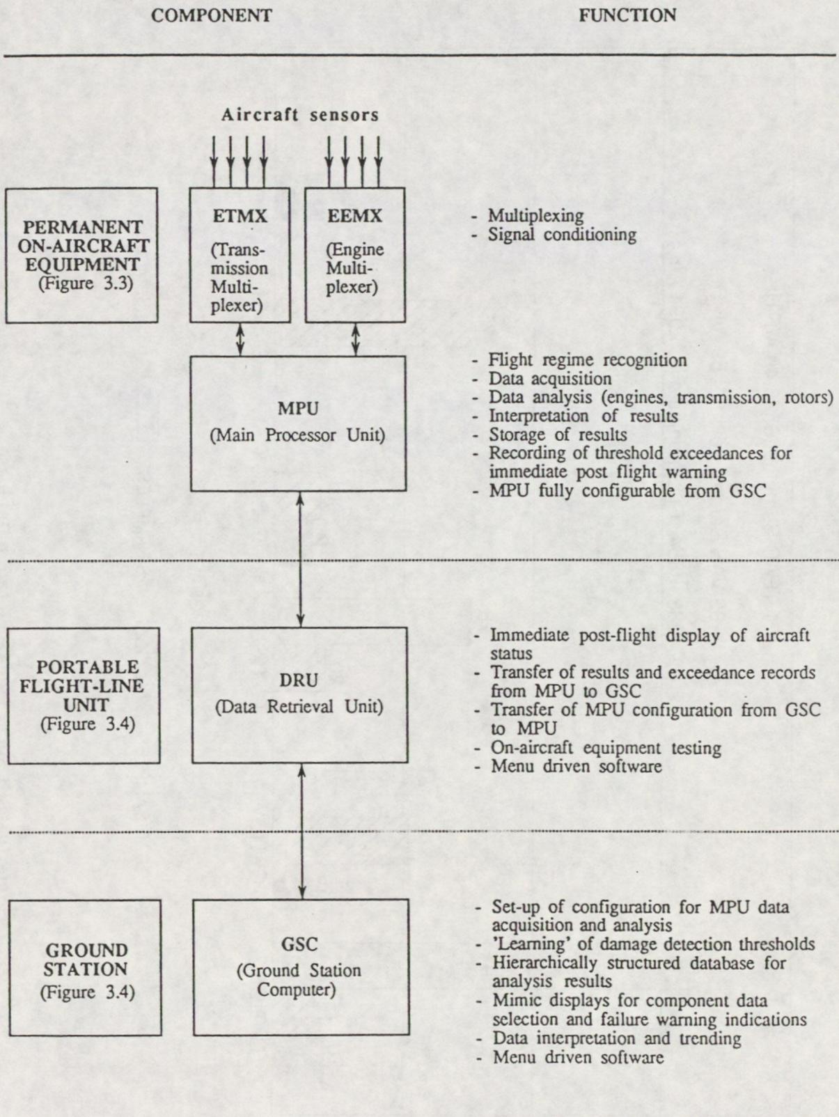
Figure 9 – BIHL S61N – System Components and Functions
