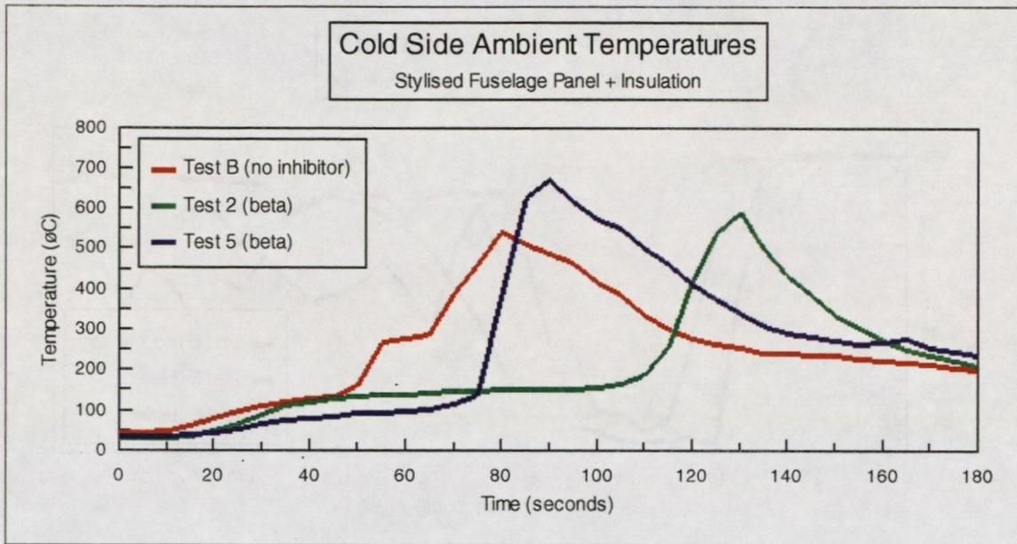
Figure 5 Test Data Set B Stylised Fuselage + Insulation Results
