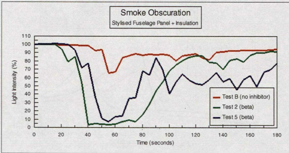
Figure 7 Test Data Set B Stylised Fuselage + Insulation Results
