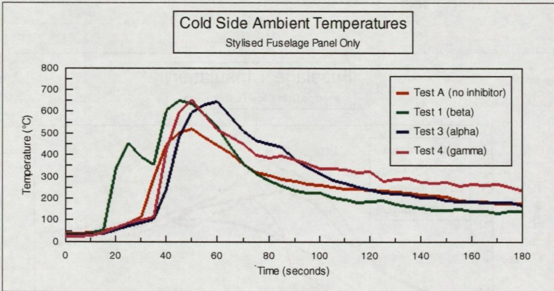
Figure 4 Test Data Set B Stylised Fuselage Panel Results
