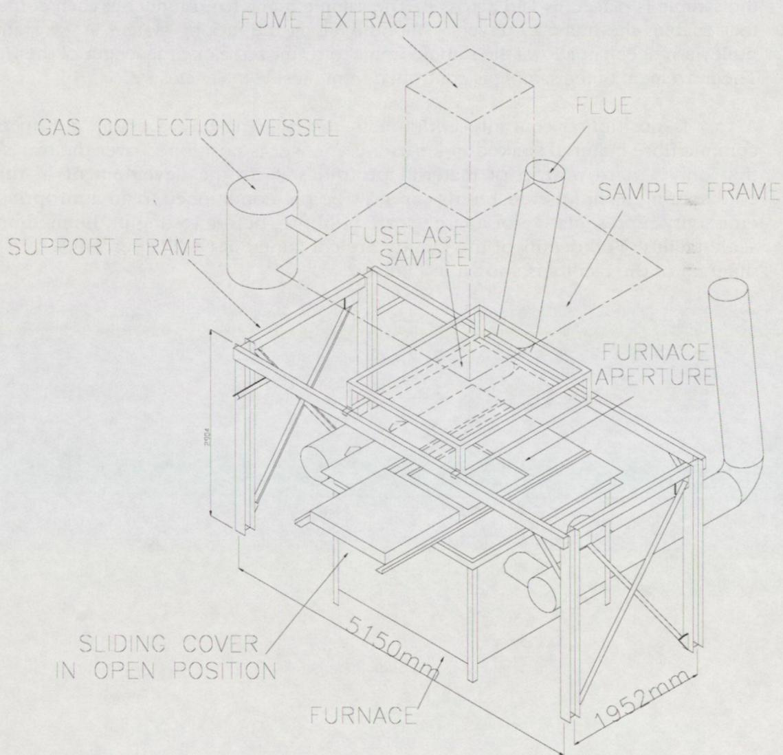
**Figure 1 Medium Scale Burnthrough Facility**
