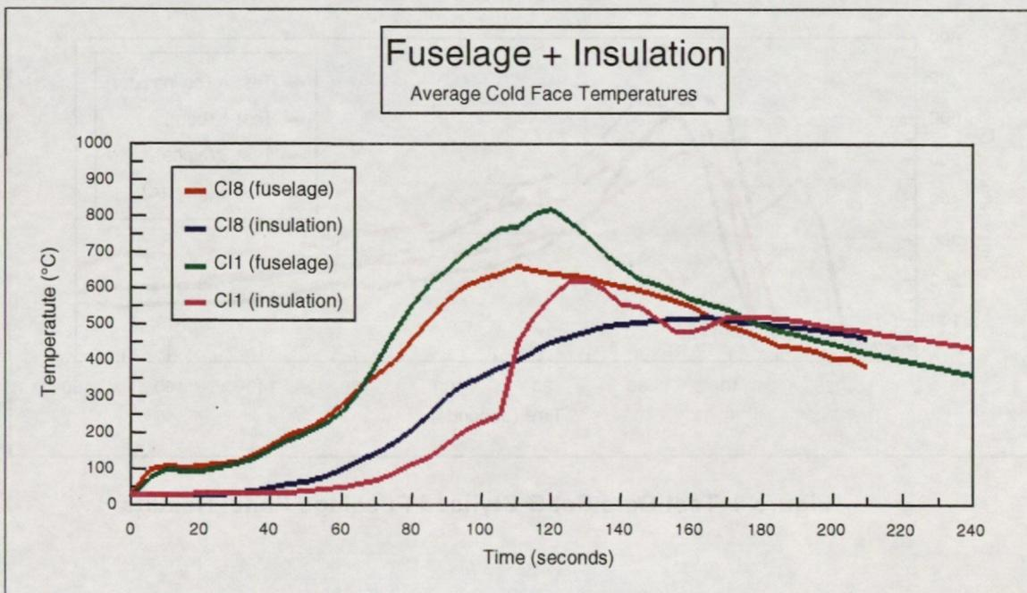
Figure 2 Test Data Set A Fuselage Panel + Insulation Results
