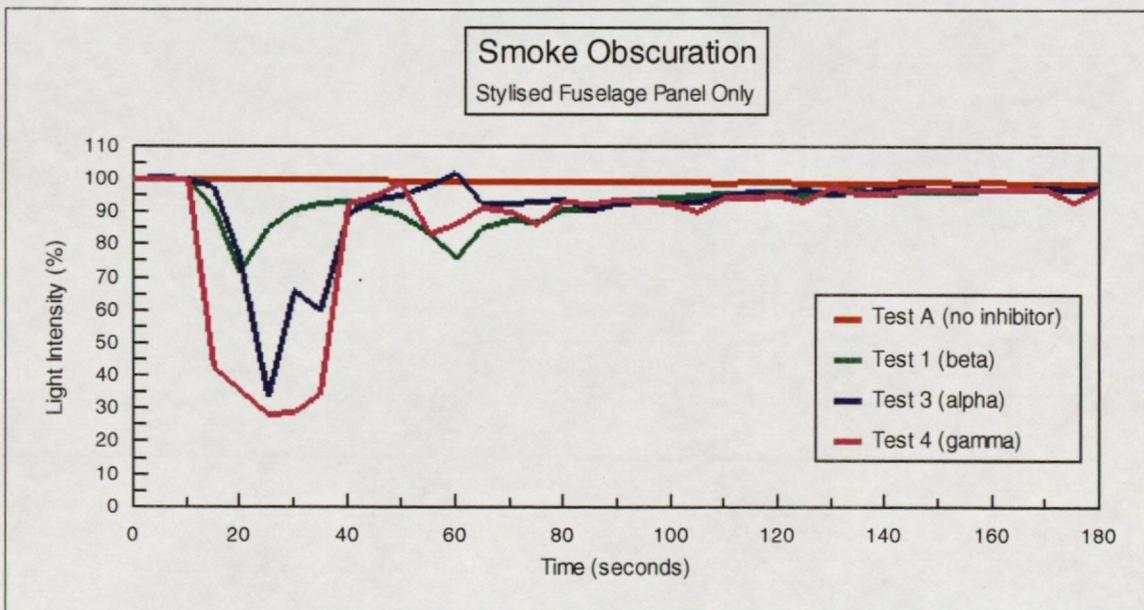
Figure 6 Test Data Set B Stylised Fuselage Results
