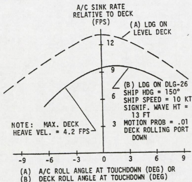
**Figure 10 Predicted safe sink rates for an SH-2F helicopter**
