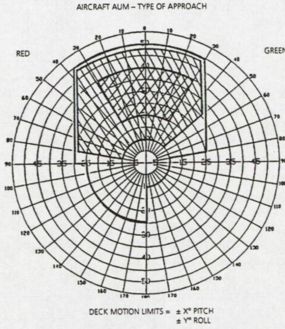
**Figure 12 Typical ship/helicopter operation limits**
