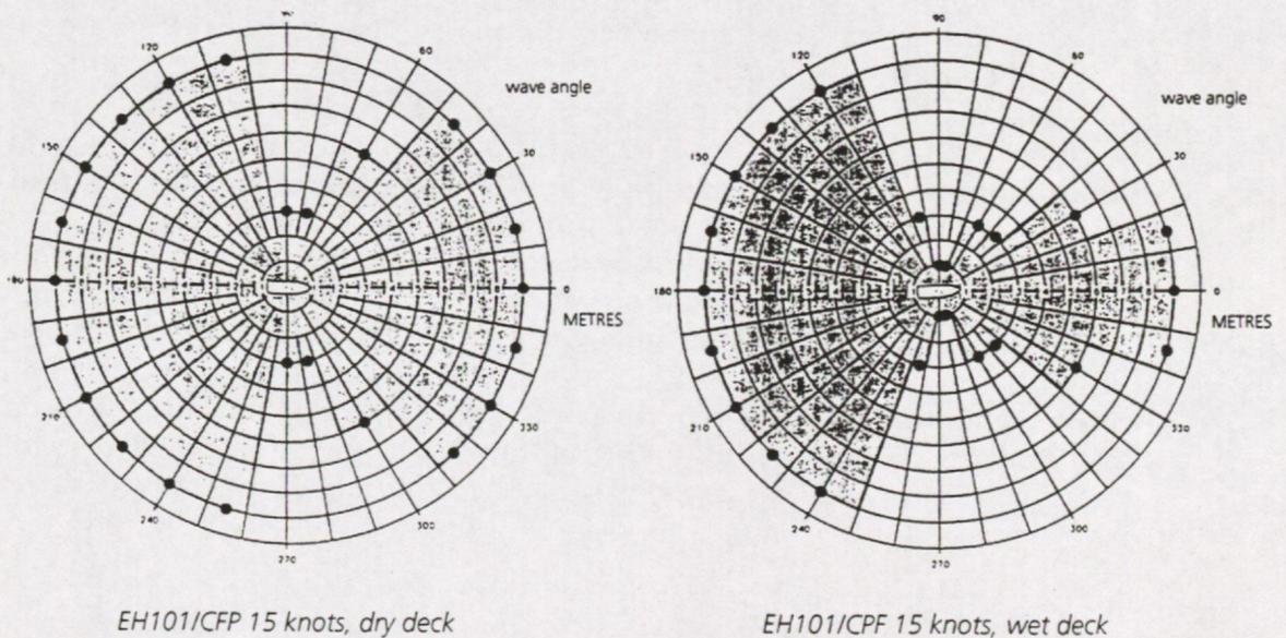
**Figure 11 Deck safety envelopes, as a function of wave height and direction, for an EH101 helicopter and CPF class frigate**
