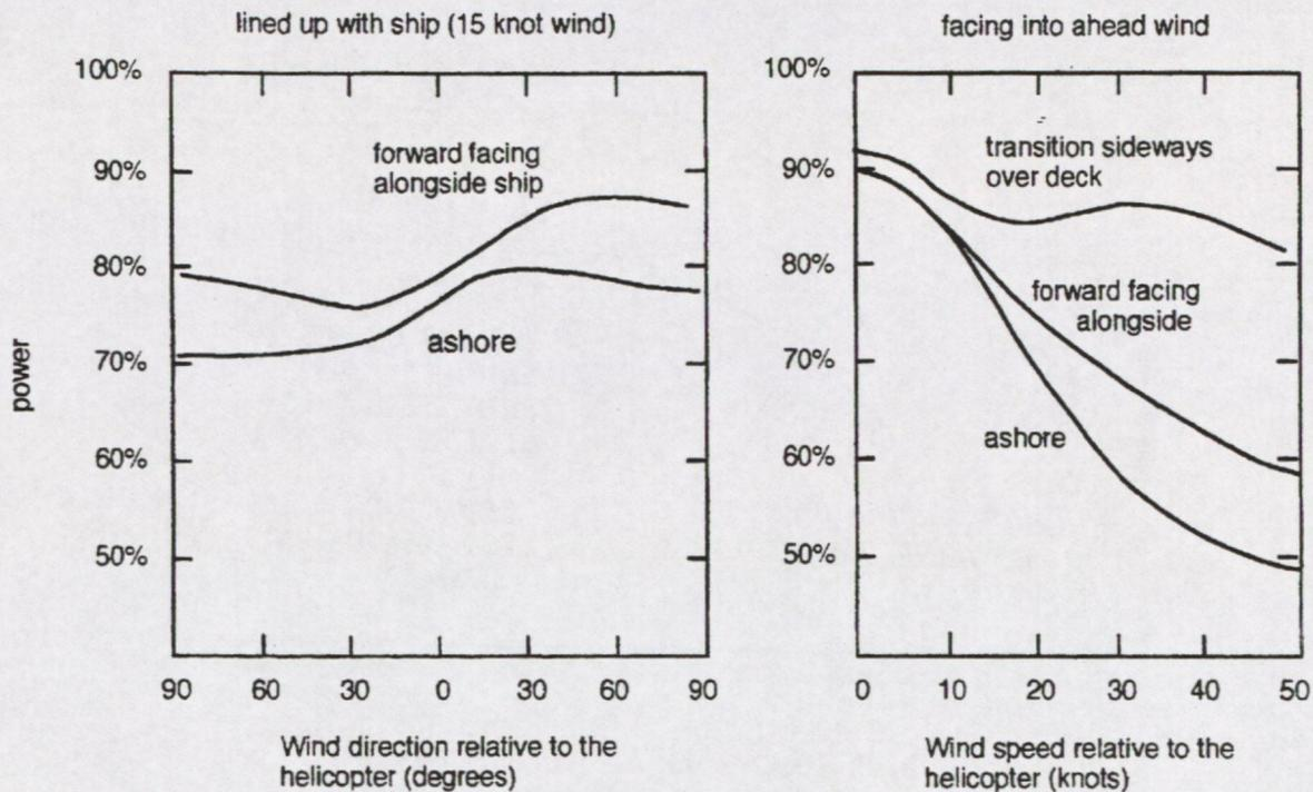
**Figure 9 The effect of turbulence around a deck on the power required for hovering**
