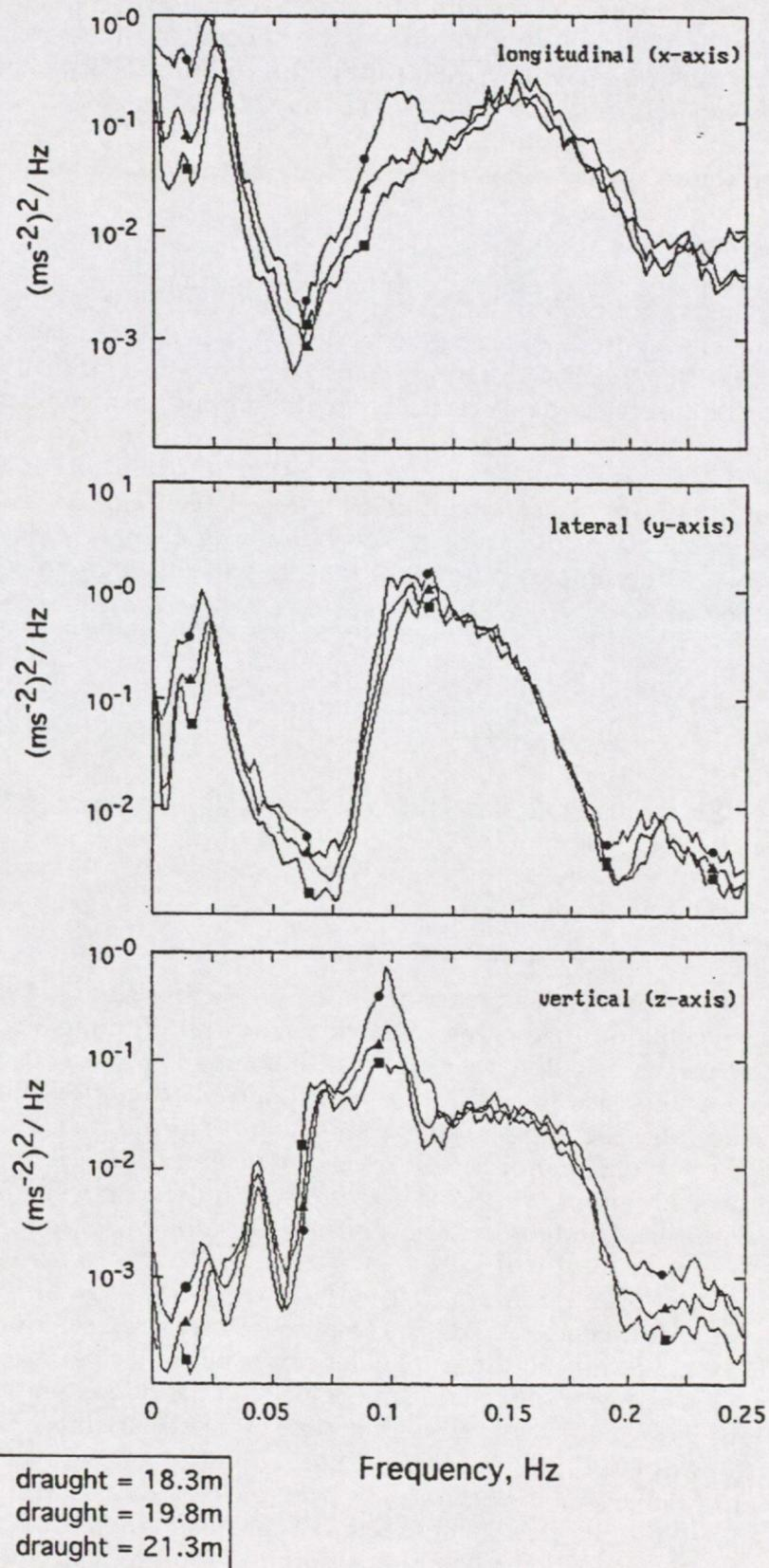
Figure 4 A comparison of power spectral densities of accelerations in the three translational axes of a semi-submersible drilling rig at three draughts After Lewis and Griffin (1990)
