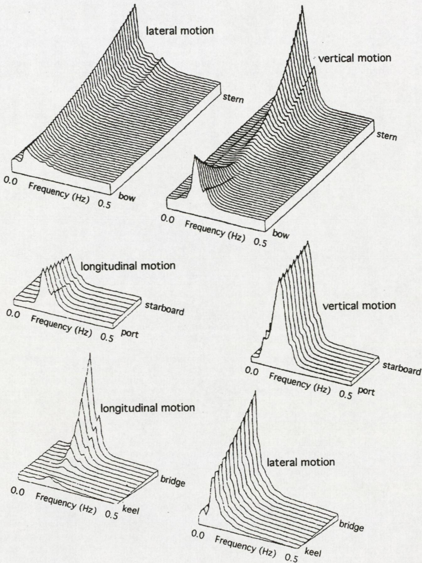
Figure 2 The variation in power spectral densities of translational accelerations with position in a ship
