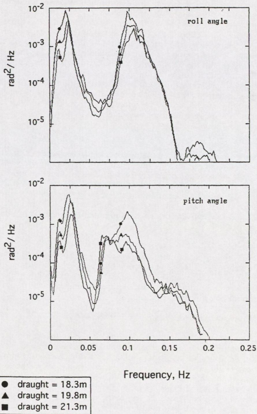
**Figure 5** A comparison of power spectral densities of roll and pitch displacements of a semi-submersible drilling rig at three draughts
