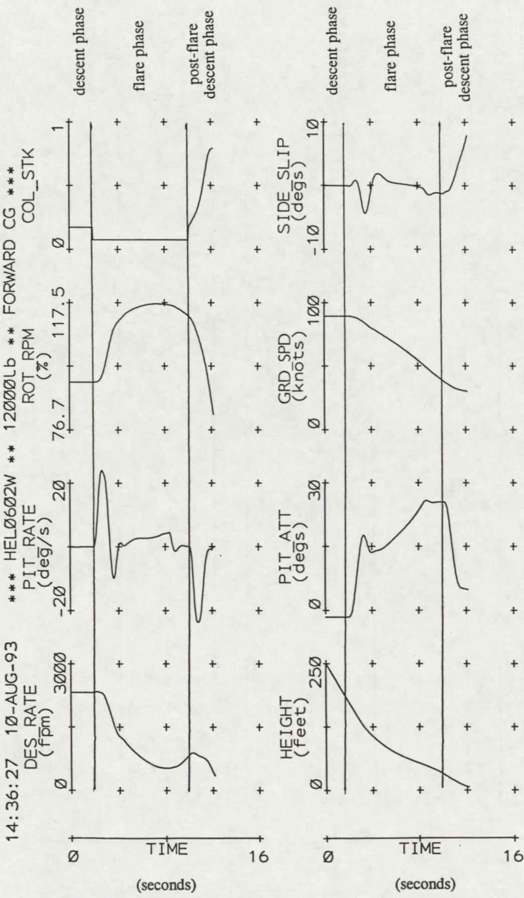
Figure 14 HEL0602W Autorotative Landing following a Maximum Duration Descent Profile (90 knots)
