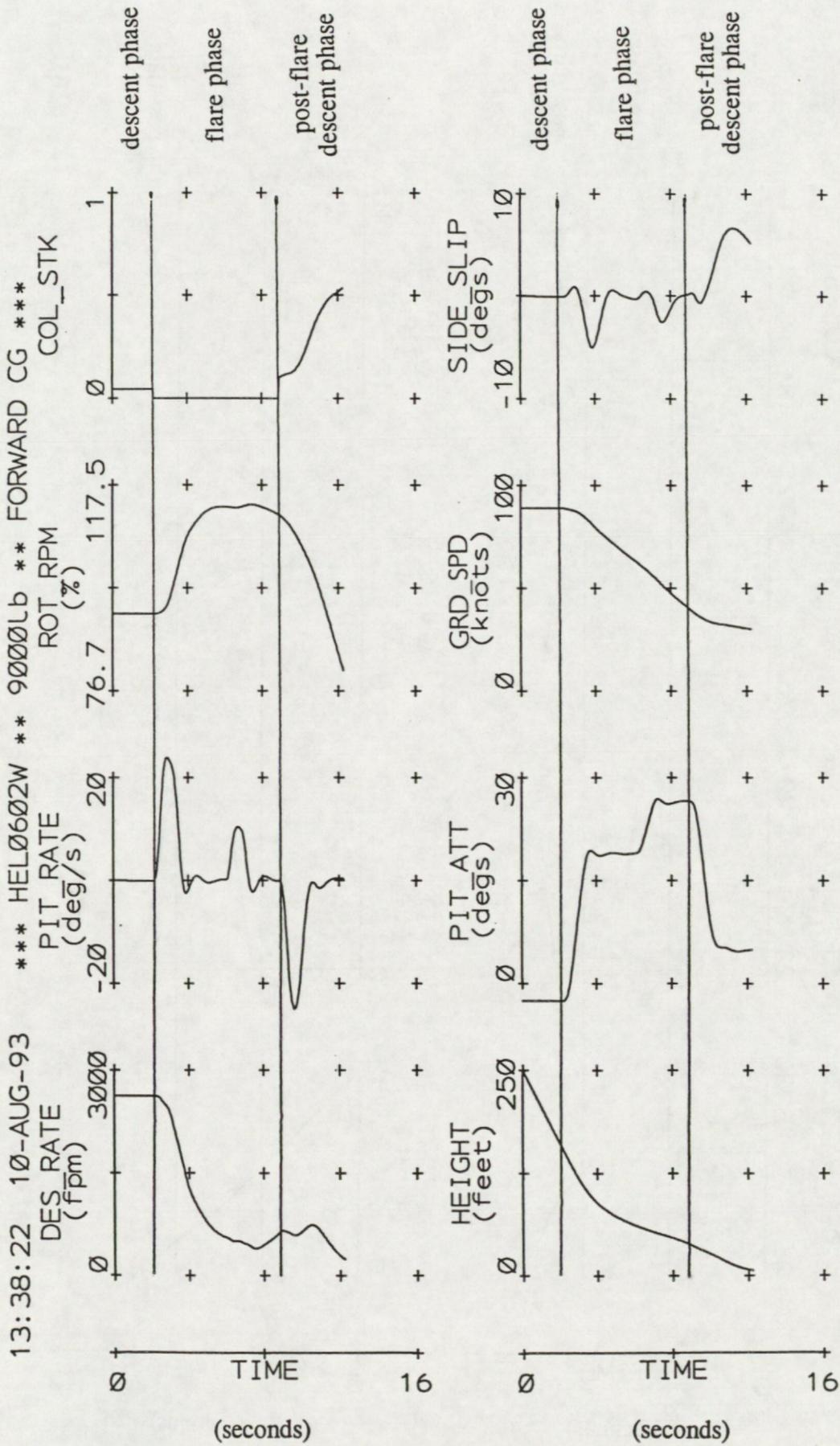
Figure 10 HEL0602W Autorotative Landing following a Maximum Duration Descent Profile (90 knots)
